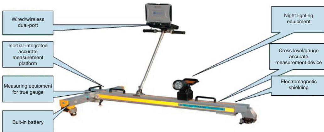
FIGURE 14.11 #0 track inspection device in China.
