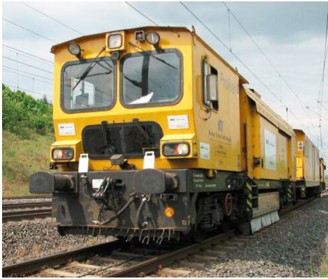
FIGURE 14.25 Turnout grinding train.
