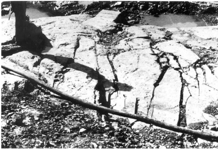
Figure 2.9. Upper surface of Unit E sandstone at Mangrove Creek Dam valley bulge, showing joints open as much as 100 mm, clay-filled in part.
