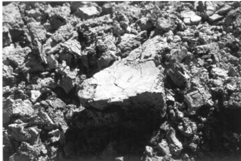
(b) View of pieces of the fissured soil. The large piece is about 300 mm across
