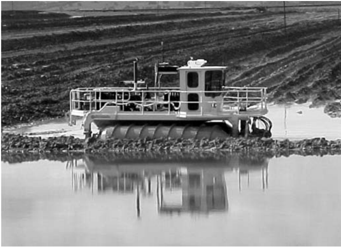
Figure 19.15. Rotating screw device for breaking up the salt layer on top of alumina red mud tailings. (Photograph courtesy of Geographe Earthmoving).
