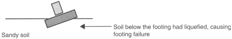
Figure 27.5 Foundation failure due to liquefaction
