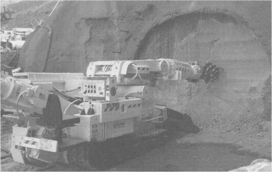
Figure 26.4 Roadheader in action. (Source: http://www.antraquip.net )
