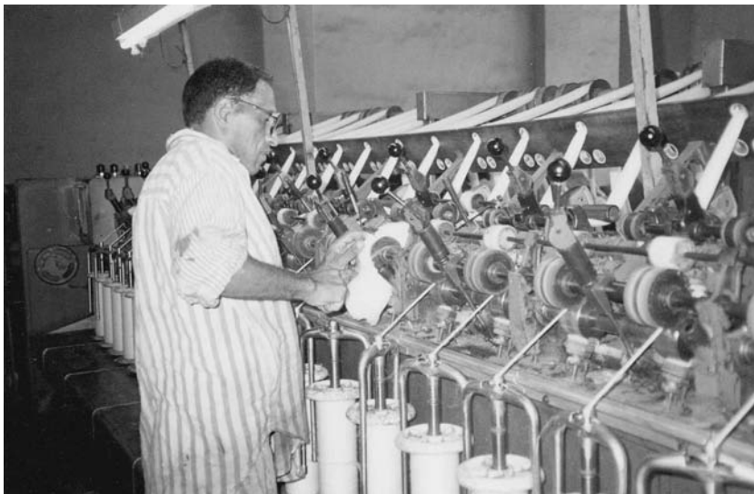
Illustration 3.1. Fathy repairing a tangle on the front of the winding machine.
