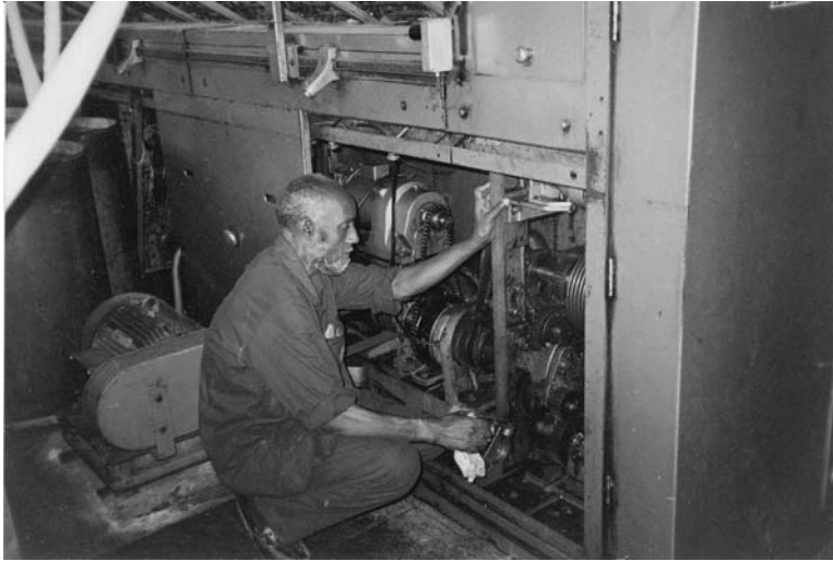
Illustration 3.4. Sheikh Darwish, a mechanic, making an adjustment to the winding machine.
