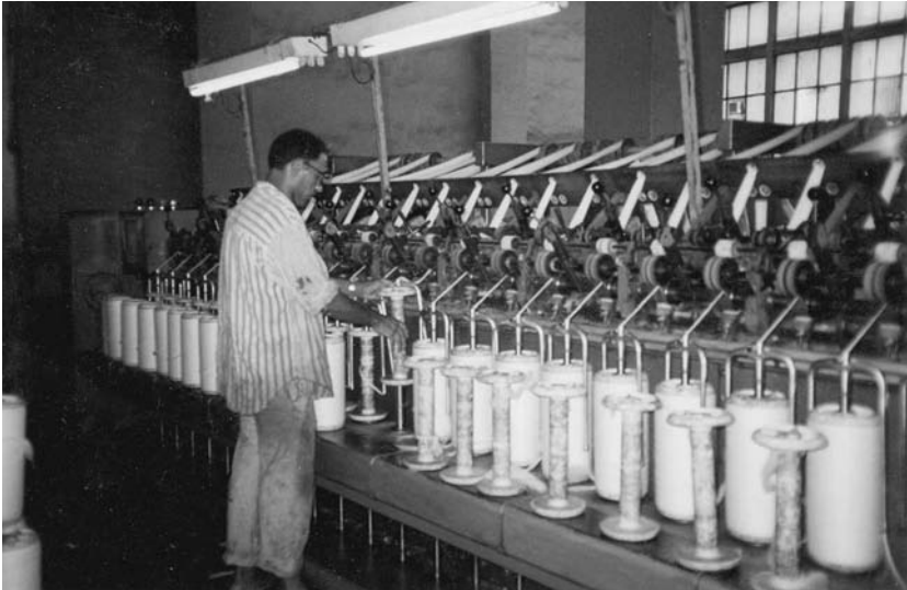
Illustration 3.3. Fathy replacing the spindles on the winding machine.
