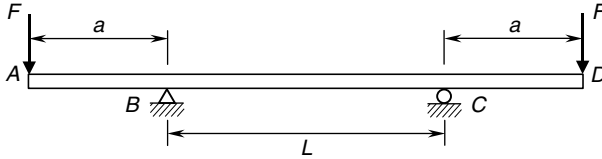
FIGURE 2.67 Twin concentrated forces.
