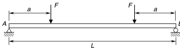
FIGURE 2.44 Twin concentrated forces.
