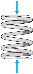
FIGURE 12.5 Helical compression spring of unequal pitch.
