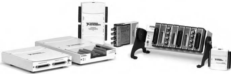
FIGURE 29.1 Examples of typical, computer-based data acquisition devices. Plug-in devices are also commonly available for USB, PCI, and PCI Express buses.
