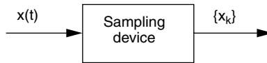
FIGURE 3.16 A continuous-time signal x(t) and a sampling device that produces a sample sequence \{x_k\} .
