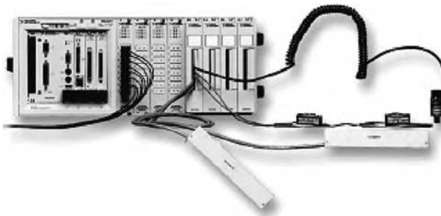
FIGURE 35.10 Rack-mount industrial PC-based data-logging system.
