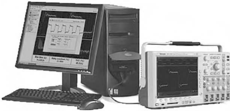
FIGURE 33.4 Virtual instrumentation implementation using a traditional instrument as the measurement hardware.
