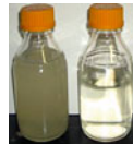
Fig. 8.5 Photograph of domestic septic tank effluent ( left ) and single pass sand filter effluent ( right )
