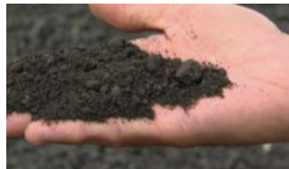
Fig. 15.2 Class A biosolids produced from wastewater treatment plant sludge in Chicago, Illinois (source: Chicago Tonight, 11 Aug 2014)
