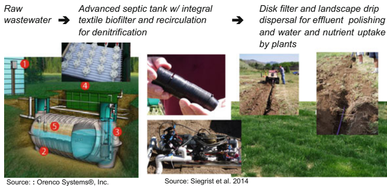
Fig. 1.16 Example of a system and illustration of key components for use where soil and site conditions are suitable for soil-based treatment and water reuse and nutrient recovery is desired
