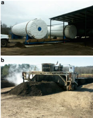
Fig. 15.3 Photographs of septage composting using (a) in-vessel or (b) windrow composting. (Photographs courtesy of Robert Rubin)
