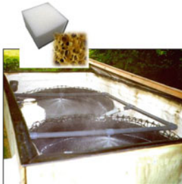
b. Foam cubes are containerized in a cylindrical unit with a distribution and underdrain system built in. Effluent is intermittently dosed onto the filter surface.
