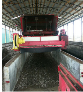
Fig. 15.4 Photograph of aerated bin composting of septage along with fats, oils and greases. (Photograph courtesy of Robert Rubin)
