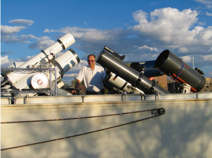
Fig. 5.6 Four hundred years later, amateur telescopes can produce professional results. In this photograph, the author stands next to some of his telescopes, left-right: Obadiah, a 16-in. Schmidt camera with a 7-in. apochromatic refractor on top; Pegasus, the 8-in. reflector he has used since 1964; Samwise, a 10-in. telescope; and Clyde, a Celestron 14-in. telescope. Photograph by Wendee Wallach-Levy
