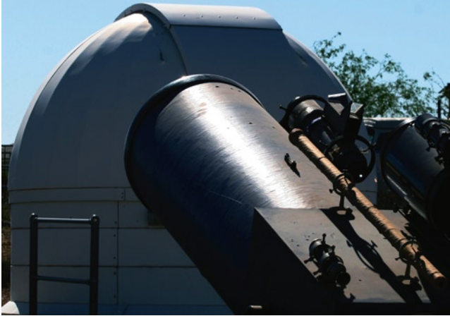
Fig. 5.5 This replica of Galileo’s telescope rests atop the author’s 16-in. diameter reflector, with which he has discovered eight comets. The telescope is pointing towards a 6-ft diameter dome which houses another telescope. Photograph by David H. Levy
