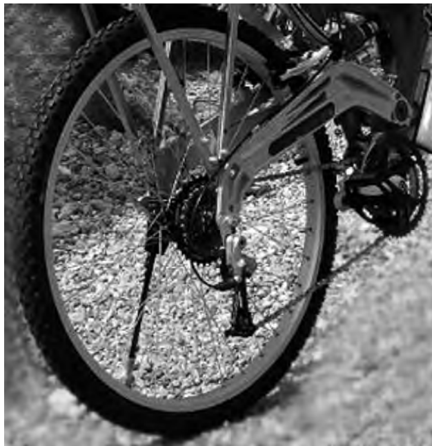
FIGURE 4.25 Bicycle chain drive.
