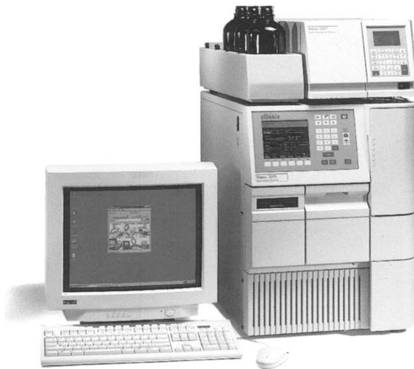
Figure 9 A versatile integrated solvent and sample management module configured with modular refractive index detector for performing basic GPC.
