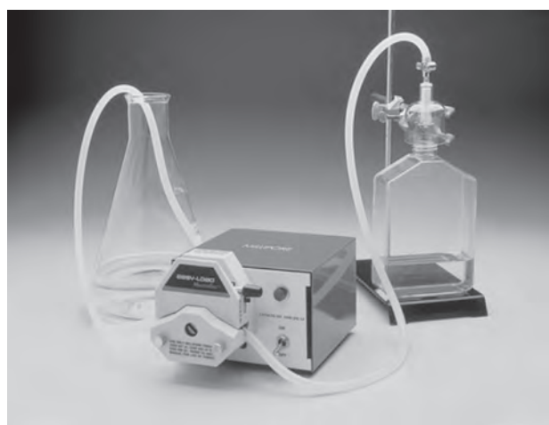
Fig. 10.12. Peristaltic Pump Filtration. Sterile filtration with peristaltic pump between nonsterile reservoir and sterilizing filter (Courtesy of Millipore, Ltd., UK. This setup is no longer supplied by Millipore, who have introduced the Millipore Mobius FlexReady, designed for use on a larger scale, but a different peristaltic pump could be used.)
