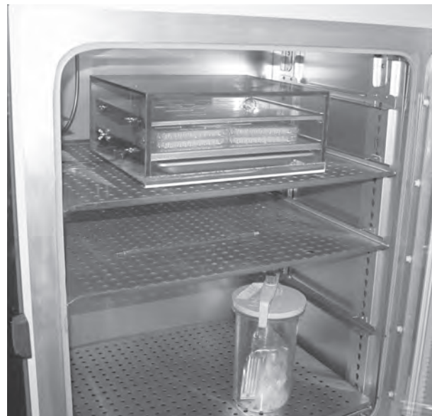
Fig. 4.11. Culture Chambers. Inexpensive alternatives to CO 2 incubator. Upper shelf, custom-made clear plastic box (Courtesy of Reeve Irvine Institute); lower shelf, anaerobic jar (BD Biosciences.)
