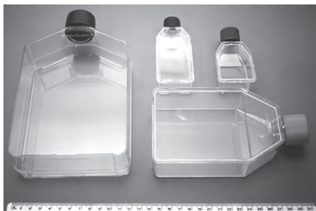
Fig. 7.5. Plastic Flasks. Sizes illustrated are 10 and 25 cm 2 (Falcon, BD Biosciences), 75 cm 2 (Corning), and 185 cm 2 (Nalge Nunc) (see Table 7.2 for representative sizes and capacities).
