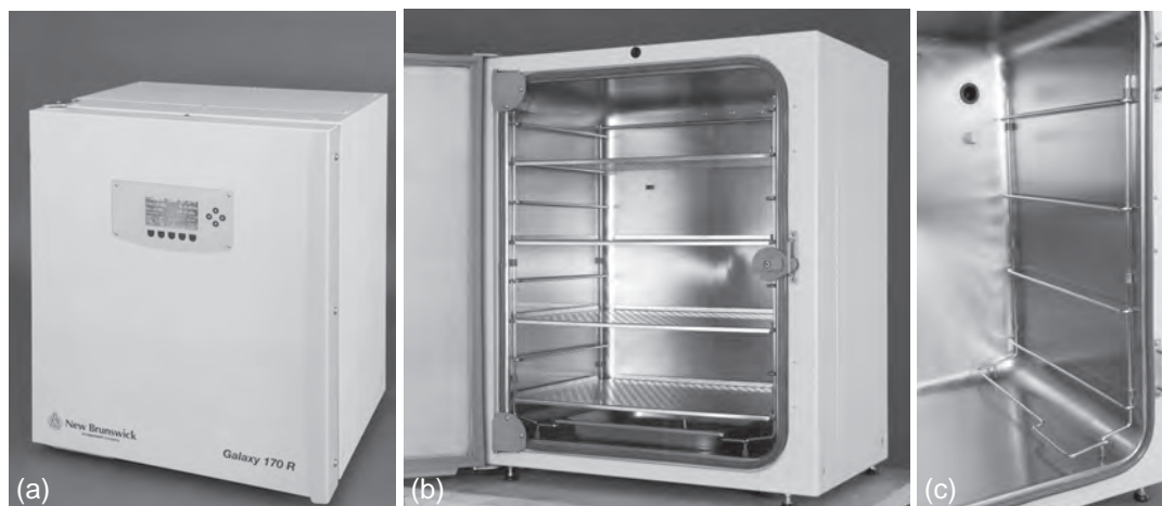
Fig. 4.12. CO 2 Incubator. Galaxy 170R fanless CO 2 incubator. (a) Exterior with LCD display panel. (b) Interior showing shelving and water tray in place; and (c) showing smooth easily cleaned interior with removable racking that does not penetrate the stainless steel lining. (See also Fig. 4.13.) (Courtesy of New Brunswick Scientific–RS Biotech.)
