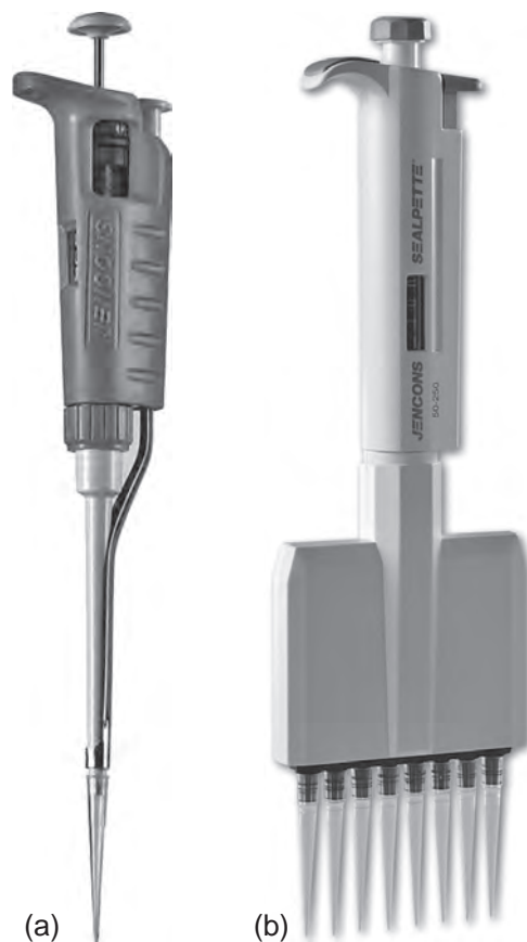
Fig. 4.3. Pipettors. (a) Variable-volume pipetting device. Also available in fixed volume. The pipettor is not itself sterilized but is used with sterilized plastic tips. (b) Multipoint pipettor with manifold to take 8 plastic tips; also available for 4 and 12. (Courtesy of VWR-Jencons.)
