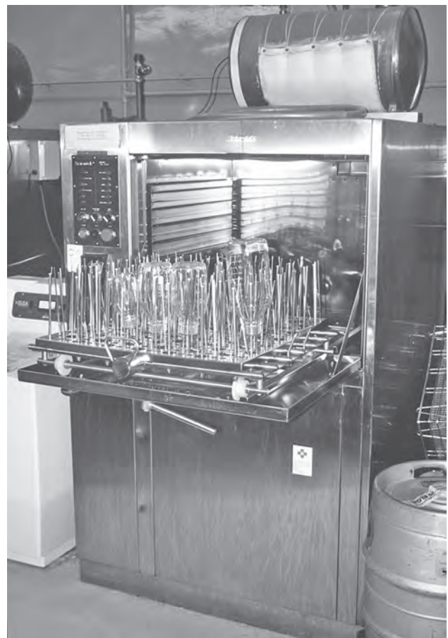
Fig. 4.14. Glassware Washing Machine. Glassware is placed on individual jets, which ensures thorough washing and rinsing (Betterbuilt). (Courtesy of Beatson Institute.)
