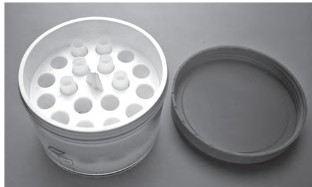
Fig. 19.4. Nunc Cooler. Plastic holder with fluid-filled base. The specific heat of the coolant in the base insulates the container and gives a cooling rate of about 1^{\circ}\text{C}/\text{min} in the ampoules.
