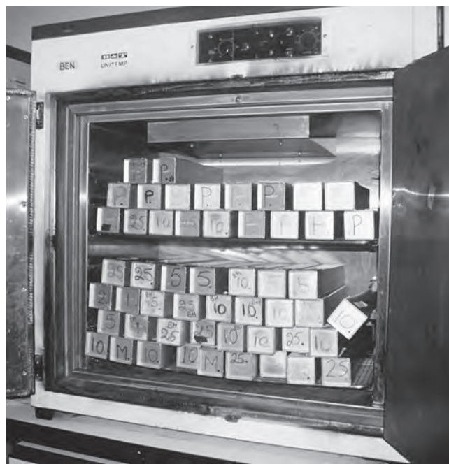
Fig. 10.7. Sterilizing Oven. Pipette cans are stacked with spaces between to allow circulation of hot air. Brown staining on front of oven shows evidence of volatile material from sterile-indicating tape, a problem when using tape in a hot oven.
