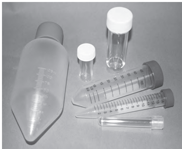
Fig. 4.18. Tubes. Centrifuge and samples tubes, available sterile but non-tissue-culture grade, although tissue culture grade tubes are available (BD Biosciences; Corning). Clockwise from the left: 250-mL centrifuge tube (Corning), 5-mL Bijou bottle (Sterilin), 30-mL universal container (Sterilin), 50-mL centrifuge tube (BD Biosciences), 15-mL centrifuge tube (BD Biosciences), and 5-mL sample tube (BD Biosciences).
