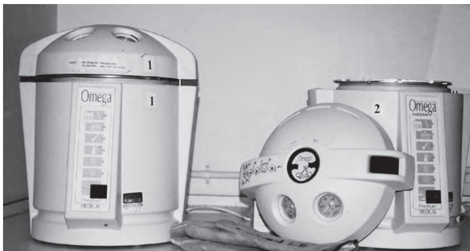
Fig. 4.16. Bench-Top Autoclave. Simple, top-loading autoclave from Prestige Medical; left with lid closed, right with lid removed for filling. (Courtesy of Beatson Institute.)
