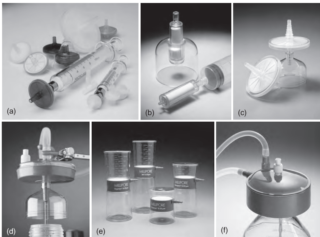
Fig. 10.11. Disposable Sterilizing Filters. (a) Millex 25-mm disk syringe filter. (b) Sterivex high capacity; Luer fitting but can be attached via hose. (c) Millex 50-mm, in-line filter, with and without bell. (d) Steripak large in-line filter with bell (lowered in use to cover neck of bottle). (e) Stericup with storage vessels; also available as Stericap bottle-top filter. (f) Bottle-top filter drawing from separate reservoir (see Fig. 10.10 with built-in reservoir). (a–d) Positive pressure. (e, f) Negative pressure. (Photographs courtesy of Millipore Ltd., UK.)
