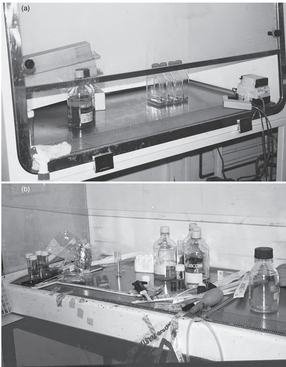
Fig. 5.4. Layout of Work Area. (a) Laminar-flow hood laid out correctly with pipettes on the left at the back, propped up for easy access and to allow airflow to the rear grill, medium to the left of the work area, culture flasks central and well back from the front edge, and pipette controller on the right. Positions may be reversed for left-handed workers. (b) Laminar-flow hood being used incorrectly. The hood is too full, and many items encroach on the air intake at the front, destroying the laminar airflow and compromising both containment and sterility.
