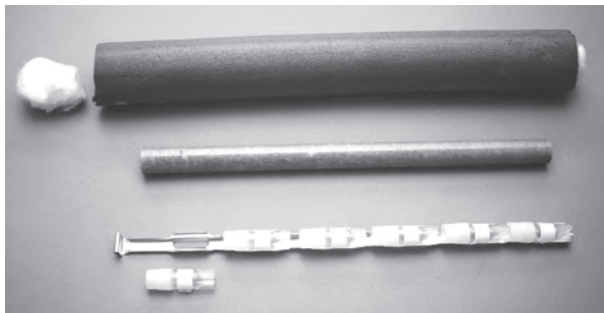
Fig. 19.2. Ampoules on Cane with Insulation for Slow Cooling. Plastic ampoules are clipped onto an aluminum cane (bottom), enclosed in a cardboard tube (middle), and placed inside an insulating foam tube (top). The insulating tube is plugged at either end with cotton or another suitable insulating material before placing it to cool slowly in a -70^{\circ}\text{C} or -80^{\circ}\text{C} freezer.
