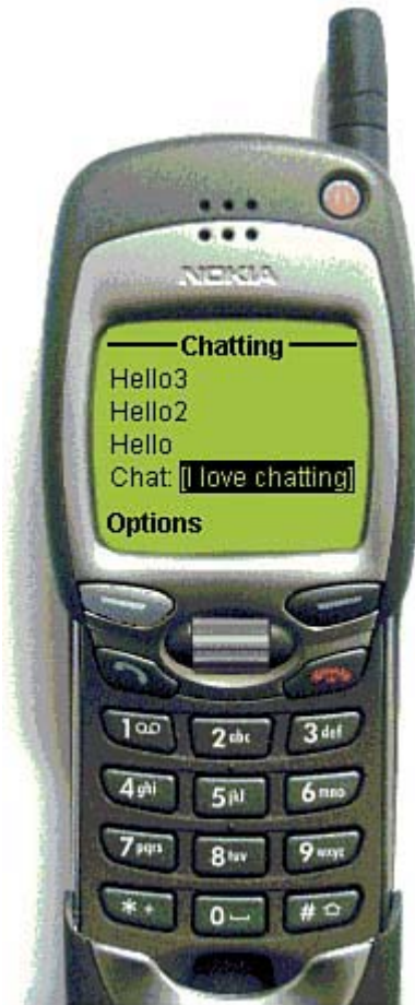
Figure 4.8. A WAP chat application using a servlet.
