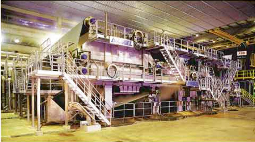
Fig. 5.8 The twin-wire pulp machine at Aracruz Celulose S.A.'s new C line at its Barra do Riacho mill (Knight 2002. Reproduced with permission)
