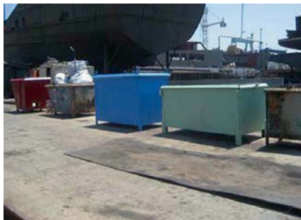
Fig. 39.7 Waste container management system for production wastes in docking area.
