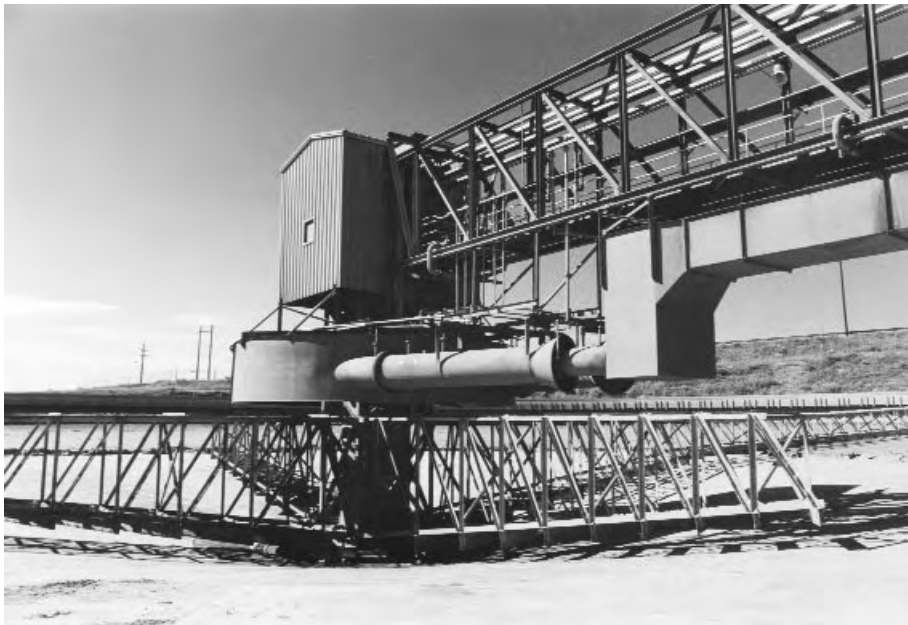
FIG. 18-92 E-Duc® Feed dilution system installed on 122-m-diameter thickener. (EIMCO Process Equipment Co.)
