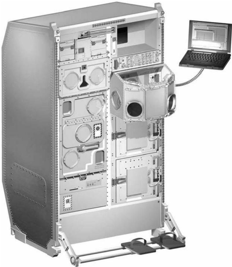
Figure 11.2. Biolab—a multiuser laboratory facility for ISS—for studies on small biological systems. (Courtesy of D. Ducrois, European Space Agency, Paris, France.)
