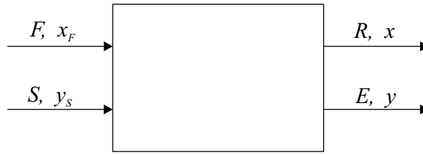
Figure 10.3 Flow diagram for the single-stage mixer settler.
