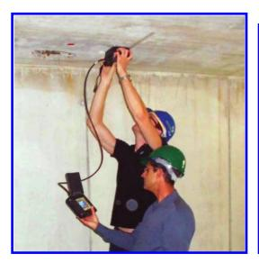
Figure 11. Pulse echo measurement.
