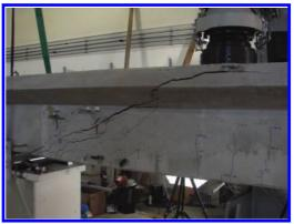
Figure 9. Critical shear crack at beam no. 6.
