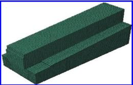
Figure 7. Non-linear finite element crosshead modelling.
