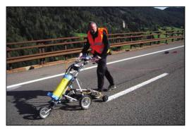
Figure 11. Equipment used for the potential measurements.
