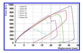
Figure 10. Load versus displacement curves of beams no. 1, 6, 7, 8, 9 and 11.
