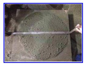
Photo 1. Polymer Modified Self-Compacting Concrete.
