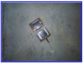
Figure 15. Crack displacement sensor installed on the upper deck of the concrete box girder.
