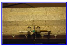
Figure 6. Close-up of the crack-bridging specimen, the stochastic pattern on the testing surface as well as the inductive displacement sensor.
