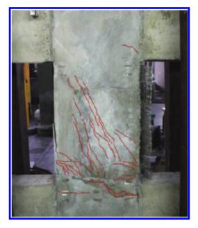
Figure 9. Crack pattern at failure for TRCC retrofitted specimen.
