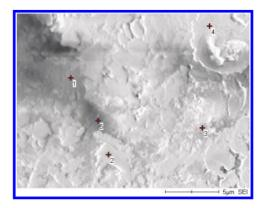
Figure 17. Morphology of C-S-H gel phase of BFS (Up: point 1 C/S = 1.26, point 2 C/S = 1.13, point 3 C/S = 1.26, point 4 C/S = 0.94, and point 5 C/S = 1.18; Down: point 1 C/S = 1.60, point 2 C/S = 1.07, point 3 C/S = 0147, point 4 C/S = 1.14, and point 5 C/S = 2.27) after 8-week extraction.
