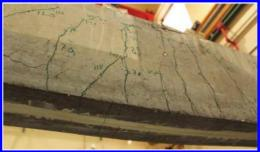
Figure 10. Flexural cracks at the mid-span of Beam-SMA.
