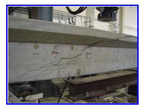
Figure 7. Side view of reference beam after shear failure.
