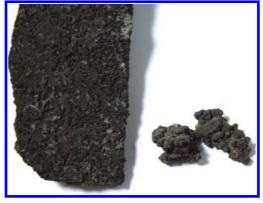
Figure 8. Example of Black crust collected on Saint-Jean de Montmartre church, (Paris, 1894–1904). Locally its thickness exceeds 1 cm.
