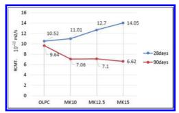
Figure 9. Migration coefficient of RCMT test.
