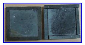
Figure 4. Disk specimens after ECE application.
