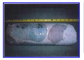
Figure 18. Scale and length of core 1: note size of aggregate.
