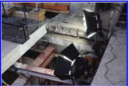
Figure 5. setup of the photogrammetric deformation measure-ment in the support region.
