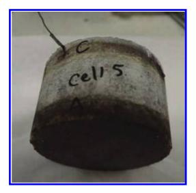
Figure 1. Specimen with embedded titanium mesh (top side).
