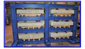
Figure 2. Test setup for simultaneous testing of six beams in a 4-point-flexural-test.
