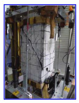
Photo 2. After axial compression test (D4-1).
