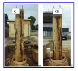
Figure 3. Specimen after corrosion process—crack pattern; a) specimen C; b) specimens CR.
