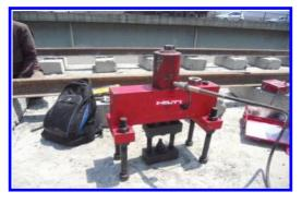
Figure 10. Photo showing pull out testing of anchors in progress.
