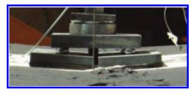
Figure 5. Device for introduction of concentrated force.
