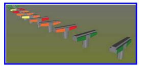
Figure 12. BIM environment showing variation in chloride levels.
