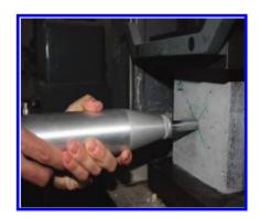
Figure 2. Rebound hammer test on a cubic specimen.
