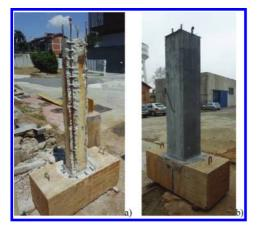
Figure 4. Specimen CR; a) before jacket cast; ) after jacket cast.
