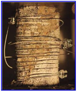
Figure 13. Failure mode of the SMA confined concrete cylinder.
