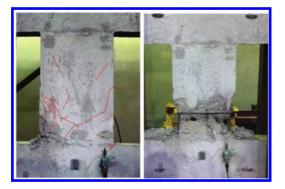
Figure 6. Crack pattern and failure detail: cyclically tested coupling beam with longitudinal and transverse reinforcement.
