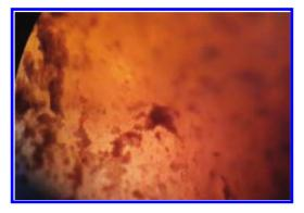
Figure 10. Cracking on the surface of grain, size is 1/19 mm.
