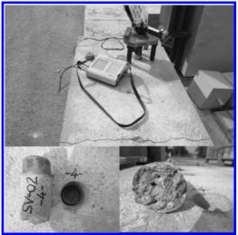
Figure 12. Tensile bond strength tests.
