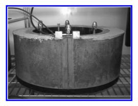
Figure 2. LVDT at the tip of the notch (CTOD): HPC-2 specimen at 21 days.
