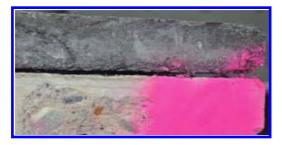
Figure 8. Delamination of R-UHPFRC layer prior to testing.
