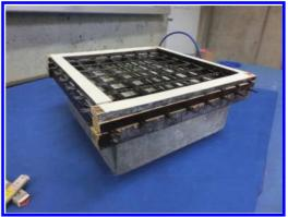
Figure 6. Specimen with carbon textiles before the mortar was filled in.
