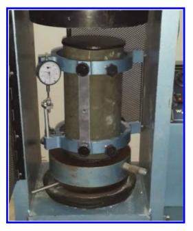
Figure 9. Measuring longitudinal deformation using extensioneter.
