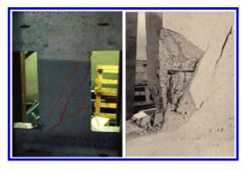
Figure 4. Crack pattern and failure detail of monotonically tested beam with longitudinal and transverse reinforcement.
