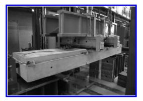
Figure 9. 4-point bending test.
