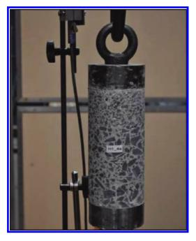
Figure 5. Investigation on the adhesive strength of drilling cores consisting of old (thickness approx. 140 mm) and new concrete (thickness approx. 60 mm).
