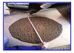
Figure 2. Slump flow test.
