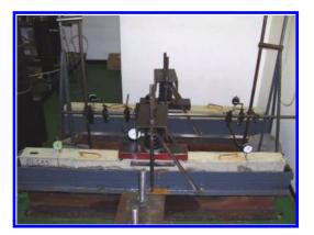
Figure 1. Compressing springs to apply the sustained load and a general view of the loaded frames.
