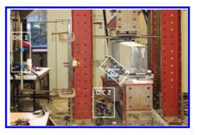
Figure 3. Two DIC systems are used to monitor the cracking behaviour of the beams.
