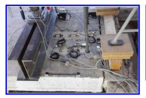
Figure 6. setup of different deformation measurement techniques to monitor the shear section during load testing.
