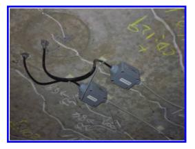
Figure 14. Structural temperature sensors installed inside the concrete structure.
