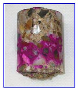
Figure 20. *Maison du Brésil* located in the vicinity of the Parisian beltway (Paris, 1957–1959). Phenolphthalein test on a core indicating a 4 cm carbonation depth.
