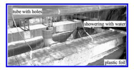
Figure 3. Showering of the concrete beams with water in order to induce autogenous crack healing and trigger the self-healing mechanism based on the use of embedded SAPs.
