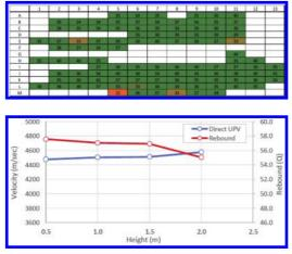
Figure 4. UPV and rebound with height for a shaft wall.
