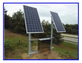
Figure 3. Central measuring and control unit and solar panels.
