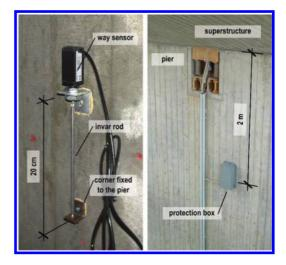
Figure 5. Sensor system for the measurement of concrete strains at the pier head.
