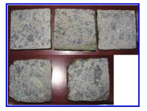
Figure 2. Typical slices from concrete suffered different FT cycles. (From left to right: F52-0, F52-25, F52-175 (the first row), F52-275, F52-325 (the second row), the numbers means FT cycles).
