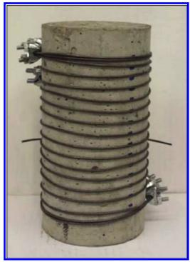
Figure 10. SMA confined concrete cylinder.
