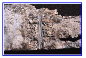
Figure 9. loss of bond at the end-anchorage of the prestressing stands.
