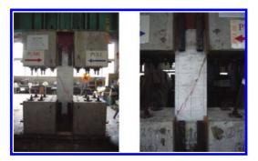
Photo 1. After shear failure test.
