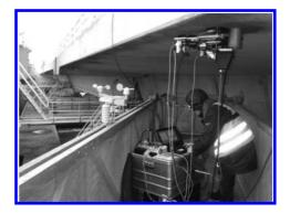
Figure 14. On-site investigation on a bridge. The scanner with the laser-head is fixed with compressed air at the cantilever to estimate the chlorine concentration.
