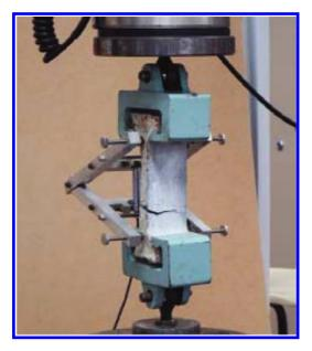
Figure 5. Experimental setup for the direct tensile testing of dog-bone specimens.
