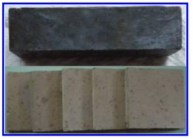
Figure 1. Cement paste specimen and paste disks using in migration cell.
