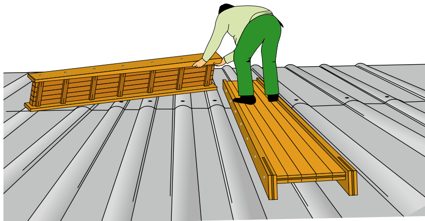
Figure 6.12 Proper precautions must always be taken when working on or near fragile roofs or surfaces.
