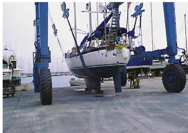
Figure 8.14 Manoeuvring a yacht using a large overhead travelling gantry and slings in a marina
