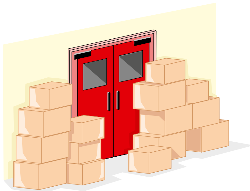
Figure 11.13 Partly blocked fire exit door
