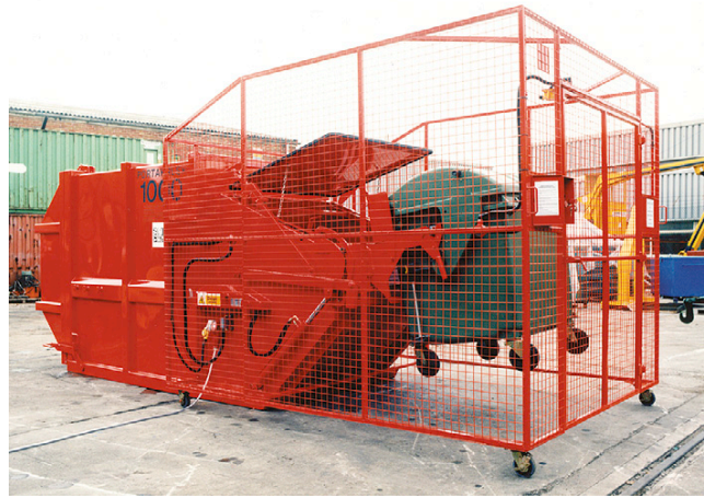
Figure 9.27 Typical retail compactor
