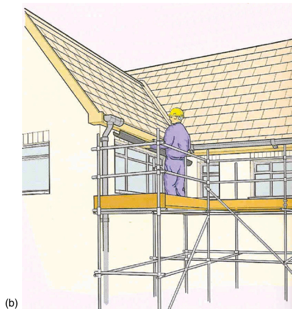
Figure 6.17 (a) Typical independent tied scaffold; (b) fixed scaffold left in place to gutters
