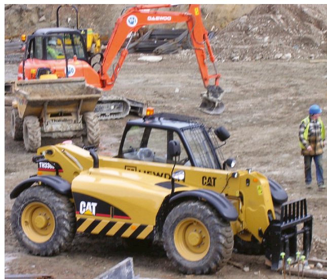
Figure 7.3 Various construction plant with driver protection
