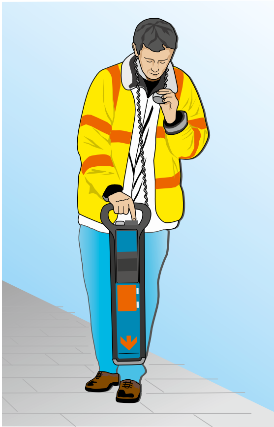
Figure 10.13 Using a cable detector
