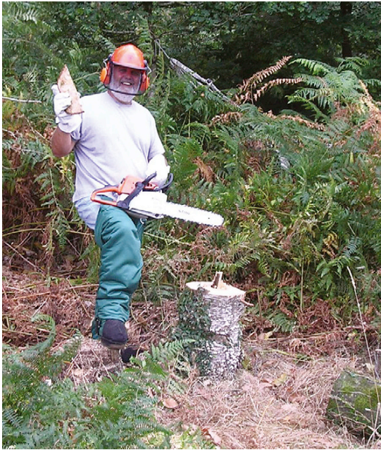
Figure 9.26 Kevlar gloves, overtrousers and overshoes providing protection against chain saw cuts. Helmet ear and face shield protect the head. Apprentice under training – first felling
