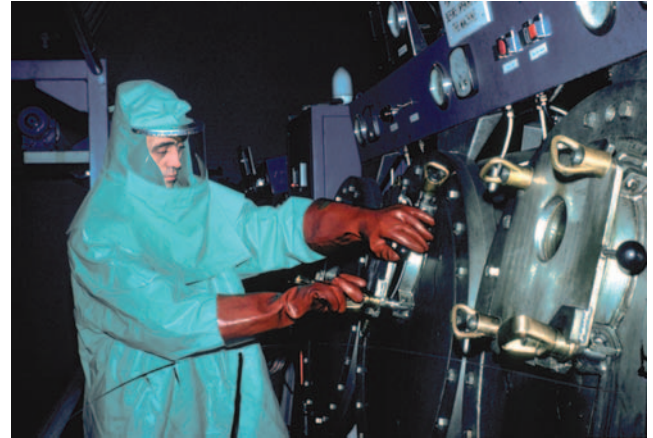
Figure 6.14 PPE used for loading a textile dye vessel.
