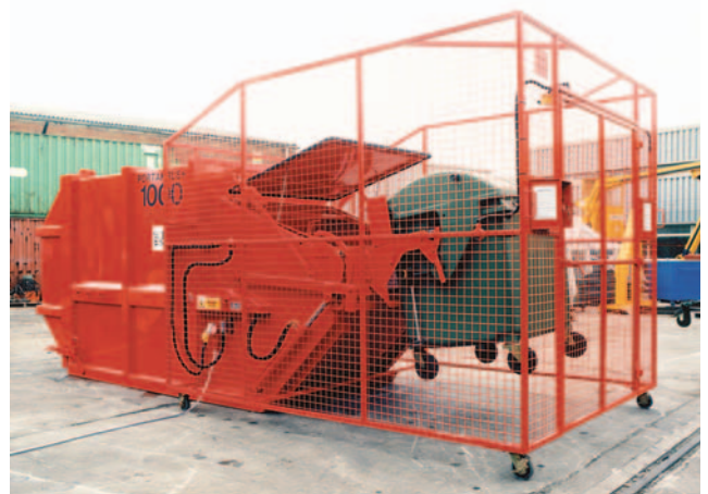
Figure 11.29 Typical retail compactor.
