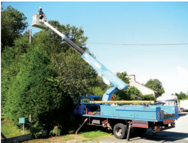
Figure 18.4 Mobile elevating work platform, France.
