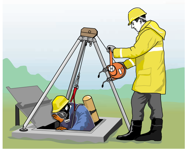
Figure 6.20 Entering a confined space.
