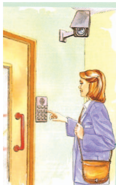
Figure 15.15 Security-coded access and surveillance CCTV camera.
