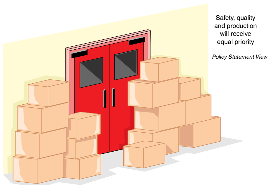
Figure 2.4 Sound policy exists but not put into practice – blocked fire exit.
