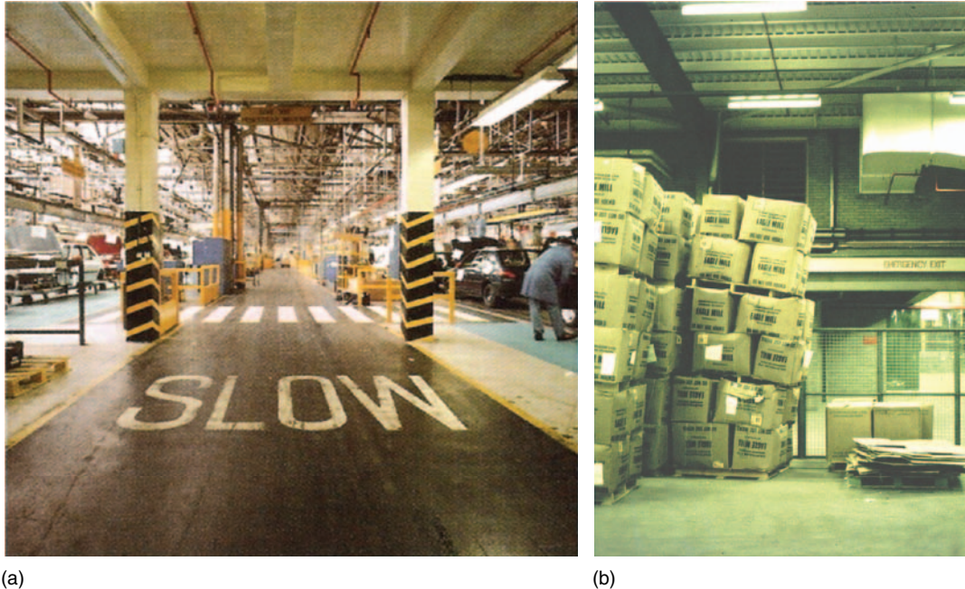
Figure 9.5 (a) Internal roadway with appropriate markings. (b) Unsafe stacks of heavy boxes.
