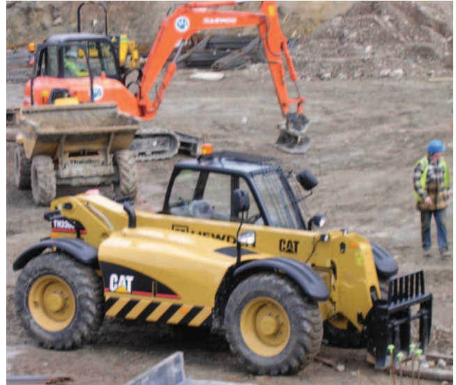
Figure 9.8 Various construction plant with driver protection.
