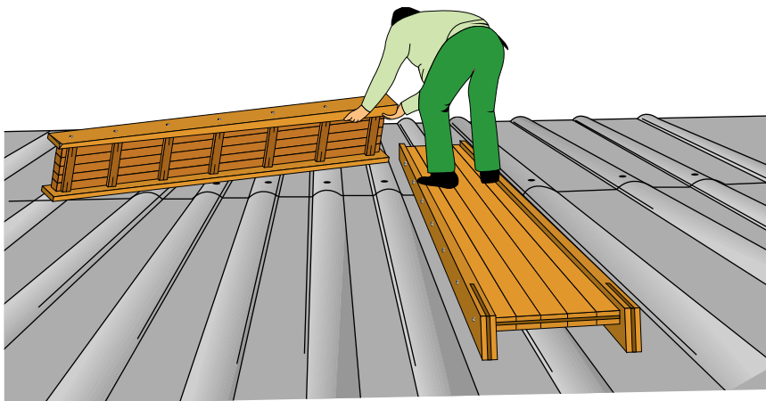
Figure 16.2 Proper precautions must always be taken when working on or near fragile roofs.
