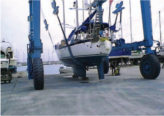
Figure 10.11 Manoeuvring a yacht using a large overhead travelling gantry and slings in a marina.
