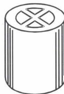
Fig. 6.1.1.2.1. Cross Partition Ring.
