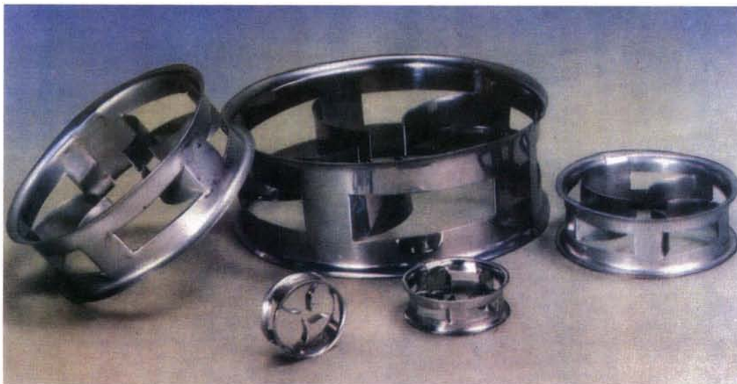
Fig. 6.1.3.3-1. Cascade Mini Rings are Cylindrical Elements With Height Only One-Third of the Outside Diameter. Fingers Punched From The Wall Project Into The Interior Increasing the Interfacial Area of the Packing Element.
