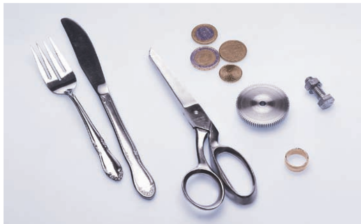
Figure 1.8 Familiar objects that are made of metals and metal alloys (from left to right): silverware (fork and knife), scissors, coins, a gear, a wedding ring, and a nut and bolt.
