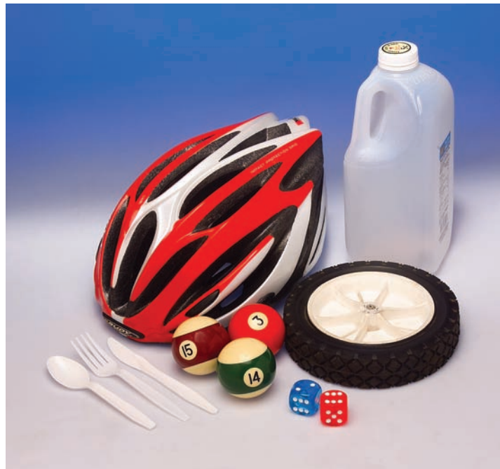
Figure 1.10 Several common objects that are made of polymeric materials: plastic tableware (spoon, fork, and knife), billiard balls, a bicycle helmet, two dice, a lawn mower wheel (plastic hub and rubber tire), and a plastic milk carton.
