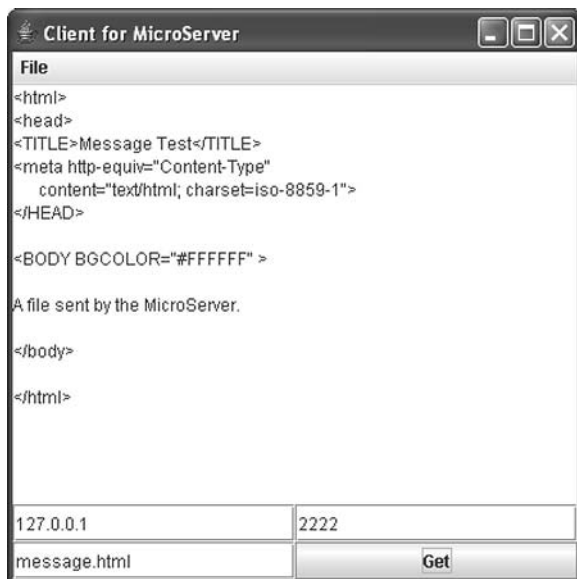
Figure 14.3 The client application – ClientApp – displays a file that it obtained from the MicroServer . The fields in the lower control panel indicate the host name of the server, the port on which to contact the server, and the name of the file to request from the server. Here the server and client ran on the same machine.
