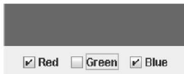
Figure 7.4 The JCheckBox component allows for the selection of more than one item in a set of checkboxes. With CheckBoxesPanel displayed by UITestApplet , the user selects one or more of three color components to create the background color for the top panel.
