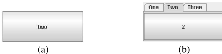
Figure 7.11 (a) A CardLayout only shows one component at a time. (b) A JTabbedPane component, like this one with three tabbed pages, makes clear how many panes are overlapping.
