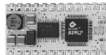
Figure 24.1 The Javelin Stamp module comes as a 24-pin DIP package. See also Figure 24.3, which shows an evaluation card with the Javelin Stamp. (Photo courtesy of Parallax Corp.)
