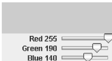
Figure 7.7 The JSlider component allows the user to select from a continuous range of values. With the SliderPanel class displayed in UITestApplet , the three sliders set the Red–Green–Blue component values from 0 to 255 each. The combined RGB values determine the color of the background of the top area.
