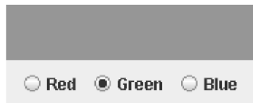
Figure 7.5 The JRadioButton component allows for the selection of only one button in a set of buttons. With RadioButtonsPanel displayed by UiTestApplet , the user selects one of three color components to create the background color for the top panel.
