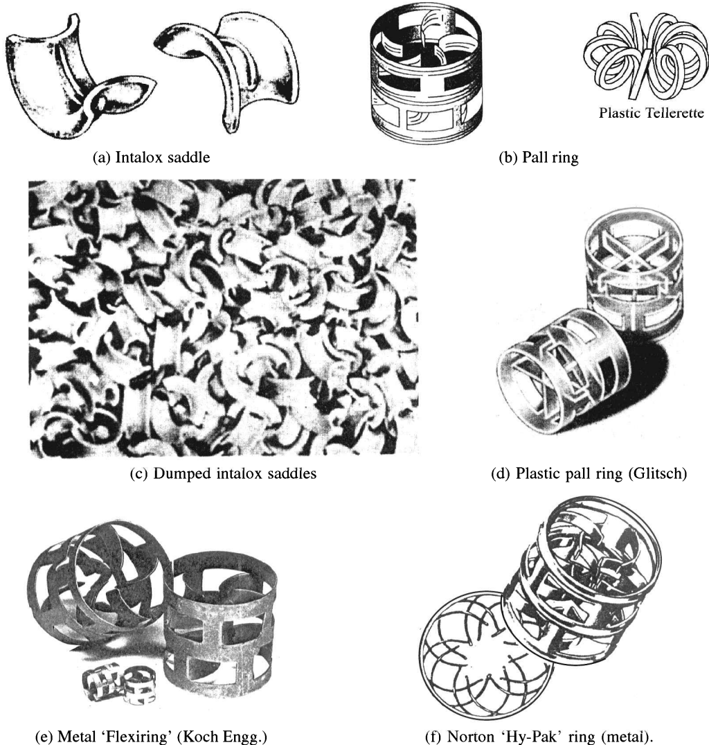
Figure 5.21 Second generation random packings.
