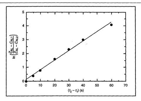
$k_{\rm L}a$  is equal to the slope of the straight line in the plot = 0.069 s<sup>-1</sup>.
