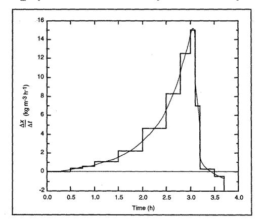
Results for  $\frac{dx}{dt}$  read from the average rate-equal area curve and the calculated specific growth rates are listed below.
