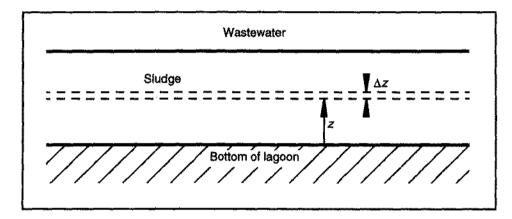
Substrate diffuses into the shell across the upper boundary at  $z+\Delta z$ , and diffuses out across the lower boundary at z. Substrate consumption within the shell follows first-order kinetics. Following the procedure on p 301, from Fick's law, the rate of substrate input by diffusion is:
