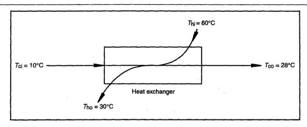
The temperature differences at the two ends of the exchanger are  $\Delta T_1 = (30 - 10) = 20^{\circ}$ C and  $\Delta T_2 = (60 - 28) = 32^{\circ}$ C. Substituting these values into Eq. (8.34) for the log-mean temperature difference:
