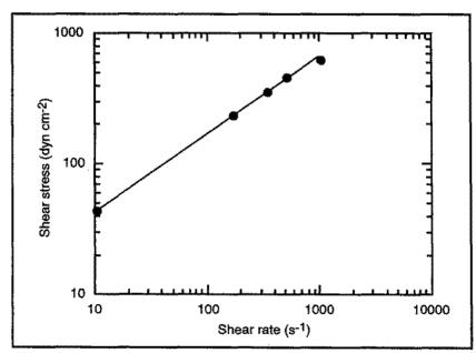
The equation for the straight line in the log-log plot is  $\tau = 11.43 \dot{\gamma}^{0.587}$ . Therefore, the flow behaviour index n = 0.587 and the consistency index K = 11.43 dyn s<sup>n</sup> cm<sup>-2</sup>. The sum of squares of the residuals for this data fit is 1137.
