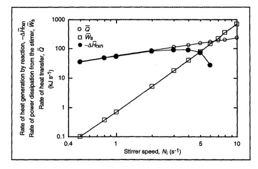
(d) The rate of removal of metabolic heat (the  $-\Delta \hat{H}_{rxn}$  component of  $\hat{Q}$ ) reaches a maximum at around  $N_i = 3 \text{ s}^{-1}$ .
