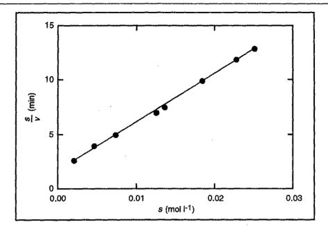
The equation for the straight line in the plot is  $^{s}/_{v} = 1.70 + 445$  s, where s has units of mol  $^{-1}$  and  $^{s}/_{v}$  has units of min. Therefore, from Eq. (11.39),  $^{1}/_{v_{\text{max}}} = 445$  mol  $^{1}$  l min, so that  $v_{\text{max}} = 2.25 \times 10^{-3}$  mol  $^{1-1}$  min  $^{-1}$ . Also from Eq. (11.39),  $^{K}$ m/ $_{v_{\text{max}}} = 1.70$ . Multiplying this value by the result for  $v_{\text{max}}$ ,  $K_{\text{m}} = 3.83 \times 10^{-3}$  mol  $^{1-1}$ .
