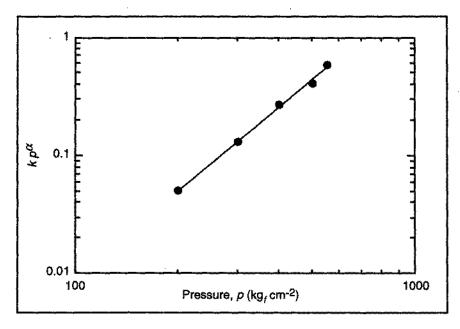
As the equation to the straight line in the plot is  $k p^{\alpha} = 1.71 \times 10^{-7} p^{2.37}$ ,  $\alpha = 2.37$ . Therefore, for this system, Eq. (10.23) becomes:
