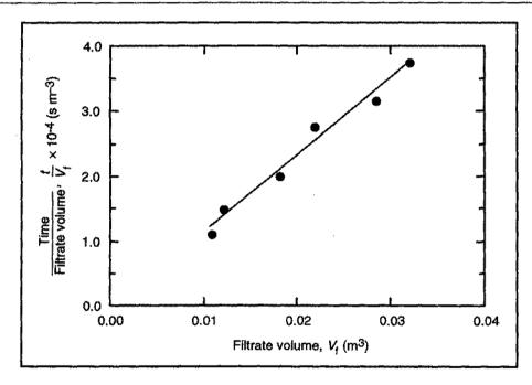
The slope of the straight line in the plot  $K_1 = 1.18 \times 10^6$  s m<sup>-6</sup>; the intercept  $K_2 = -363$  s m<sup>-3</sup>. From Eq. (10.13), using the conversion factors 1 mmHg =  $1.333 \times 10^2$  kg m<sup>-1</sup> s<sup>-2</sup> (Table A.5, Appendix A) and 1 cP =  $10^{-3}$  kg m<sup>-1</sup> s<sup>-1</sup> (Table A.9, Appendix A), the specific cake resistance  $\alpha$  is:
