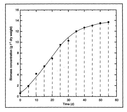
The growth rate dx/dt is determined using the central-difference formula, Eq. (11.23). These results and values of the specific growth rate  $\mu$  are listed and plotted below as a function of time.
