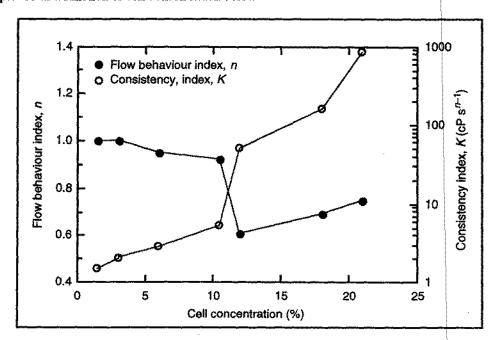
The cell broth is Newtonian up to a cell concentration of about 2%, then becomes pseudoplastic. The flow behaviour index continues to decrease until a cell concentration of about 12% is reached. The consistency index rises throughout the culture with increasing cell concentration.
