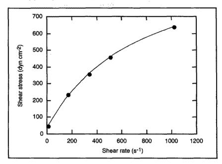
(b) The rheogram in (a) is similar to those for pseudoplastic and Casson plastic fluids in Figure 7.7. It is not clear from the rheogram whether the fluid exhibits a yield stress at  $\dot{\gamma}=0$  or not; therefore, both non-Newtonian models are worth checking. From the equation in Figure 7.7 for pseudoplastic fluids, a plot of shear stress versus shear rate on log-log coordinates would be expected to give a straight line. This plot is shown below.
