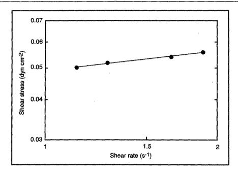
The equation for the straight line on the log-log plot is  $\tau = 0.049 \dot{\gamma}^{0.20}$ . From Eq. (7.7), this means that the flow behaviour index n is 0.20 and the consistency index K is 0.049 N s<sup>n</sup> m<sup>-2</sup>.
