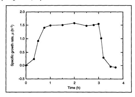
As expected for most batch cell cultures, growth occurs at around the maximum specific growth rate for most of the culture period. Taking the average of the values of  $\mu$  between times 0.75 h and 3 h,  $\mu_{\text{max}} = 1.50 \pm 0.05 \text{ h}^{-1}$ , where 0.05 is the standard deviation.
