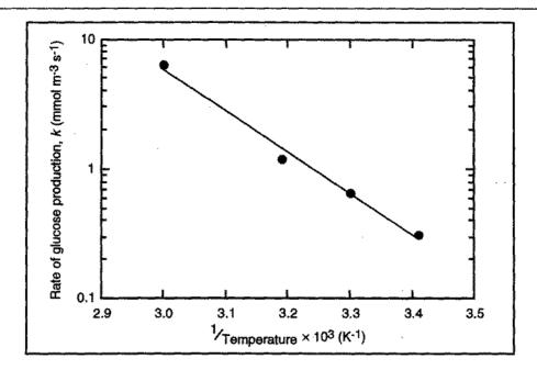
The equation for the straight line in the plot is  $k = 1.87 \times 10^{10} \ e^{-7300/T}$ , where k has units of mmol m<sup>-3</sup> s<sup>-1</sup> and T has units of K. Therefore, from Eq. (11.21),  $E/R = 7300 \ \text{K}$ . From Table 2.5,  $R = 8.3144 \ \text{J K}^{-1} \ \text{gmol}^{-1} = 8.3144 \times 10^{-3} \ \text{kJ K}^{-1} \ \text{gmol}^{-1}$ ; therefore,  $E = 7300 \ \text{K} \times 8.3144 \times 10^{-3} \ \text{kJ K}^{-1} \ \text{gmol}^{-1} = 60.7 \ \text{kJ gmol}^{-1}$ .
