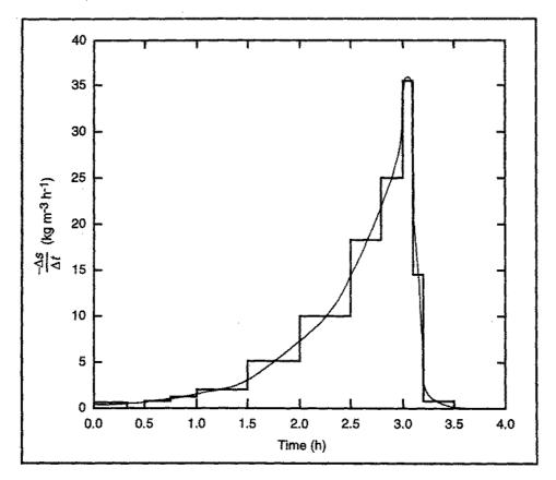
Results for  $^{-ds}/_{dt}$  read from the average rate-equal area curve are listed below, together with the instantaneous biomass yield coefficients calculated using Eq. (11.49) and the values of  $r_X$  from (a).
