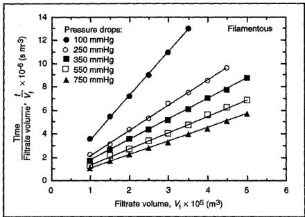
From Eq. (10.12), the slopes of the straight lines in the plots are equal to  $K_1$  for each pressure drop. These values are listed below.
