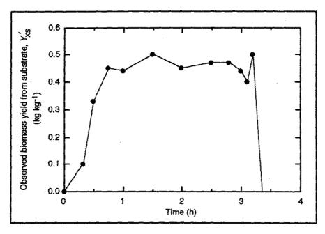
During the exponential growth phase between 0.75 h and 3 h when  $\mu = \mu_{\text{max}}$ ,  $Y_{\text{XS}}$  is approximately constant with an average value of 0.46  $\pm$  0.02 kg kg<sup>-1</sup>, where 0.02 is the standard deviation.
