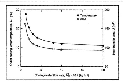
From the equations developed in (c), at a cooling-water flow rate of  $5 \times 10^5$  kg h<sup>-1</sup>,  $T_{co} = 14.3$ °C and A = 101 m<sup>2</sup>. The area A of a cylindrical cooling-coil is equal to  $2 \pi r L$ , where r is the cylinder radius and L is its length. For a radius of 5 cm = 0.05 m:
