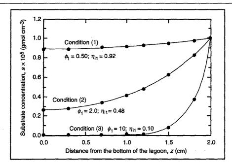
As  $\phi_1$  increases,  $\eta_{11}$  decreases, the concentration profile becomes steeper, and the minimum substrate concentration in the sludge is reduced.
