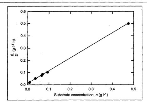
The slope of the straight line in the plot is 1.027 h; the intercept is 0.0119 g l<sup>-1</sup> h. From Eq. (13.92), the slope =  $^{1}/\mu_{\text{max}}$ ; therefore,  $\mu_{\text{max}} = ^{1}/_{1.027}$  h = 0.97 h<sup>-1</sup>. The intercept =  $^{K}\text{S}/\mu_{\text{max}}$ ; therefore  $K_{\text{S}} = 0.0119$  g l<sup>-1</sup> h × 0.97 h<sup>-1</sup> = 0.012 g l<sup>-1</sup>.
