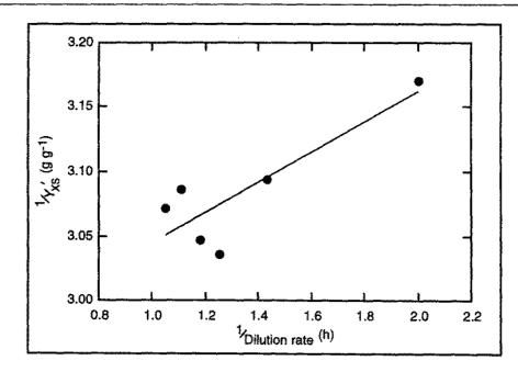
The scatter in the plot is typical for measured values of  $1/\gamma'_{XS}$ . The slope of the straight line in the plot is 0.12 g g<sup>-1</sup> h<sup>-1</sup>; the intercept is 2.93 g g<sup>-1</sup>. From Eq. (13.93), the slope =  $m_S$ ; therefore  $m_S = 0.12$  g g<sup>-1</sup> h<sup>-1</sup>. The intercept =  $1/\gamma_{XS}$ ; therefore  $\gamma_{XS} = 1/2.93$  h<sup>-1</sup> = 0.34 g g<sup>-1</sup>.
