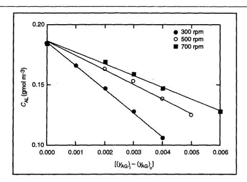
(a) The slopes of the straight lines in the plot for 300, 500 and 700 rpm are -19.58, -12.04 and -9.68 gmol m<sup>-3</sup>, respectively. These values can be used to determine  $k_{\rm L}a$  using R = 0.000082057 m<sup>3</sup> atm gmol<sup>-1</sup> K<sup>-1</sup> from Table 2.5 and converting the temperature to degrees Kelvin using Eq. (2.24):
