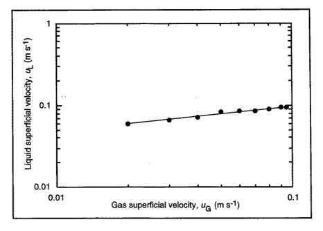
The data are reasonably well fitted using a power law model. The equation for the straight line in the plot is:
