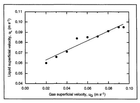
The data are reasonably well fitted using a linear model. The linear least squares equation for the straight line fit is:
