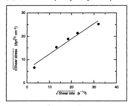
The equation for the straight line in the plot is  $\tau^{1/2} = 5.93 + 0.648 \dot{\gamma}^{1/2}$ . From the equation in Figure 7.7, this means that  $K_p = 0.648 \,\mathrm{dyn}^{1/2} \,\mathrm{s}^{1/2} \,\mathrm{cm}^{-1}$  and the yield stress  $\tau_0 = 35.2 \,\mathrm{dyn} \,\mathrm{cm}^{-2}$ . The sum of squares of the residuals for this data fit is 8986.
