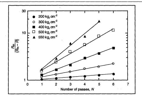
The values of  $k p^{\alpha}$  obtained from the slopes of the straight lines for each pressure are listed below.
