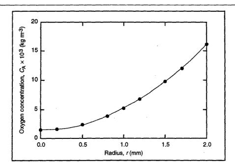
As the minimum value of  $C_A$  at the centre of the bead is still about 2.9 times  $K_m$ , the assumption of zero-order kinetics is reasonable.
