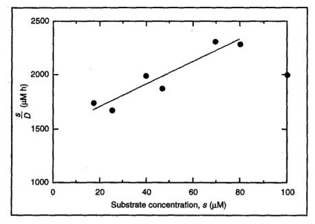
The slope of the straight line in the plot is 10.48 h; the intercept is 1493  $\mu$ M h. From Eq. (13.92), the slope =  $^{1}/\mu_{max}$ ; therefore,  $\mu_{max} = ^{1}/_{10.48}$  h = 0.095 h<sup>-1</sup>. The intercept =  $^{K_S}/_{\mu_{max}}$ ; therefore  $K_S = 1493$   $\mu$ M h × 0.095 h<sup>-1</sup> = 142  $\mu$ M.
