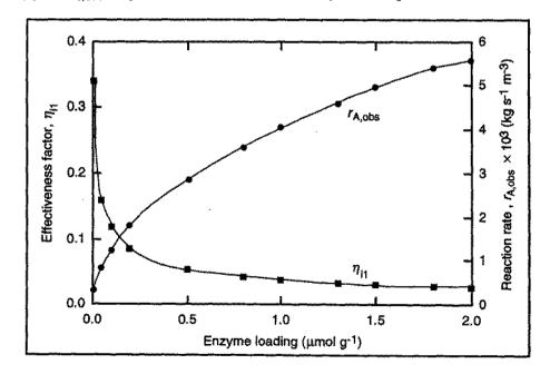
As the enzyme loading is increased from  $0.01 \mu mol g^{-1}$ , the effectiveness factor drops significantly. Although the reaction rate continues to rise with increasing enzyme loading, at loadings above about  $0.5 \mu mol g^{-1}$ , less than 5% of the potential activity of the enzyme is being utilised. Further increases in enzyme loading therefore represent an effective waste of more than 95% of that enzyme.
