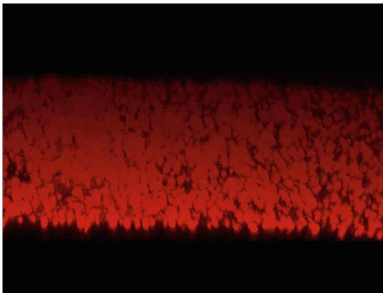
Fig. 9 Confocal laser scanning microscopy 3D rendering of PCL-patterned scaffold containing PCL nanospheres mixed into at a ratio of 4:1 PCL:PLGA spheres. Texas Red was mixed into the PLGA during the emulsion process in order to visualize them
