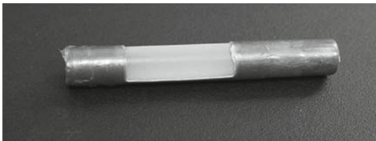
Fig. 11 A nanoporous capsule for encapsulating insulin producing cells
