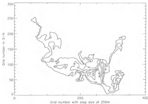
Fig. 5 Suspended sediment concentrations in mg/l in the Oder Estuary under calm wave climate
