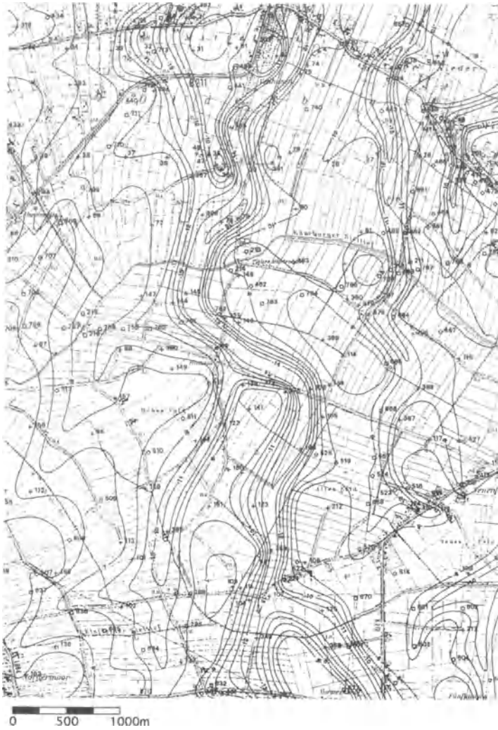
Fig.6 Detail of the manually constructed structure contour map of the base of the Holocene accumulation wedge. Topographic base: 1:25 000 map sheet 2716 (Elsfleth). (With permission of the Niedersächsisches Landesverwaltungsamt – Landesvermessung – dated 29 Nov. 1996 Az.: B4 - 2005/97)
