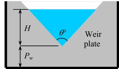
Therefore, the discharge rate is proportional to the tangent of the half notch angle, and the ratio of discharge rates is calculated to be
