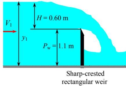
**Assumptions** 1 The flow is steady. 2 The upstream velocity head is negligible. 3 The channel is sufficiently wide so that the end effects are negligible.
