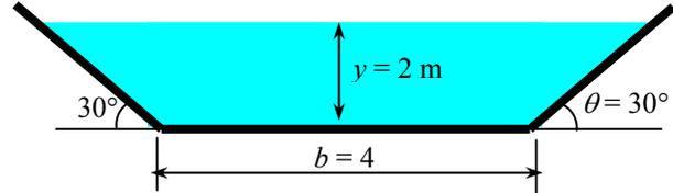
Bottom slope of the channel is  $S_0 = 0.001$ . Then the flow rate can be determined from Manning's equation to be
