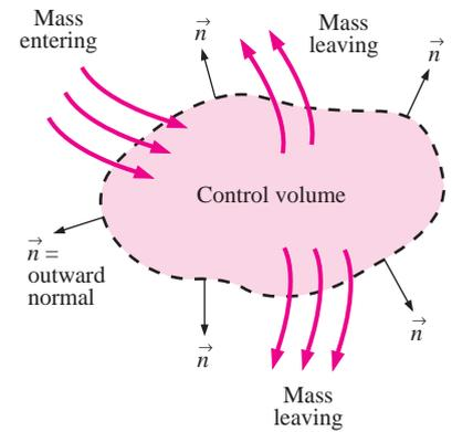
$$\dot{B}_{\text{net}} = \dot{B}_{\text{out}} - \dot{B}_{\text{in}} = \int_{\text{CS}} \rho b \vec{V} \cdot \vec{n} dA$$
