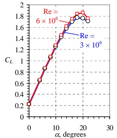
**Discussion** The behavior of the lift and drag coefficients beyond stall is not as dramatic as we might have expected. Why? The flow becomes *unsteady* for angles of attack beyond the stall angle. However, we are performing *steady* calculations. For higher angles, the run does not even converge; the CFD calculation is stopped because it has exceeded the
