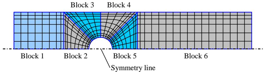
With the block structure of Fig. 1 no cells are highly skewed, and cells are clustered near the cylinder wall and the upper wall of the duct as desired.
