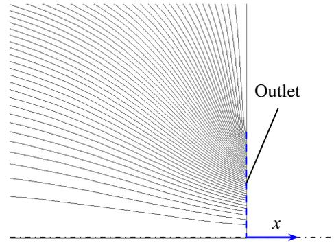
**Discussion** Newer versions of FlowLab may give slightly different results. The error in  $\Delta P$  caused by neglecting the downstream extension is significant. This reinforces our discussion in the text about extending outlets.
