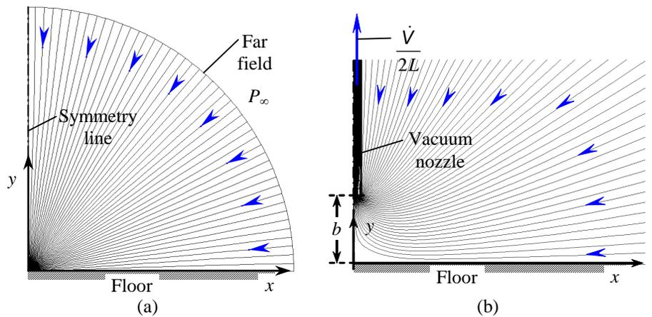
**FIGURE 2** CFD calculations of flow into the nozzle of a vacuum cleaner; (a) streamlines in the entire flow domain, (b) close-up view of streamlines, (c) contours of constant magnitude of vorticity illustrating regions where the irrotational flow approximation is valid, and (d) comparison of pressure coefficient with that predicted by the irrotational flow approximation.
