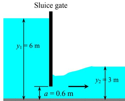
**Discussion** Note that the use of the discharge coefficient enables us to determine the flow rate through sluice gates by measuring 3 flow depths only.
