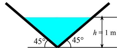
The bottom slope of the channel is  $S_0 = \tan 0.5^\circ = 0.008727$ .
