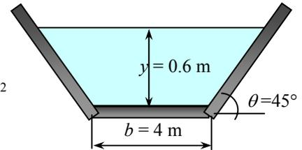
When calculating the Froude number, the hydraulic depth should be used rather than the maximum depth or the hydraulic radius. For a non-rectangular channel, hydraulic depth is defined as the ratio of the flow area to top width,
