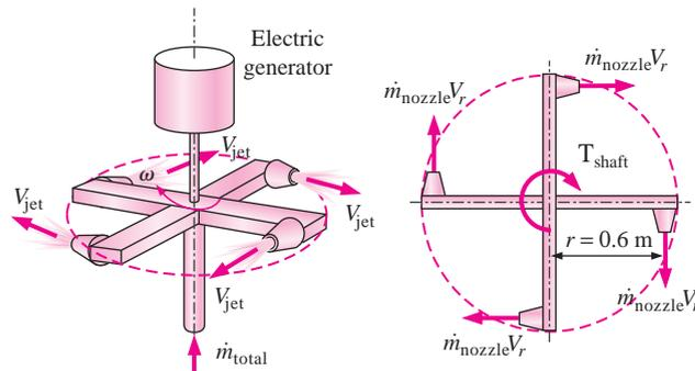
**FIGURE 6–38** Schematic for Example 6–9 and the free-body diagram.
