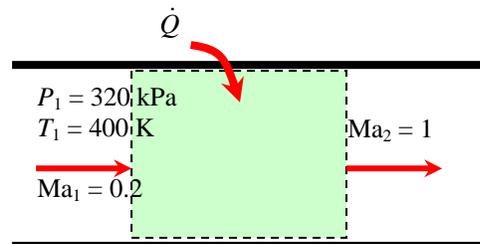
The Rayleigh flow functions corresponding to the inlet and exit Mach numbers are
