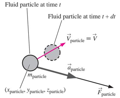
**FIGURE 4–6** Newton’s second law applied to a fluid particle; the acceleration vector (gray arrow) is in the same direction as the force vector (black arrow), but the velocity vector (blue arrow) may act in a different direction.
