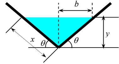
Now we apply the criterion that the best hydraulic cross-section for an open channel is the one with the minimum wetted perimeter for a given cross-section. Taking the derivative of  $p$  with respect to  $\theta$  while holding  $A_c$  constant gives
