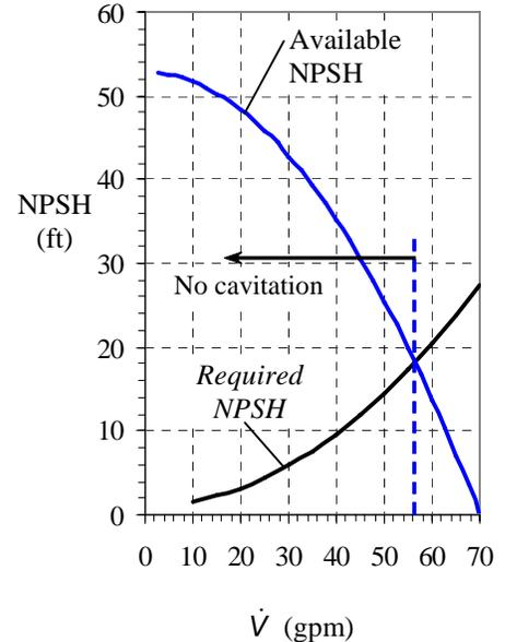
$$\text{NPSH} = \frac{(2116.2 - 66.19) \text{ lbf/ft}^2}{(62.24 \text{ lbm/ft}^3)(32.174 \text{ ft/s}^2)} \left( \frac{32.174 \text{ lbf ft}}{\text{s}^2 \text{ lbf}} \right) + 20.0 \text{ ft} - \left( 0.0174 \frac{12.0 \text{ ft}}{0.10 \text{ ft}} + 6.8 \right) \frac{(11.35 \text{ ft/s})^2}{2(32.174 \text{ ft/s}^2)} = 35.1 \text{ ft} \quad (7)$$
