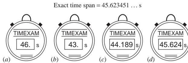
precise than a digital voltmeter with only three digits. However, the number of displayed digits has nothing to do with the overall *accuracy* of the measurement. An instrument can be very precise without being very accurate when there are significant bias errors. Likewise, an instrument with very few displayed digits can be more accurate than one with many digits (Fig. 1–43).
