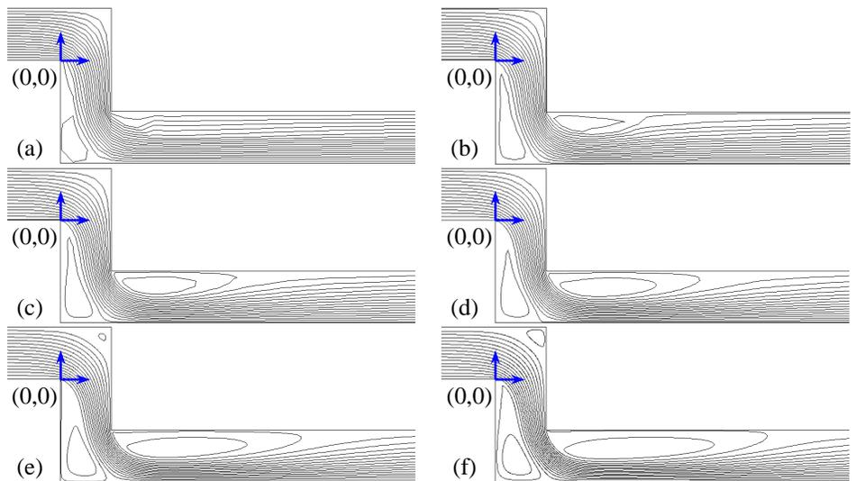
**FIGURE 1** Streamlines for steady, incompressible, two-dimensional, turbulent flow through a jog in a channel at various levels of grid resolution: cell count = (a) 900, (b) 2500, (c) 5700, (d) 9100, (e) 13,600, and (f) 18,000. The origin (0,0) is marked on each figure for reference.
