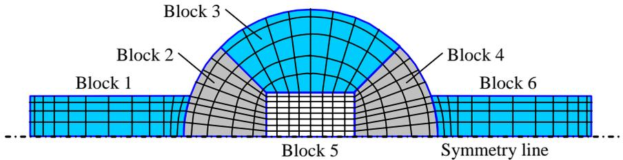
The setup of Fig. 1 contains six blocks. With this block structure, no cells are highly skewed, and cells are clustered near upper wall of the duct as desired. Cells are also clustered at the junctions between Blocks 1 and 2 and Blocks 4 and 6, where flow separation may occur.
