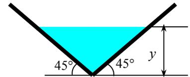
This channel at these flow conditions is classified as **mild** since  $y > y_c$ , and the flow is subcritical.
