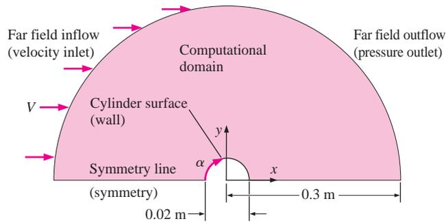
Computational domain (light blue shaded region) used to simulate steady two-dimensional flow over a circular cylinder (not to scale). It is assumed that the flow is symmetric about the  $x$ -axis. Applied boundary conditions are shown for each edge in parentheses. We also define  $\alpha$ , the angle measured along the cylinder surface from the front stagnation point.
