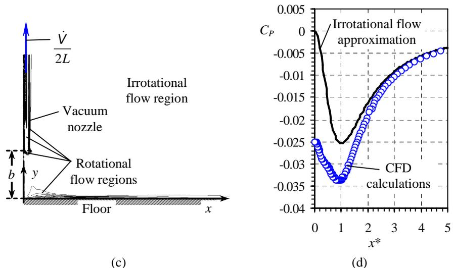
We see from Fig. 2c that vorticity is negligibly small everywhere in the flow field except close to the floor, along the vacuum nozzle wall, near the inlet of the nozzle, and inside the nozzle duct. In these
