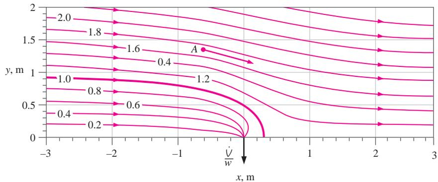
The thick streamline in Fig. 9–25 is called the **dividing streamline** because it divides the flow into two parts. Namely, all the water below this dividing streamline gets sucked into the slot, while all the water above the dividing streamline continues on its way downstream. What is the volume flow rate of water being sucked through the slot? Estimate the magnitude of the velocity at point A.
