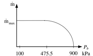
**Discussion** We see from the plots that once the flow is choked at a back pressure of 475.5 kPa, the mass flow rate remains constant regardless of how low the back pressure gets.
