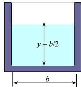
**Discussion** The concept of best cross-section is an important consideration in the design of open channels because it directly affects the construction costs.
