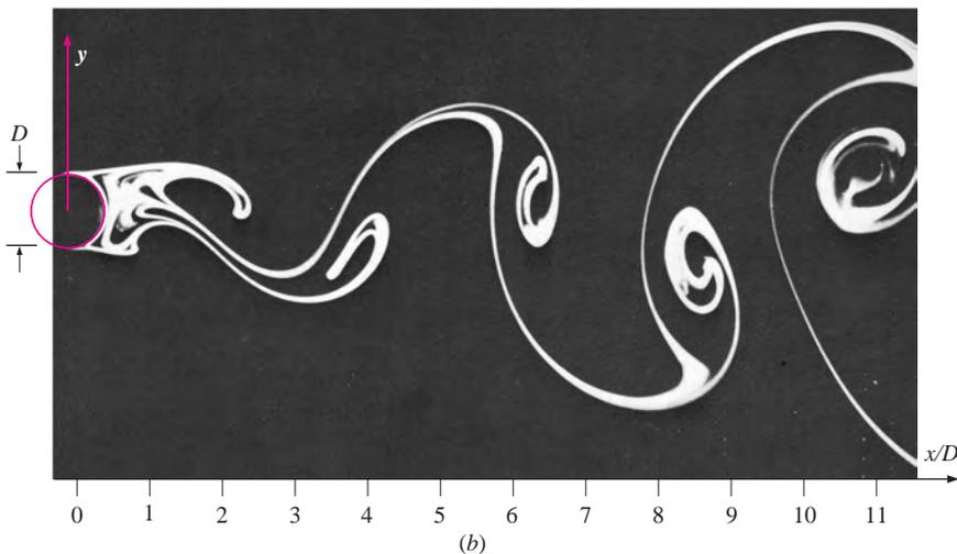
**FIGURE 15-40** Close-up view of vortices shedding from a circular cylinder: (a) instantaneous vorticity contour plot produced by CFD at  $Re = 150$ , and (b) dye streaklines produced by dye introduced at the cylinder surface at  $Re = 140$ . An animated version of this CFD picture is available on the book’s website.
