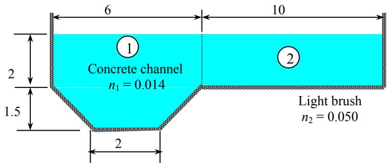
The flow area, perimeter, and hydraulic radius for each subsection and the entire channel are:
