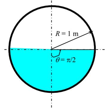
Then the flow rate can be determined from Manning's equation to be
