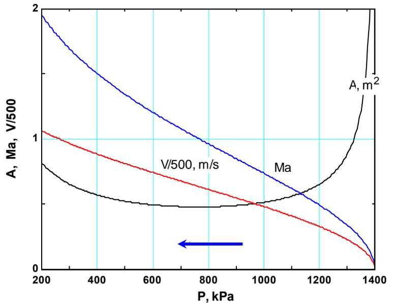
**Discussion** We are assuming that the back pressure is sufficiently low that the flow is choked at the throat, and the flow downstream of the throat is supersonic without any shock waves. Mach number and velocity continue to rise right through the throat into the diverging portion of the nozzle, since the flow becomes supersonic.
