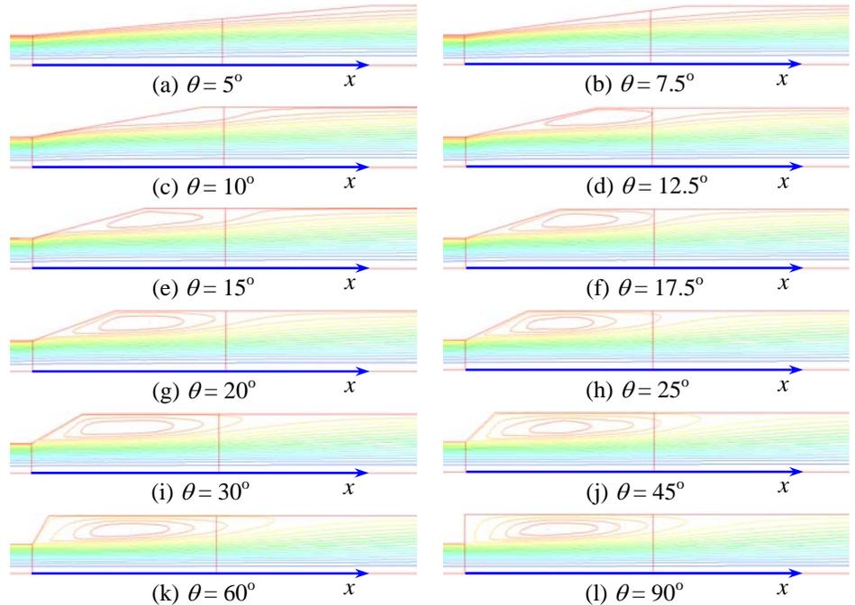
**FIGURE 1** Streamlines for steady, incompressible, axisymmetric, turbulent flow through a diffuser at various values of diffuser half-angle:  $\theta =$  (a)  $5^\circ$ , (b)  $7.5^\circ$ , (c)  $10^\circ$ , (d)  $12.5^\circ$ , (e)  $15^\circ$ , (f)  $17.5^\circ$ , (g)  $20^\circ$ , (h)  $25^\circ$ , (i)  $30^\circ$ , (j)  $45^\circ$ , (k)  $60^\circ$ , and (l)  $90^\circ$ . (The latter case is a sudden expansion.)
