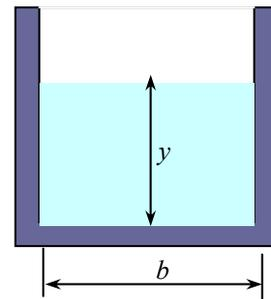
**Discussion** It is clear from the table and the chart that the depth-to-width ratio of  $y/b = 0.5$  corresponds to the best cross-section for an open channel of rectangular cross-section.
