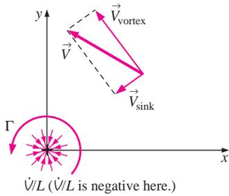
**FIGURE 10-57** Superposition of a line source of strength  $\dot{V}/L$  and a line vortex of strength  $\Gamma$  located at the origin. Vector velocity addition is shown at some arbitrary location in the  $xy$ -plane.
