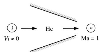
The ratio of the nozzle inlet area to the throat area is determined from
