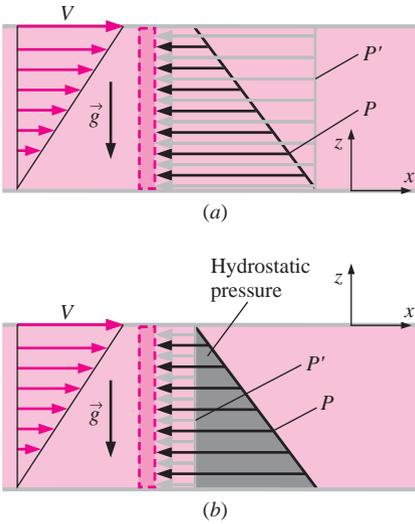
**FIGURE 10-5** Pressure and modified pressure distribution on the right face of a fluid element in Couette flow between two infinite, parallel, horizontal plates: (a)  $z = 0$  at the bottom plate, and (b)  $z = 0$  at the top plate. The *modified pressure*  $P'$  is constant, but the *actual pressure*  $P$  is not constant in either case. The shaded area in (b) represents the hydrostatic pressure component.
