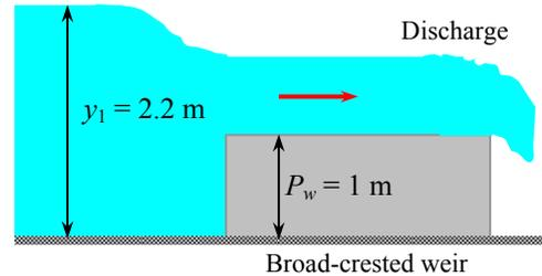
The minimum flow depth above the weir is the critical depth, which is determined from
