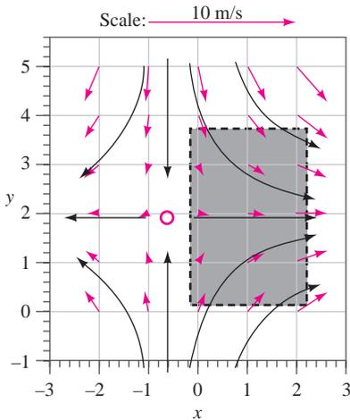
**FIGURE 4-4** Velocity vectors for the velocity field of Example 4-1. The scale is shown by the top arrow, and the solid black curves represent the approximate shapes of some streamlines, based on the calculated velocity vectors. The stagnation point is indicated by the blue circle. The shaded region represents a portion of the flow field that can approximate flow into an inlet (Fig. 4-5).
