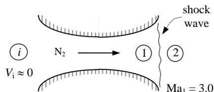
The fluid properties after the shock (denoted by subscript 2) are related to those before the shock through the functions listed in Table A-14. For  $\text{Ma}_1 = 3.0$  we read
