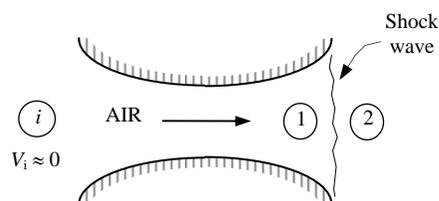
The fluid properties after the shock (denoted by subscript 2) are related to those before the shock through the functions listed in Table A-14. For  $\text{Ma}_1 = 2.0$  we read
