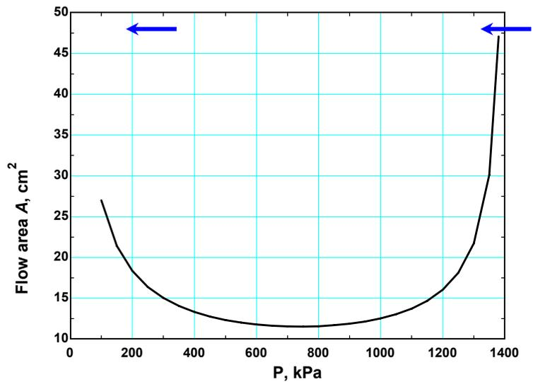
**Discussion** The shape is not actually to scale since the horizontal axis is pressure rather than distance. If the pressure decreases linearly with distance, then the shape *would* be to scale.
