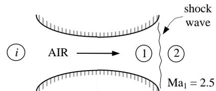
Then the stagnation pressure  $P_{02}$ , static pressure  $P_2$ , and static temperature  $T_2$ , are determined to be
