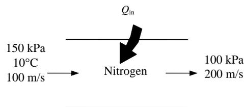
From the energy balance relation  $E_{\text{in}} - E_{\text{out}} = \Delta E_{\text{system}}$  with  $w = 0$
