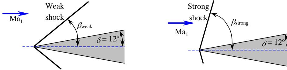
**Assumptions** 1 The flow is steady. 2 The boundary layer on the wedge is very thin. 3 Air is an ideal gas with constant specific heats.
