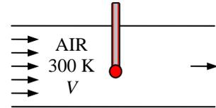
**Discussion** Note that the stagnation temperature is nearly identical to the thermodynamic temperature at low velocities, but the difference between the two is significant at high velocities.
