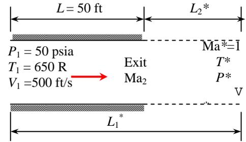
$$T_1 = T_{01} - \frac{V_1^2}{2c_p} = 650 \text{ R} - \frac{(500 \text{ ft/s})^2}{2 \times 0.2400 \text{ Btu/lbm}\cdot\text{R}} \left( \frac{1 \text{ Btu/lbm}}{25,037 \text{ ft}^2/\text{s}^2} \right) = 629.2 \text{ R}$$
