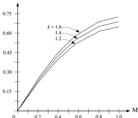
**Discussion** Note that the mass flow rate increases with increasing Mach number and specific heat ratio. It levels off at  $\text{Ma} = 1$ , and remains constant (choked flow).
