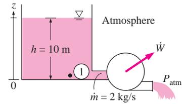
$$\begin{aligned} \dot{W}_{\text{max}} &= \dot{m} \frac{P_1 - P_{\text{atm}}}{\rho} = \dot{m} \frac{\rho gh}{\rho} = \dot{m} gh \\ &= (2 \text{ kg/s})(9.81 \text{ m/s}^2)(10 \text{ m}) \\ &= 196 \text{ W} \end{aligned}$$
