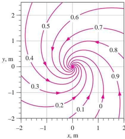
**FIGURE 10-58** Streamlines created by superposition of a line sink and a line vortex at the origin. Values of  $\psi$  are in units of  $\text{m}^2/\text{s}$ .
