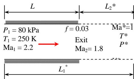
**Assumptions** 1 The assumptions associated with Fanno flow (i.e., steady, frictional flow of an ideal gas with constant properties through a constant cross-sectional area adiabatic duct) are valid. 2 The friction factor remains constant along the duct.
