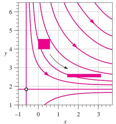
**FIGURE 4–41** Deformation of an initially square parcel of marked fluid subjected to the velocity field of Example 4–6 for a time period of 1.5 s. The stagnation point is indicated by the circle at  $x = -0.625 \text{ m}$  and  $y = 1.875 \text{ m}$ , and several streamlines are plotted.
