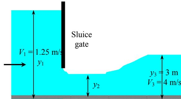
**Assumptions** 1 The flow is steady or quasi-steady. 2 The channel is sufficiently wide so that the end effects are negligible.
