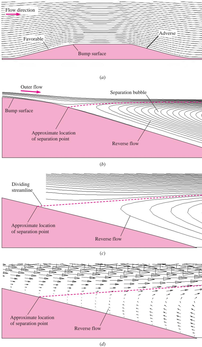
**FIGURE 10-124** CFD calculations of flow over a bump: (a) solution of the Euler equation with outer flow streamlines plotted (no flow separation), (b) laminar flow solution showing flow separation on the downstream side of the bump, (c) close-up view of streamlines near the separation point, and (d) close-up view of velocity vectors, same view as (c).
