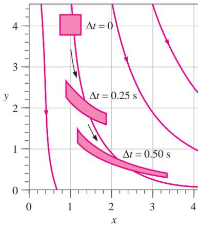
**FIGURE 4-47** Deformation of an initially square fluid parcel subjected to the velocity field of Example 4-8 for a time period of 0.25 s and 0.50 s. Several streamlines are also plotted in the first quadrant. It is clear that this flow is *rotational*.
