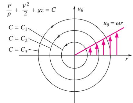
**FIGURE 10–20** Solid body rotation is an example of an inviscid region of flow that is also rotational. The Bernoulli constant  $C$  differs from streamline to streamline but is constant along any particular streamline.
