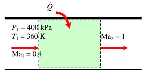
The Rayleigh flow functions corresponding to the inlet and exit Mach numbers are  $T_{02}/T_0^* = 1$  (since  $\text{Ma}_2 = 1$ )
