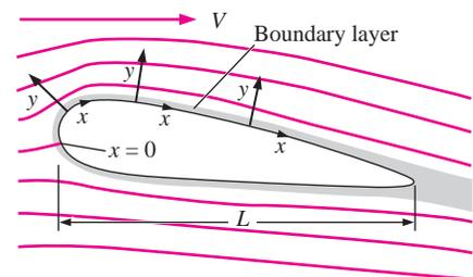
**FIGURE 10–85** The boundary layer coordinate system for flow over a body;  $x$  follows the surface and is typically set to zero at the front stagnation point of the body, and  $y$  is everywhere normal to the surface locally.
