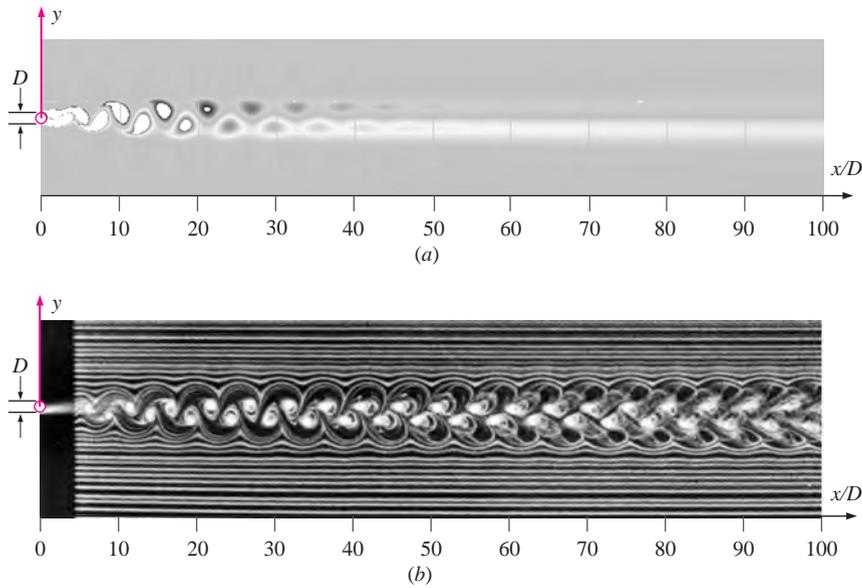
**FIGURE 15-39** Laminar flow in the wake of a circular cylinder at  $Re \cong 150$ : (a) an instantaneous snapshot of vorticity contours produced by CFD, and (b) time-integrated streaklines produced by a smoke wire located at  $x/D = 5$ . The vorticity contours show that Kármán vortices decay rapidly in the wake, whereas the streaklines retain a “memory” of their history from upstream, making it appear that the vortices continue for a great distance downstream.
