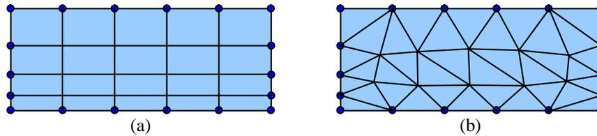
There are  $5 \times 4 = 20$  cells in the structured grid, and there are 36 cells in the unstructured grid.
