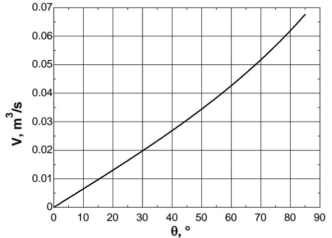
**Discussion** Note that a general flow rate equation for the V-notch would be in the form of  $\dot{V} = K \tan(\theta/2) H^{5/2}$ , where  $K = C_d 8\sqrt{2g}/15$  and  $C_d$  is the discharge coefficient whose value is determined experimentally to account for nonideal effects.
