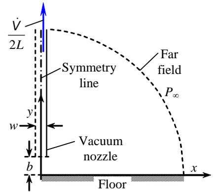
**FIGURE 1** CFD model of air being sucked into a vertical vacuum nozzle; the  $y$ -axis is a line of symmetry (not to scale – the far field is actually much further away from the nozzle than is sketched here).
