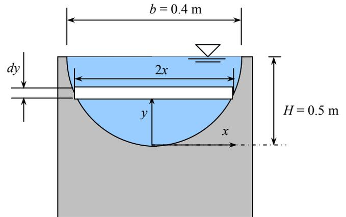
Noting that the flow velocity is  $V = \sqrt{2g(H-y)}$ , the flow rate through this differential area is
