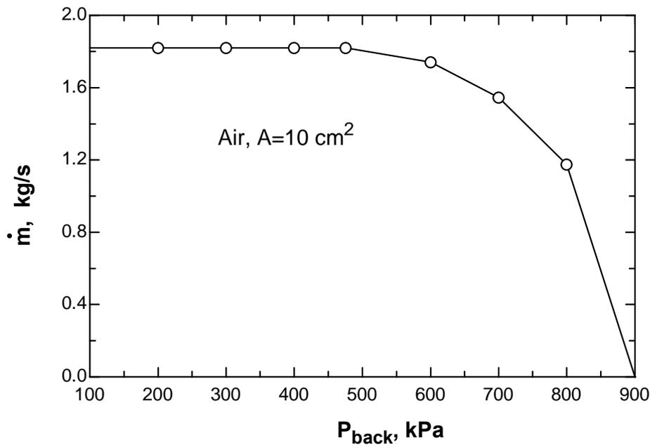
**Discussion** We see from the plot that once the flow is choked at a back pressure of 475.5 kPa, the mass flow rate remains constant regardless of how low the back pressure gets.
