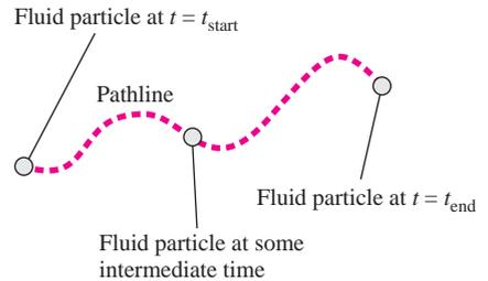
A *pathline* is formed by following the actual path of a fluid particle.
