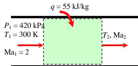
The exit stagnation temperature is, from the energy equation  $q = c_p(T_{02} - T_{01})$ ,
