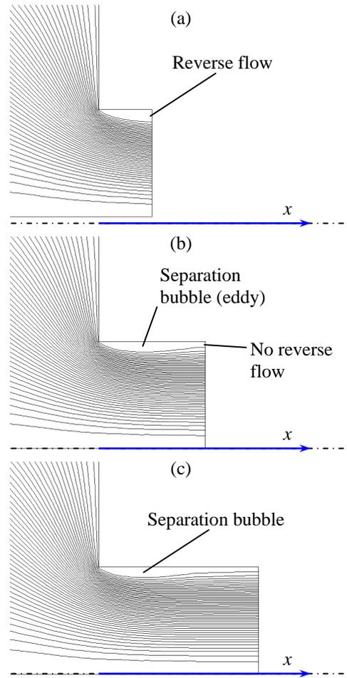
**FIGURE 1** Streamlines:  $L_{extend}/D_2 =$  (a) 0.25, (b) 0.50, and (c) 0.75.
