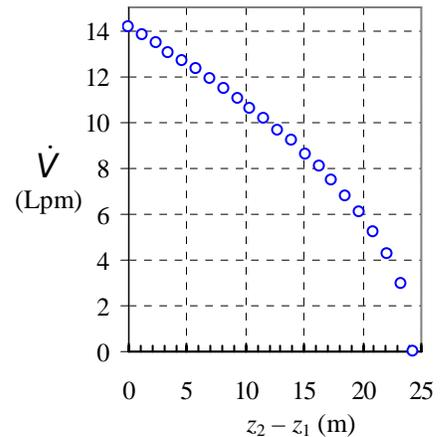
**Discussion** You may wish to think of the backward-flow through the pump as a case in which the pump efficiency is *negative*. In fact, at  $(z_2 - z_1) = H_0$ , the pump could be replaced by a closed valve to keep the water from draining from the upper reservoir to the lower reservoir.
