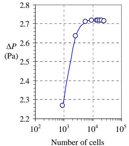
**FIGURE 2** Pressure difference vs. number of cells.
