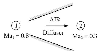
For an adiabatic diffuser, the energy equation reduces to  $h_{01} = h_{02}$ . Noting that  $h = c_p T$  and the specific heats are assumed to be constant, we have
