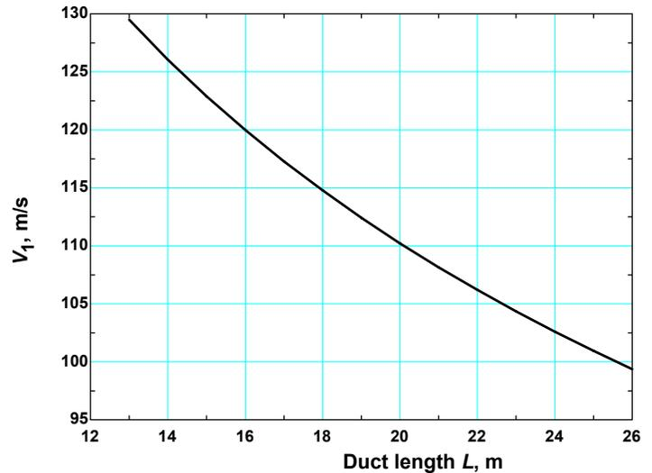
**Discussion** Note that once the flow is choked, any increase in duct length results in a decrease in the mass flow rate and the inlet velocity.
