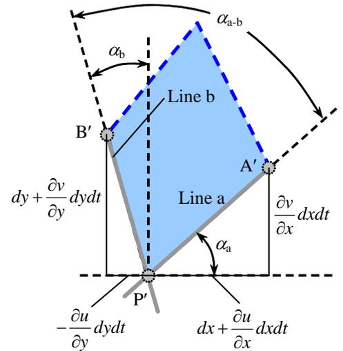
**FIGURE 1** A close-up view of the distorted fluid element at time  $t_2$ .
