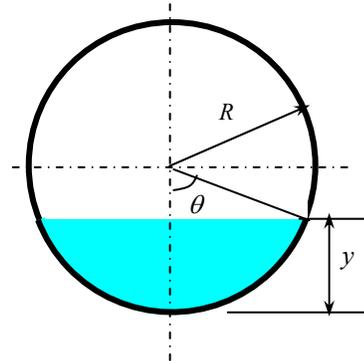
**Discussion** The depth-to-radius ratio of  $y/R = 1$  corresponds to a half-full circular channel, and it is clear from the table and the chart that, for a fixed flow area, the flow rate becomes maximum when the channel is half-full.
