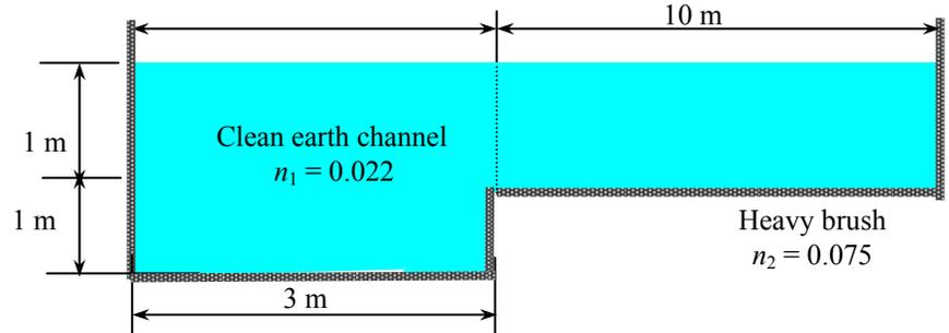
The flow area, perimeter, and hydraulic radius for each subsection and the entire channel are:
