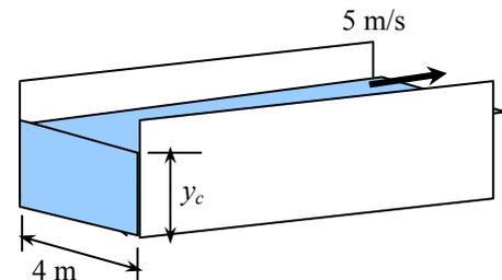
**Discussion** Critical flow is not a stable type of flow and can be observed for short intervals. Occurrence of critical depth is important as boundary condition most of the time. For example it can be used as a flow rate computation mechanism for a channel ending with a drawdown.
