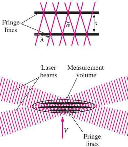
**FIGURE 8-75** Fringes that form as a result of the interference at the intersection of two laser beams of an LDV system (lines represent peaks of waves). The top diagram is a close-up view of two fringes.
