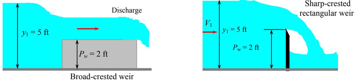
**Assumptions** 1 The flow is steady. 2 The upstream velocity head is negligible. 3 The channel is sufficiently wide so that the end effects are negligible.
