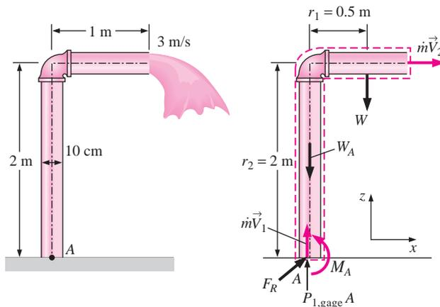
**FIGURE 6-37** Schematic for Example 6-8 and the free-body diagram.
