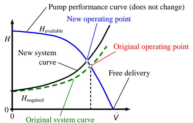
**Discussion** The shift of operating point to lower  $\dot{V}$  agrees with our physical intuition. Namely, as we close the valve somewhat, the pump has to do more work to overcome the losses, and we expect the flow rate to decrease accordingly.
