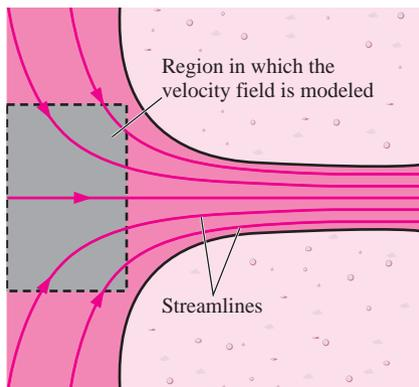
**FIGURE 4-5** Flow field near the bell mouth inlet of a hydroelectric dam; a portion of the velocity field of Example 4-1 may be used as a first-order approximation of this physical flow field. The shaded region corresponds to that of Fig. 4-4.
