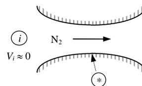
Critical properties are those at a location where the Mach number is  $Ma = 1$ . From Table A-13 at  $Ma = 1$ , we read  $T/T_0 = 0.8333$ ,  $P/P_0 = 0.5283$ , and  $\rho/\rho_0 = 0.6339$ . Then the critical properties become
