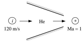
The Mach number at the nozzle exit is given to be  $Ma = 1$ . Therefore, the properties at the nozzle exit are the *critical properties* determined from
