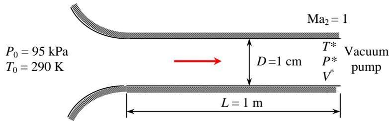
**Assumptions** 1 The assumptions associated with Fanno flow (i.e., steady, frictional flow of an ideal gas with constant properties through a constant cross-sectional area adiabatic duct) are valid. 2 The friction factor is constant along the duct.
