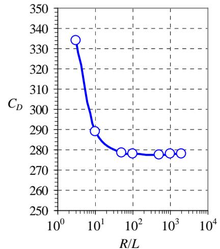
**Discussion** When analyzing creeping flow using CFD, it is important to extend the computational domain very far from the object of interest, since viscous effects influence the flow very far from the object. This effect is not as great at high Reynolds numbers, where the inertial terms dominate the viscous terms.
