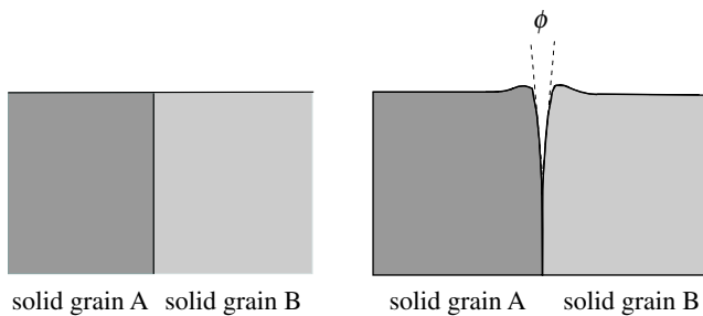
Figure 6.12 Grain boundary after polishing (a) and after the subsequent thermal etching (b).
