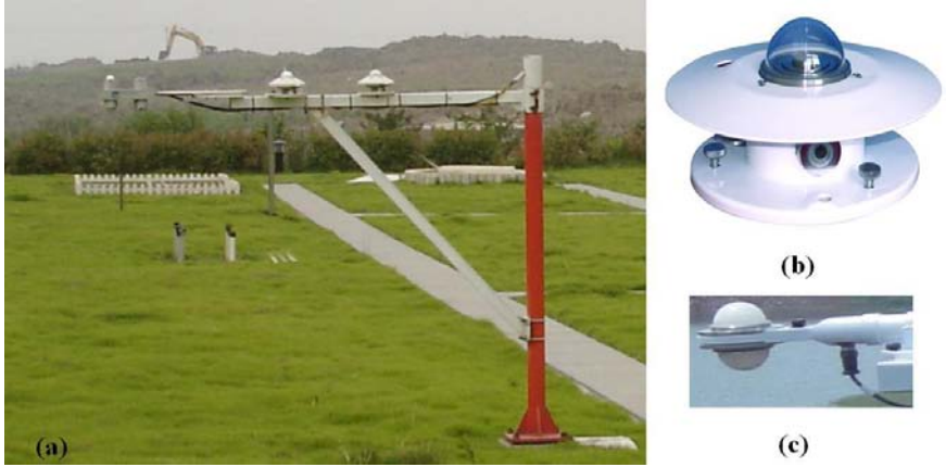
FIG. 2. Pyranometers: (a) field installation, (b) a pyranometer to measure total radiation, (c) a net pyranometer.
