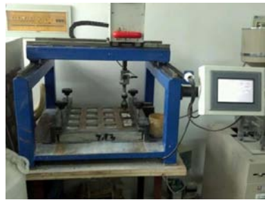
FIG. 7 Pull-off Bond Strength Measurement
