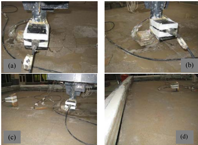
FIG. 5. Snapshots of the model during Test Stage 3 of this experiment: (a) crack formed near soil-pile interface, (b) gap formed between soil and pile, and water spilled out, (c) pile head tilted after a few cycles, and (d) lateral displacement of frozen crust observed.
