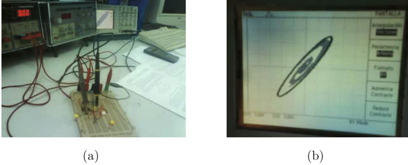
Figure 1.11: (a) A Wien bridge circuit built on a protoboard. (b) Experimental observation on an oscilloscope of the limit cycle, for the real value R_F = 10.63 \text{ K}\Omega .
