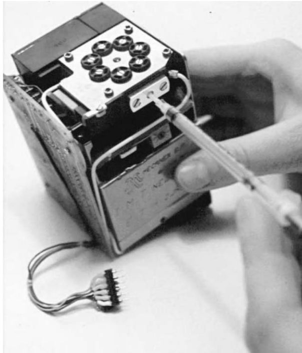
Figure 4-11. Space bioreactor developed in collaboration by the ETH Zurich, Mecanex, Nyon and the University of Neuchâtel. Photo courtesy of Isabelle Walther.
