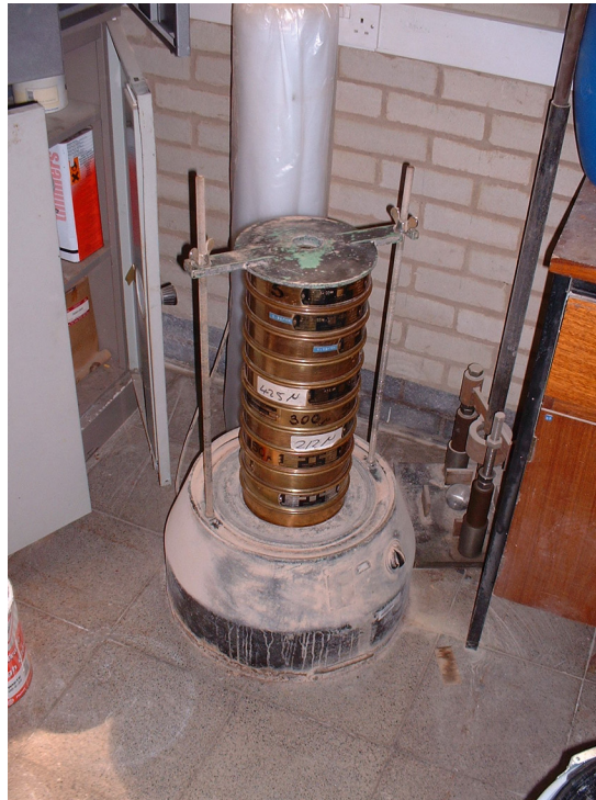
FIGURE 19.2 Sieves Stacked in Sieve Shaker
