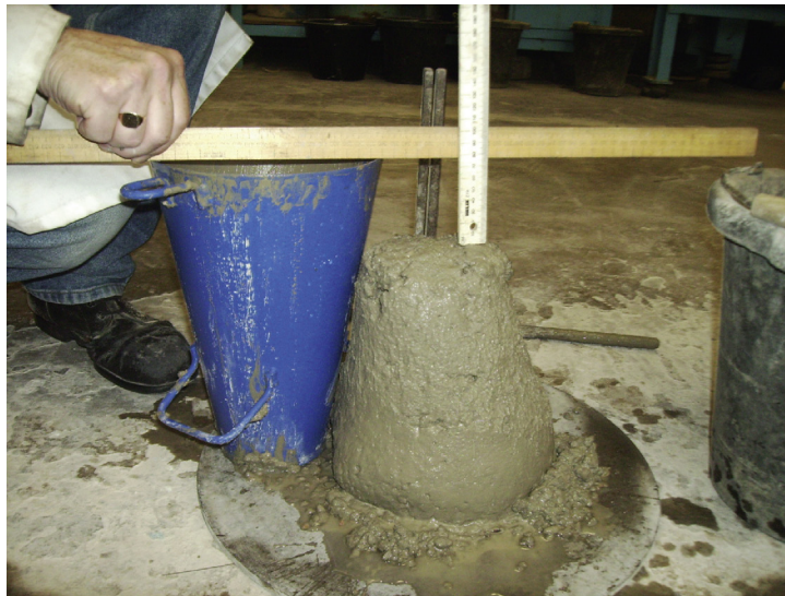
FIGURE 22.2 The Slump Test
