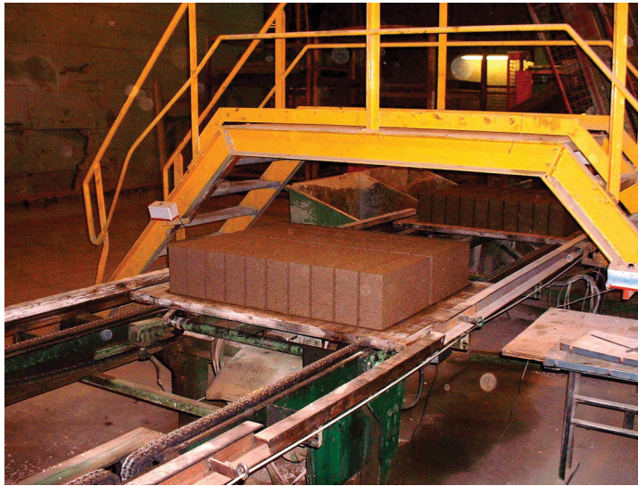
FIGURE 34.6 Production of Aggregate Concrete Blocks
