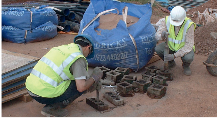
FIGURE 22.11 Compacting Test Cubes on Site
