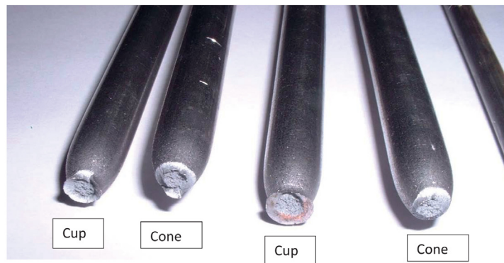
FIGURE 3.6 Steel Samples After Failure
