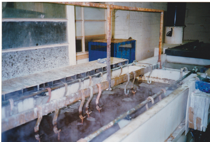
FIGURE 32.5 A Small Scale Electroplating Tank
