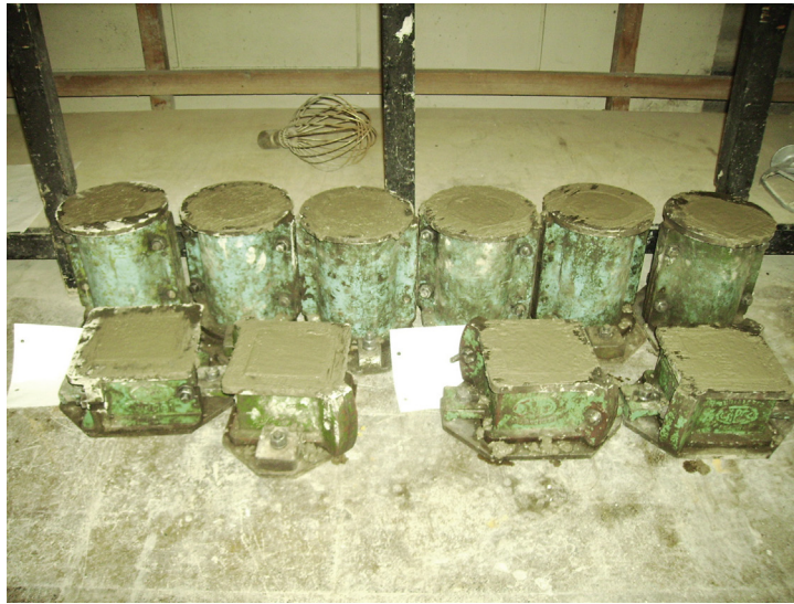
FIGURE 22.12 Filled Cube and Cylinder Moulds
