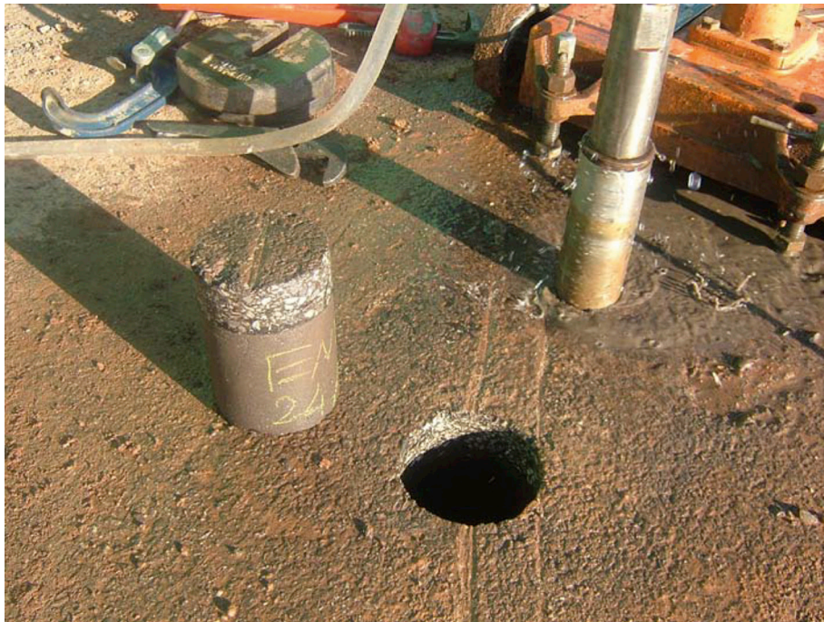
FIGURE 27.7 Core Recovered From Road Slab
