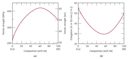
**FIGURE 10.5** For the copper–nickel system, (a) tensile strength versus composition, and (b) ductility (%EL) versus composition at room temperature. A solid solution exists over all compositions for this system.
