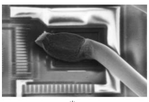
**FIGURE 20.24** Scanning electron micrographs of (a) a ball bond  $(475\times)$ , and (b) a wedge bond  $(275\times)$ . (Photographs courtesy of National Semiconductor Corporation.)
