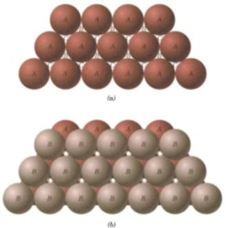
FIGURE 3.27 (a) A portion of a close-packed plane of atoms; A, B, and Cpositions are indicated. (b) The AB stacking sequence for close-packed atomic planes. (Adapted from W. G. Moffatt, G. W. Pearsall, and J. Wulff, The Structure and Properties of Materials, Vol. I, Structure, p. 50. Copyright © 1964 by John Wiley & Sons, New York. Reprinted by permission of John Wiley & Sons, Inc.)
