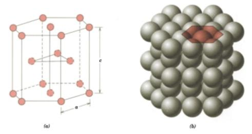
**FIGURE 3.3** For the hexagonal close-packed crystal structure, (a) a reduced-sphere unit cell (a and c represent the short and long edge lengths, respectively), and (b) an aggregate of many atoms. (Figure (b) from W. G. Moffatt, G. W. Pearsall, and J. Wulff, *The Structure and Properties of Materials,* Vol. I, *Structure,* p. 51. Copyright © 1964 by John Wiley & Sons, New York. Reprinted by permission of John Wiley & Sons, Inc.)
