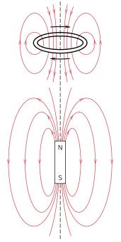
**FIGURE 18.1** Magnetic field lines of force around a current loop and a bar magnet.
