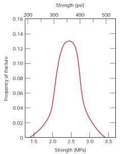
FIGURE 9.16 The frequency distribution of observed fracture strengths for a portland cement. (From W. Weibull, *Ing. Vetensk. Akad.*, Proc. 151, No. 153, 1939.)
