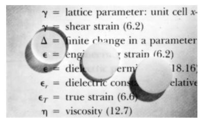
FIGURE 19.10 Photograph showing the light transmittance of three aluminum oxide specimens. From left to right: single-crystal material (sapphire), which is transparent; a polycrystalline and fully dense (nonporous) material, which is translucent; and a polycrystalline material that contains approximately 5% porosity, which is opaque. (Specimen preparation, P. A. Lessing; photography by J. Telford.)
