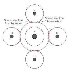
FIGURE 2.10 Schematic representation of covalent bonding in a molecule of methane (CH<sub>4</sub>).
