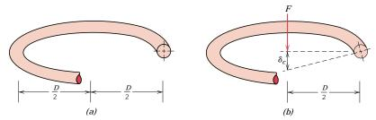
**FIGURE 20.5** Schematic diagrams of one coil of a helical spring, (a) prior to being compressed, and (b) showing the deflection  $\delta_c$  produced from the compressive force F. (Adapted from K. Edwards and P. McKee, *Fundamentals of Mechanical Component Design*. Copyright © 1991 by McGraw-Hill, Inc. Reproduced with permission of The McGraw-Hill Companies.)
