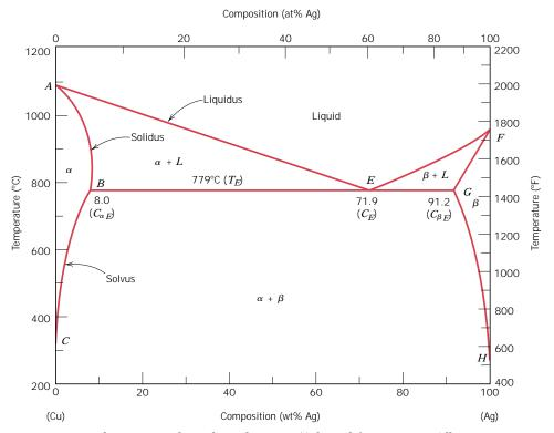
**FIGURE 10.6** The copper-silver phase diagram. (Adapted from *Binary Alloy Phase Diagrams, 2nd edition, Vol. 1, T. B. Massalski, Editor-in-Chief, 1990. Reprinted by permission of ASM International, Materials Park, OH.)*
