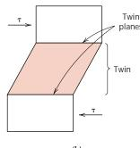
**FIGURE 8.13** For a single crystal subjected to a shear stress  $\tau$ , (a) deformation by slip; (b) deformation by twinning.
