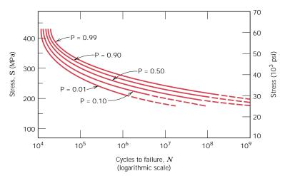
fatigue failure. High-cycle fatigue is associated with fatigue lives greater than about  $10^4$  to  $10^5$  cycles.
