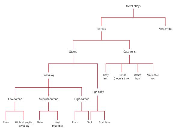
FIGURE 13.1 Classification scheme for the various ferrous alloys.
