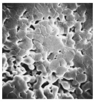
FIGURE 14.25 Scanning electron micrograph of an aluminum oxide powder compact that was sintered at 1700°C for 6 min. 5000×. (From W. D. Kingery, H. K. Bowen, and D. R. Uhlmann, *Introduction to Ceramics*, 2nd edition, p. 483. Copyright © 1976 by John Wiley & Sons, New York. Reprinted by permission of John Wiley & Sons, Inc.)
