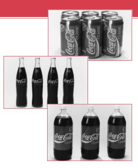
A familiar item that is fabricated from three different material types is the beverage container. Beverages are marketed in aluminum (metal) cans (top), glass (ceramic) bottles (center), and plastic (polymer) bottles (bottom). (Permission to use these photographs was granted by the Coca-Cola Company.)
