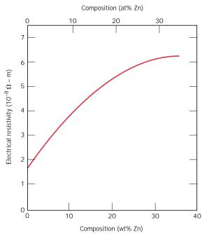
FIGURE 12.35 Room-temperature electrical resistivity versus composition for copper-zinc alloys. (Adapted from *Metals Handbook: Properties and Selection: Nonferrous Alloys and Pure Metals*, Vol. 2, 9th edition, H. Baker, Managing Editor, American Society for Metals, 1979, p. 315.)
