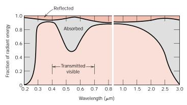
FIGURE 19.8 The variation with wavelength of the fractions of incident light transmitted, absorbed, and reflected through a green glass. (From W. D. Kingery, H. K. Bowen, and D. R. Uhlmann, *Introduction to Ceramics*, 2nd edition. Copyright © 1976 by John Wiley & Sons, New York. Reprinted by permission of John Wiley & Sons, Inc.)
