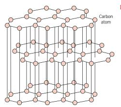
**FIGURE 3.17** The structure of graphite.
