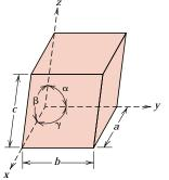
**FIGURE 3.19** A unit cell with x, y, and z coordinate axes, showing axial lengths (a, b, and c) and interaxial angles ( $\alpha$ ,  $\beta$ , and  $\gamma$ ).
