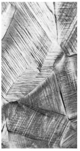
FIGURE 8.10 Slip lines on the surface of a polycrystalline specimen of copper that was polished and subsequently deformed. 173×. (Photomicrograph courtesy of C. Brady, National Bureau of Standards.)
