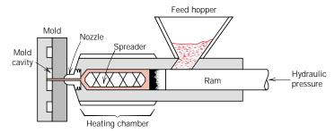
**FIGURE 14.28** Schematic diagram of an injection molding apparatus. (Adapted from F. W. Billmeyer, Jr., *Textbook of Polymer Science,* 2nd edition. Copyright © 1971 by John Wiley & Sons, New York. Reprinted by permission of John Wiley & Sons, Inc.)
