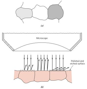
**FIGURE 5.15** (a) Polished and etched grains as they might appear when viewed with an optical microscope. (b) Section taken through these grains showing how the etching characteristics and resulting surface texture vary from grain to grain because of differences in crystallographic orientation. (c) Photomicrograph of a polycrystalline brass specimen.  $60\times$ . (Photomicrograph courtesy of J. E. Burke, General Electric Co.)
