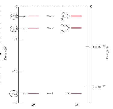
These states do not vary continuously with energy; that is, adjacent states are separated by finite energies. For example, allowed states for the Bohr hydrogen atom are represented in Figure 2.2a. These energies are taken to be negative, whereas the zero reference is the unbound or free electron. Of course, the single electron associated with the hydrogen atom will fill only one of these states.
