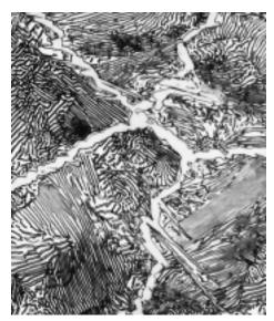
FIGURE 10.35 Photomicrograph of a 1.4 wt% C steel having a microstructure consisting of a white proeutectoid cementite network surrounding the pearlite colonies. 1000×. (Copyright 1971 by United States Steel Corporation.)
