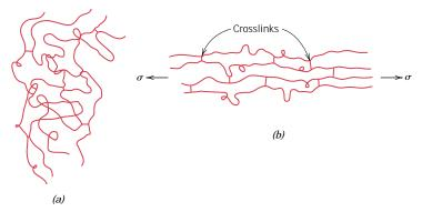
**FIGURE 8.29** Schematic representation of crosslinked polymer chain molecules (a) in an unstressed state and (b) during elastic deformation in response to an applied tensile stress. (Adapted from Z. D. Jastrzebski, *The Nature and Properties of Engineering Materials*, 3rd edition. Copyright © 1987 by John Wiley & Sons, New York. Reprinted by permission of John Wiley & Sons, Inc.)
