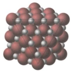
FIGURE 3.31 A section of the rock salt crystal structure from which a corner has been removed. The exposed plane of anions (light spheres inside the triangle) is a {111}-type plane; the cations (dark spheres) occupy the interstitial octahedral positions.
