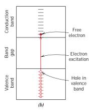
moted across the energy band gap and into empty states at the bottom of the conduction band. This is possible only by supplying to an electron the difference in energy between these two states, which is approximately equal to the band gap energy  $E_g$ . This excitation process is demonstrated in Figure 12.6. For many materials this band gap is several electron volts wide. Most often the excitation energy is from a nonelectrical source such as heat or light, usually the former.
