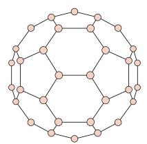
**FIGURE 3.18** The structure of a  $C_{60}$  molecule.
