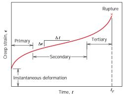
**FIGURE 9.40** Typical creep curve of strain versus time at constant stress and constant elevated temperature. The minimum creep rate  $\Delta\epsilon/\Delta t$  is the slope of the linear segment in the secondary region. Rupture lifetime  $t_r$  is the total time to rupture.
