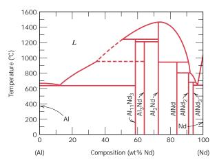
FIGURE 10.39 The aluminum-neodymium phase diagram. (Adapted from *ASM Handbook*, Vol. 3, *Alloy Phase Diagrams*, H. Baker, Editor, 1992. Reprinted by permission of ASM International, Materials Park, OH.)
