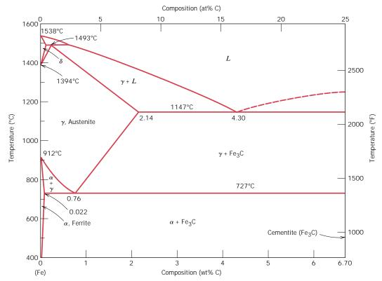
**FIGURE 10.26** The iron–iron carbide phase diagram. (Adapted from *Binary Alloy Phase Diagrams, 2nd edition, Vol. 1, T. B. Massalski, Editor-in-Chief, 1990. Reprinted by permission of ASM International, Materials Park, OH.)*
