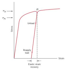
FIGURE 7.17 Schematic tensile stress-strain diagram showing the phenomena of elastic strain recovery and strain hardening. The initial yield strength is designated as  $\sigma_{y_0}$ ;  $\sigma_{y_i}$  is the yield strength after releasing the load at point D, and then upon reloading.
