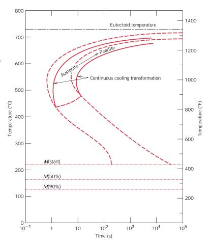
of rates over which both pearlite and martensite are produced. Finally, a totally pearlitic structure develops for low cooling rates.
