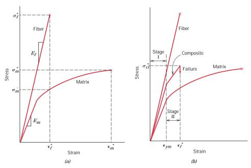
**FIGURE 15.9** (a) Schematic stress-strain curves for brittle fiber and ductile matrix materials. Fracture stresses and strains for both materials are noted. (b) Schematic stress-strain curve for an aligned fiber-reinforced composite that is exposed to a uniaxial stress applied in the direction of alignment; curves for the fiber and matrix materials shown in part (a) are also superimposed.
