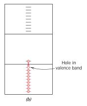
termed *p-type* because positively charged particles are primarily responsible for electrical conduction. Of course, holes are the majority carriers, and electrons are present in minority concentrations. This gives rise to a predominance of the second term on the right-hand side of Equation 12.13, or
