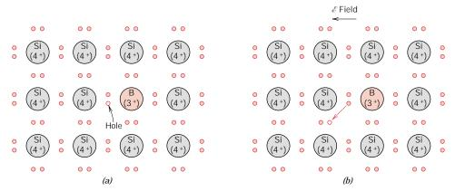
**FIGURE 12.13** Extrinsic *p*-type semiconduction model (electron bonding). (a) An impurity atom such as boron, having three valence electrons, may substitute for a silicon atom. This results in a deficiency of one valence electron, or a hole associated with the impurity atom. (b) The motion of this hole in response to an electric field.
