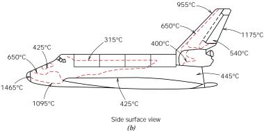
Table 20.5 Thermal Protection Systems Employed on the Space Shuttle Orbiter
