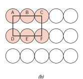
FIGURE 3.24 (a) Reducedsphere FCC unit cell with (110) plane. (b) Atomic packing of an FCC (110) plane. Corresponding atom positions from (a) are indicated.
