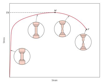
applied, often a structure has experienced so much plastic deformation that it is useless. Furthermore, fracture strengths are not normally specified for engineering design purposes.
