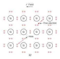
Thus, in the presence of an electric field, excited electrons and holes move in opposite directions. Furthermore, in semiconductors both electrons and holes are scattered by lattice imperfections.
