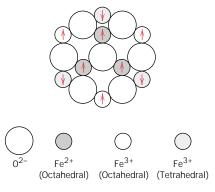
FIGURE 18.9 Schematic diagram showing the spin magnetic moment configuration for Fe<sup>2+</sup> and Fe3+ ions in Fe3O4. (From Richard A. Flinn and Paul K. Trojan, Engineering Materials and Their Applications, 4th edition. Copyright © 1990 by John Wiley & Sons, Inc. Adapted by permission of John Wiley & Sons, Inc.)
