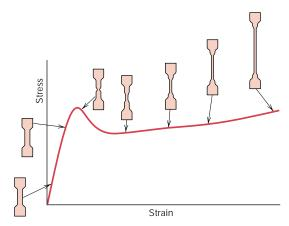
FIGURE 7.25 Schematic tensile stress-strain curve for a semicrystalline polymer. Specimen contours at several stages of deformation are included. (From Jerold M. Schultz, *Polymer Materials Science*, copyright © 1974, p. 488. Reprinted by permission of Prentice-Hall, Inc., Englewood Cliffs, NJ.)
