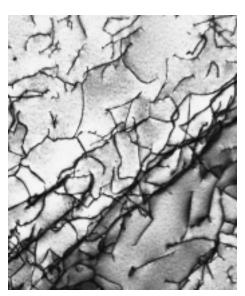
FIGURE 5.10 A transmission electron micrograph of a titanium alloy in which the dark lines are dislocations. 51,450×. (Courtesy of M. R. Plichta, Michigan Technological University.)
