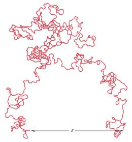
FIGURE 4.6 Schematic representation of a single polymer chain molecule that has numerous random kinks and coils produced by chain bond rotations. (From L. R. G. Treloar, *The Physics of Rubber Elasticity*, 2nd edition, Oxford University Press, Oxford, 1958, p. 47.)
