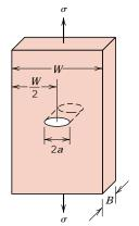
**FIGURE 9.12** Schematic representation of a flat plate of finite width having a through-thickness center crack.
