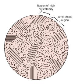
FIGURE 4.11 Fringed-micelle model of a semicrystalline polymer, showing both crystalline and amorphous regions. (From H. W. Hayden, W. G. Moffatt, and J. Wulff, *The Structure and Properties of Materials*, Vol. III, *Mechanical Behavior*. Copyright © 1965 by John Wiley & Sons, New York. Reprinted by permission of John Wiley & Sons, Inc.)
