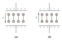
FIGURE 12.31 Dipole orientations for (a) one polarity of an alternating electric field and (b) for the reversed polarity. (From Richard A. Flinn and Paul K. Trojan, *Engineering Materials and Their Applications*, 4th edition. Copyright © 1990 by John Wiley & Sons, Inc. Adapted by permission of John Wiley & Sons, Inc.)
