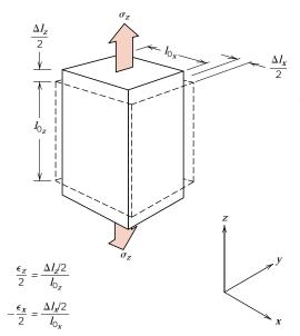
FIGURE 7.9 Axial (z) elongation (positive strain) and lateral (x and y) contractions (negative strains) in response to an imposed tensile stress. Solid lines represent dimensions after stress application; dashed lines, before.
