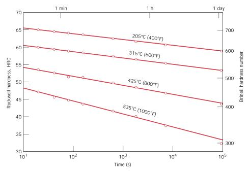
**FIGURE 11.27** Hardness versus tempering time for a water-quenched eutectoid plain carbon (1080) steel. (Adapted from Edgar C. Bain, *Functions of the Alloying Elements in Steel*, American Society for Metals, 1939, p. 233.)
