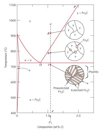
FIGURE 10.34 Schematic representations of the microstructures for an iron–carbon alloy of hypereutectoid composition  $C_1$  (containing between 0.76 and 2.14 wt% C), as it is cooled from within the austenite phase region to below the eutectoid temperature.
