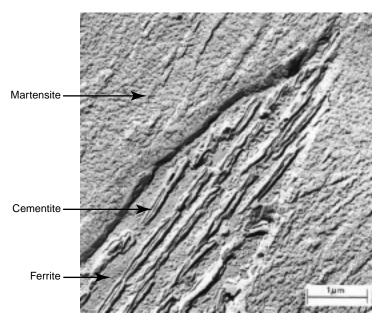
**FIGURE 11.8** Replica transmission electron micrograph showing the structure of bainite. A grain of bainite passes from lower left to upper right-hand corners, which consists of elongated and needle-shaped particles of Fe<sub>3</sub>C within a ferrite matrix. The phase surrounding the bainite is martensite. (Reproduced with permission from *Metals Handbook*, Vol. 8, 8th edition, *Metallography, Structures and Phase Diagrams,* American Society for Metals, Materials Park, OH, 1973.)
