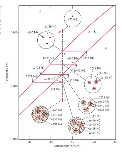
Let us begin cooling from a temperature of about 1300°C; this is indicated by point a' in the liquid region. This liquid has a composition of 35 wt% Ni–65 wt% Cu [noted as L(35 Ni) in the figure], and no changes occur while cooling through the liquid phase region (moving down vertically from point a'). At point b' (approximately 1260°C),  $\alpha$  phase particles begin to form, which, from the tie line constructed, have a composition of 46 wt% Ni–54 wt% Cu [ $\alpha(46 \text{ Ni})$ ].
