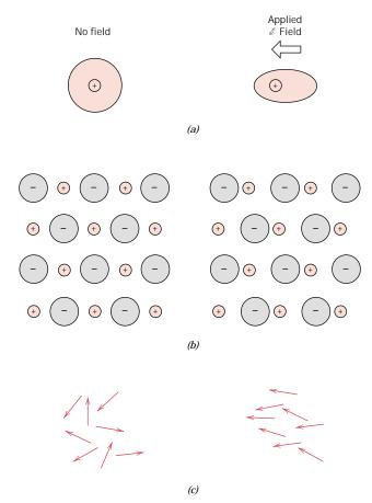
FIGURE 12.30 (a) Electronic polarization that results from the distortion of an atomic electron cloud by an electric field. (b) Ionic polarization that results from the relative displacement of electrically charged ions in response to an electric field. (c) Response of permanent electric dipoles (arrows) to an applied electric field, producing orientation polarization. (From O. H. Wyatt and D. Dew-Hughes, Metals, Ceramics and Polymers, Cambridge University Press, 1974.)
