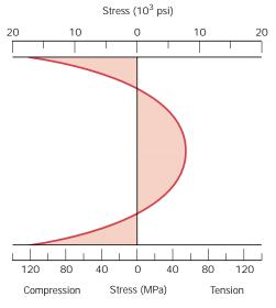
FIGURE 14.19 Room-temperature residual stress distribution over the cross section of a tempered glass plate. (From W. D. Kingery, H. K. Bowen, and D. R. Uhlmann, *Introduction to Ceramics*, 2nd edition. Copyright © 1976 by John Wiley & Sons, New York. Reprinted by permission of John Wiley & Sons, Inc.)
