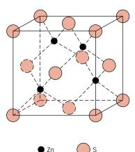
**FIGURE 3.7** A unit cell for the zinc blende (ZnS) crystal structure.
