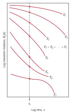
FIGURE 7.27 Schematic plot of logarithm of relaxation modulus versus logarithm of time for a viscoelastic polymer; isothermal curves are generated at temperatures  $T_1$  through  $T_7$ . The temperature dependence of the relaxation modulus is represented as  $\log E_r(t_1)$  versus temperature.
