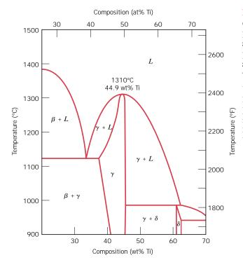
FIGURE 10.20 A portion of the nickel-titanium phase diagram on which is shown a congruent melting point for the  $\gamma$  phase solid solution at 1310°C and 44.9 wt% Ti. (Adapted from *Phase Diagrams of Binary Nickel Alloys*, P. Nash, Editor, 1991. Reprinted by permission of ASM International, Materials Park, OH.)
