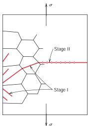
**FIGURE 9.28** Schematic representation showing stages I and II of fatigue crack propagation in polycrystalline metals. (Copyright ASTM. Reprinted with permission.)
