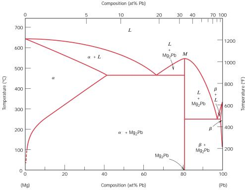
**FIGURE 10.18** The magnesium-lead phase diagram. (Adapted from *Phase Diagrams of Binary Magnesium Alloys*, A. A. Nayeb-Hashemi and J. B. Clark, Editors, 1988. Reprinted by permission of ASM International, Materials Park, OH.)
