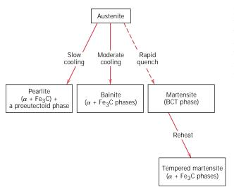
FIGURE 11.28 Possible transformations involving the decomposition of austenite. Solid arrows, transformations involving diffusion; dashed arrow, diffusionless transformation.
