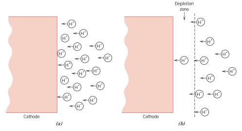
**FIGURE 16.8** For hydrogen reduction, schematic representations of the H<sup>+</sup> distribution in the vicinity of the cathode for (a) low reaction rates and/or high concentrations, and (b) high reaction rates and/or low concentrations wherein a depletion zone is formed that gives rise to concentration polarization. (Adapted from M. G. Fontana, *Corrosion Engineering*, 3rd edition. Copyright © 1986 by McGraw-Hill Book Company. Reproduced with permission.)
