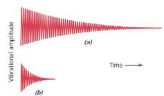
FIGURE 13.4 Comparison of the relative vibrational damping capacities of (a) steel and (b) gray cast iron. (From *Metals Engineering Quarterly*, February 1961. Copyright 1961 American Society for Metals.)
