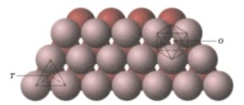
FIGURE 3.30 The stacking of one plane of close-packed spheres (anions) on top of another; tetrahedral and octahedral positions between the planes are designated by *T* and *O*, respectively. (From W. G. Moffatt, G. W. Pearsall, and J. Wulff, *The Structure and Properties of Materials*, Vol. 1, *Structure*. Copyright © 1964 by John Wiley & Sons, New York. Reprinted by permission of John Wiley & Sons, Inc.)
