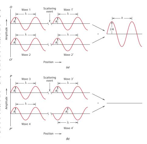
beam of x-rays impinges on a solid material, a portion of this beam will be scattered in all directions by the electrons associated with each atom or ion that lies within the beam's path. Let us now examine the necessary conditions for diffraction of x-rays by a periodic arrangement of atoms.
