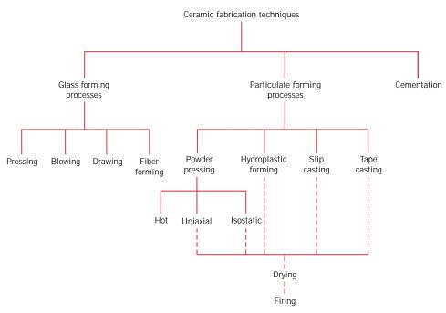
**FIGURE 14.14** A classification scheme for the ceramic-forming techniques discussed in this chapter.
