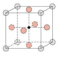
**FIGURE 3.9** A unit cell for the perovskite crystal structure.
