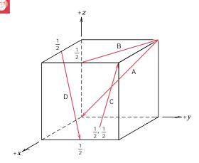
**3.53** Determine the indices for the directions shown in the following cubic unit cell:
