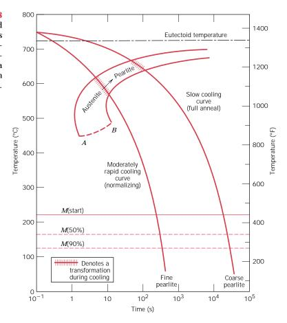
In summary, isothermal and continuous transformation diagrams are, in a sense, phase diagrams in which the parameter of time is introduced. Each is experimentally determined for an alloy of specified composition, the variables being temperature and time. These diagrams allow prediction of the microstructure after some time period for constant temperature and continuous cooling heat treatments, respectively.
