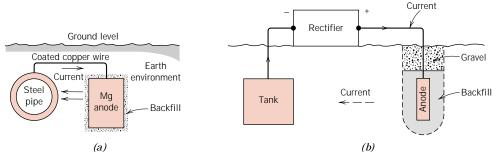
**FIGURE 16.22** Cathodic protection of (a) an underground pipeline using a magnesium sacrificial anode, and (b) an underground tank using an impressed current. (From M. G. Fontana, *Corrosion Engineering*, 3rd edition. Copyright © 1986 by McGraw-Hill Book Company. Reproduced with permission.)
