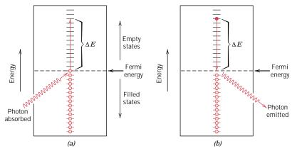
**FIGURE 19.4** (a) Schematic representation of the mechanism of photon absorption for metallic materials in which an electron is excited into a higher-energy unoccupied state. The change in energy of the electron  $\Delta E$  is equal to the energy of the photon. (b) Reemission of a photon of light by the direct transition of an electron from a high to a low energy state.
