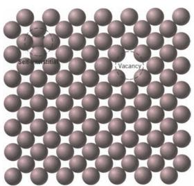
FIGURE 5.1 Two-dimensional representations of a vacancy and a self-interstitial. (Adapted from W. G. Moffatt, G. W. Pearsall, and J. Wulff, *The Structure and Properties of Materials*, Vol. I, *Structure*, p. 77. Copyright © 1964 by John Wiley & Sons, New York. Reprinted by permission of John Wiley & Sons, Inc.)
