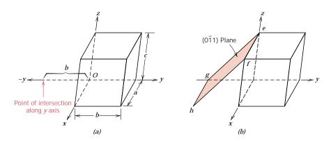
the top face of the unit cell; also, line gh represents the intersection between this same ( $0\overline{1}1$ ) plane and the plane of the bottom unit cell face extended. Similarly, lines eg and fh are the intersections between ( $0\overline{1}1$ ) and back and front cell faces, respectively.
