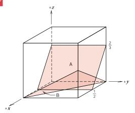
**3.59** Sketch the  $(1\overline{1}01)$  and  $(11\overline{2}0)$  planes in a hexagonal unit cell.
