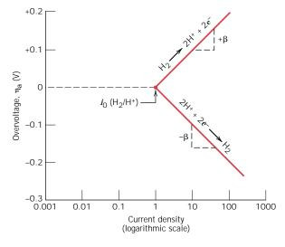
FIGURE 16.7 For a hydrogen electrode, plot of activation polarization overvoltage versus logarithm of current density for both oxidation and reduction reactions. (Adapted from M. G. Fontana, *Corrosion Engineering*, 3rd edition. Copyright © 1986 by McGraw-Hill Book Company. Reproduced with permission.)
