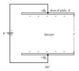
FIGURE 12.29 Schematic representations of (a) the charge stored on capacitor plates for a vacuum, (b) the dipole arrangement in an unpolarized dielectric, and (c) the increased charge storing capacity resulting from the polarization of a dielectric material. (Adapted from A. G. Guy, Essentials of Materials Science, McGraw-Hill Book Company, New York, 1976.)
