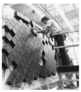
FIGURE 20.17 Photograph showing the installation of thermal protection ceramic tiles on the Space Shuttle Orbiter. [Photograph courtesy the National Aeronautics and Space Administration (NASA).]
