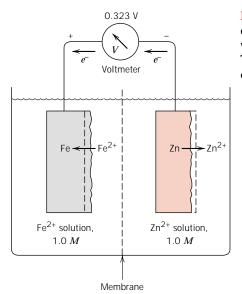
**FIGURE 16.3** An electrochemical cell consisting of iron and zinc electrodes, each of which is immersed in a 1M solution of its ion. The iron electrodeposits while the zinc corrodes.
