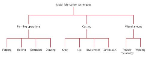
**FIGURE 14.1** Classification scheme of metal fabrication techniques discussed in this chapter.
