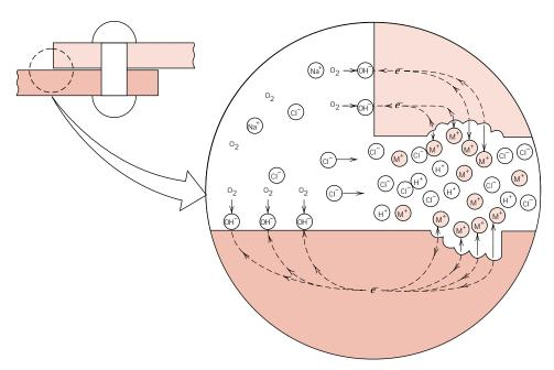
FIGURE 16.16 Schematic illustration of the mechanism of crevice corrosion between two riveted sheets. (From M. G. Fontana, *Corrosion Engineering*, 3rd edition. Copyright © 1986 by McGraw-Hill Book Company. Reproduced with permission.)
