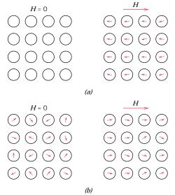
FIGURE 18.5 (a) The atomic dipole configuration for a diamagnetic material with and without a magnetic field. In the absence of an external field, no dipoles exist; in the presence of a field, dipoles are induced that are aligned opposite to the field direction. (b) Atomic dipole configuration with and without an external magnetic field for a paramagnetic material.
