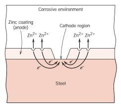
**FIGURE 16.23** Galvanic protection of steel as provided by a coating of zinc.
