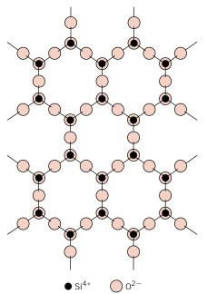
**FIGURE 3.13** Schematic representation of the two-dimensional silicate sheet structure having a repeat unit formula of  $(Si_2O_5)^{2-}$ .
