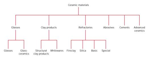
FIGURE 13.6 Classification of ceramic materials on the basis of application.
