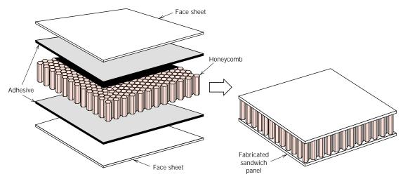
**FIGURE 15.17** Schematic diagram showing the construction of a honeycomb core sandwich panel. (Reprinted with permission from *Engineered Materials Handbook*, Vol. 1, *Composites*, ASM International, Metals Park, OH, 1987.)
