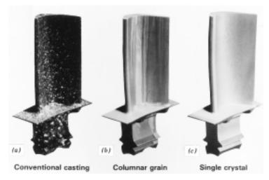
**FIGURE 9.45** (a) Polycrystalline turbine blade that was produced by a conventional casting technique. High-temperature creep resistance is improved as a result of an oriented columnar grain structure (b) produced by a sophisticated directional solidification technique. Creep resistance is further enhanced when single-crystal blades (c) are used. (Courtesy of Pratt & Whitney.)
