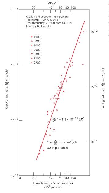
FIGURE 9.35 Logarithm crack growth rate versus logarithm stress intensity factor range for a Ni-Mo-V steel. (Reprinted by permission of the Society for Experimental Mechanics, Inc.)
