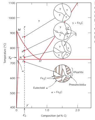
FIGURE 10.31 Schematic representations of the microstructures for an iron–carbon alloy of hypoeutectoid composition  $C_0$  (containing less than 0.76 wt% C) as it is cooled from within the austenite phase region to below the eutectoid temperature.
