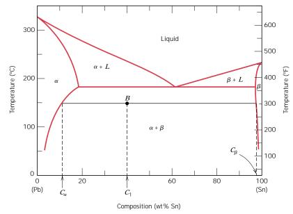
**FIGURE 10.8** The lead-tin phase diagram. For a 40 wt% Sn-60 wt% Pb alloy at  $150^{\circ}$ C (point B), phase compositions and relative amounts are computed in Example Problems 10.2 and 10.3.
