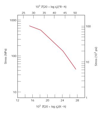
FIGURE 9.44 Logarithm stress versus the Larson-Miller parameter for an S-590 iron. (From F. R. Larson and J. Miller, *Trans. ASME*, 74, 765, 1952. Reprinted by permission of ASME.)
