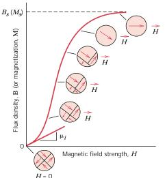
FIGURE 18.13 The *B*-versus-*H* behavior for a ferromagnetic or ferrimagnetic material that was initially unmagnetized. Domain configurations during several stages of magnetization are represented. Saturation flux density  $B_s$ , magnetization  $M_s$ , and initial permeability  $\mu_l$  are also indicated. (Adapted from O. H. Wyatt and D. Dew-Hughes, *Metals, Ceramics and Polymers,* Cambridge University Press, 1974.)
