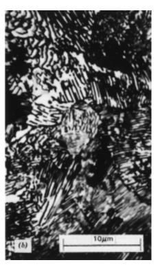
**FIGURE 11.6** Photomicrographs of (a) coarse pearlite and (b) fine pearlite. 3000×. (From K. M. Ralls, et al., *An Introduction to Materials Science and Engineering,* p. 361. Copyright © 1976 by John Wiley & Sons, New York. Reprinted by permission of John Wiley & Sons, Inc.)
