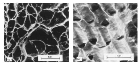
FIGURE 9.4 (a) Scanning electron fractograph showing spherical dimples characteristic of ductile fracture resulting from uniaxial tensile loads. 3300×. (b) Scanning electron fractograph showing parabolic-shaped dimples characteristic of ductile fracture resulting from shear loading. 5000×. (From R. W. Hertzberg, Deformation and Fracture Mechanics of Engineering Materials, 3rd edition. Copyright © 1989 by John Wiley & Sons, New York. Reprinted by permission of John Wiley & Sons, Inc.)
