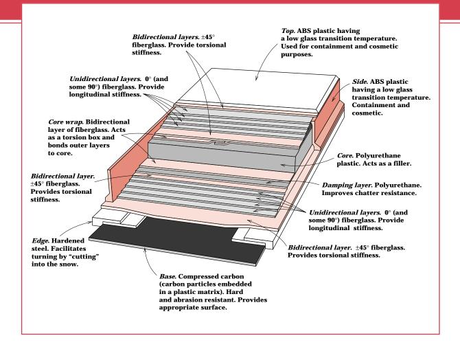
One relatively complex composite material is the modern ski. In this illustration, a cross-section of a high-performance snow ski, are shown the various components. The function of each component is noted, as well as the material that is used in its construction. (Courtesy of Evolution Ski Company, Salt Lake City, Utah.)
