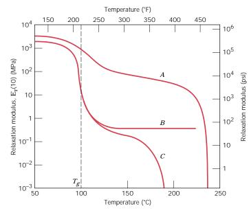
**FIGURE 7.29** Logarithm of the relaxation modulus versus temperature for crystalline isotactic (curve A), lightly crosslinked atactic (curve B), and amorphous (curve C) polystyrene. (From A. V. Tobolsky, Properties and Structures of Polymers. Copyright © 1960 by John Wiley & Sons, New York. Reprinted by permission of John Wiley & Sons, Inc.)
