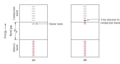
The extra nonbonding electron is loosely bound to the region around the impurity atom by a weak electrostatic attraction, as illustrated in Figure 12.11a. The binding energy of this electron is relatively small (on the order of 0.01 eV); thus, it is easily removed from the impurity atom, in which case it becomes a free or conducting electron (Figures 12.11b and 12.11c).
