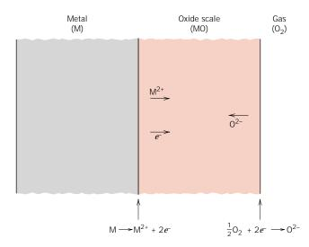
FIGURE 16.24 Schematic representation of processes that are involved in the gaseous oxidation at a metal surface.
