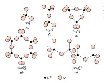
FIGURE 3.12 Five silicate ion structures formed from SiO<sub>4</sub><sup>4-</sup> tetrahedra.
