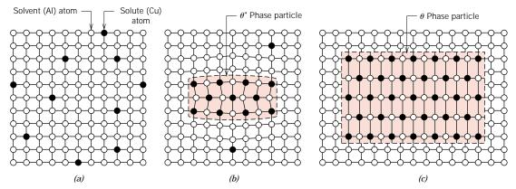
**FIGURE 11.33** Schematic depiction of several stages in the formation of the equilibrium precipitate  $(\theta)$  phase. (a) A supersaturated  $\alpha$  solid solution. (b) A transition,  $\theta''$ , precipitate phase. (c) The equilibrium  $\theta$  phase, within the  $\alpha$  matrix phase. Actual phase particle sizes are much larger than shown here.
