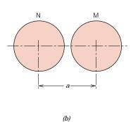
**FIGURE 3.26** (a) Reduced-sphere BCC unit cell with the [100] direction indicated. (b) Atomic spacing in the [100] direction for the BCC crystal structure—between atoms M and N in (a).
