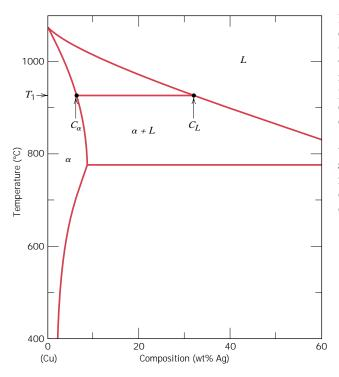
FIGURE 10.25 Enlarged copper-rich section of the Cu-Ag phase diagram in which the Gibbs phase rule for the coexistence of two phases (i.e.,  $\alpha$  and L) is demonstrated. Once the composition of either phase (i.e.,  $C_{\alpha}$  or  $C_{L}$ ) or the temperature (i.e.,  $T_{1}$ ) is specified, values for the two remaining parameters are established by construction of the appropriate tie line.
