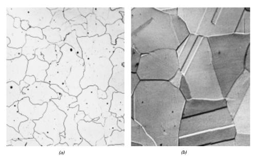
**FIGURE 10.27** Photomicrographs of (a)  $\alpha$  ferrite (90×) and (b) austenite (325×). (Copyright 1971 by United States Steel Corporation.)
