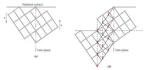
**FIGURE 8.12** Schematic diagram showing how twinning results from an applied shear stress  $\tau$ . In (b), open circles represent atoms that did not change position; dashed and solid circles represent original and final atom positions, respectively. (From G. E. Dieter, *Mechanical Metallurgy*, 3rd edition. Copyright © 1986 by McGraw-Hill Book Company, New York. Reproduced with permission of McGraw-Hill Book Company.)
