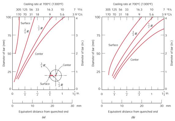
FIGURE 14.11 Cooling rate as a function of diameter at surface, three-quarters radius  $(\frac{3}{4}R)$ , midradius  $(\frac{1}{2}R)$ , and center positions for cylindrical bars quenched in mildly agitated (a) water and (b) oil. Equivalent Jominy positions are included along the bottom axis. (Adapted from *Metals Handbook: Properties and Selection: Irons and Steels,* Vol. 1, 9th edition, B. Bardes, Editor, American Society for Metals, 1978, p. 492.)
