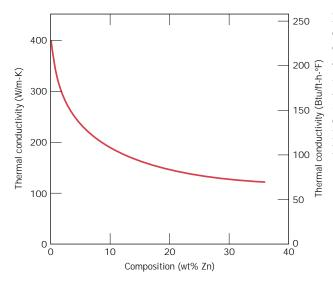
FIGURE 17.4 Thermal conductivity versus composition for copper-zinc alloys. (Adapted from Metals Handbook: Properties and Selection: Nonferrous Alloys and Pure Metals, Vol. 2, 9th edition, H. Baker, Managing Editor, American Society for Metals, 1979, p. 315.)
