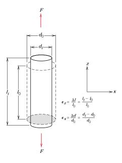
When the force F is applied, the specimen will elongate in the z direction and at the same time experience a reduction in diameter,  $\Delta d$ , of  $2.5 \times 10^{-3}$  mm in the x direction. For the strain in the x direction,
