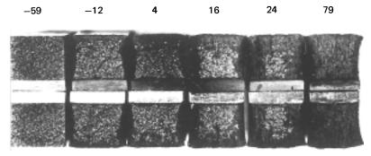
FIGURE 9.21 Photograph of fracture surfaces of A36 steel Charpy V-notch specimens tested at indicated temperatures (in °C). (From R. W. Hertzberg, *Deformation and Fracture Mechanics of Engineering Materials*, 3rd edition, Fig. 9.6, p. 329. Copyright © 1989 by John Wiley & Sons, Inc., New York. Reprinted by permission of John Wiley & Sons, Inc.)
