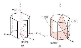
FIGURE 3.22 For the hexagonal crystal system, (a) [0001],  $[1\overline{1}00]$ , and  $[11\overline{2}0]$  directions, and (b) the (0001), (10 $\overline{1}1$ ), and ( $\overline{1}010$ ) planes.
