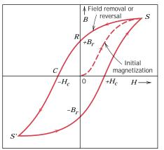
**FIGURE 18.14** Magnetic flux density versus the magnetic field strength for a ferromagnetic material that is subjected to forward and reverse saturations (points S and S'). The hysteresis loop is represented by the solid curve; the dashed curve indicates the initial magnetization. The remanence  $B_r$  and the coercive force  $H_c$  are also shown.
