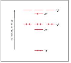
**FIGURE 2.5** Schematic representation of the filled energy states for a sodium atom.
