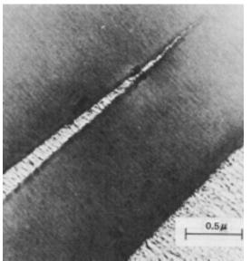
FIGURE 9.18 Photomicrograph of a craze in polyphenylene oxide. (From R. P. Kambour and R. E. Robertson, "The Mechanical Properties of Plastics," in *Polymer Science, A Materials Science Handbook,* A. D. Jenkins, Editor. Reprinted with permission of Elsevier Science Publishers.)
