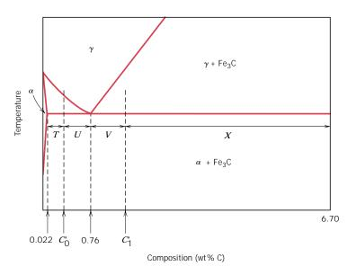
Of course, fractions of both total  $\alpha$  (eutectoid and proeutectoid) and cementite are determined using the lever rule and a tie line that extends across the entirety of the  $\alpha$  + Fe<sub>3</sub>C phase region, from 0.022 to 6.7 wt% C.
