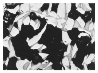
FIGURE 13.7 Photomicrograph of an aluminum oxide bonded ceramic abrasive. The light regions are the  $Al_2O_3$  abrasive grains; the gray and dark areas are the bonding phase and porosity, respectively.  $100\times$ . (From W. D. Kingery, H. K. Bowen, and D. R. Uhlmann, *Introduction to Ceramics,* 2nd edition, p. 568. Copyright © 1976 by John Wiley & Sons. Reprinted by permission of John Wiley & Sons, Inc.)
