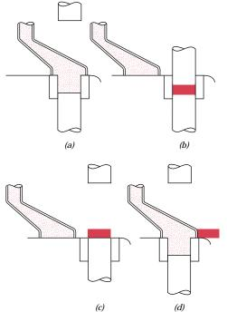
FIGURE 14.23 Schematic representation of the steps in uniaxial powder pressing. (a) The die cavity is filled with powder. (b) The powder is compacted by means of pressure applied to the top die. (c) The compacted piece is ejected by rising action of the bottom punch. (d) The fill shoe pushes away the compacted piece, and the fill step is repeated. (From W. D. Kingery, Editor, Ceramic Fabrication Processes, MIT Press. Copyright © 1958 by the Massachusetts Institute of Technology.)
