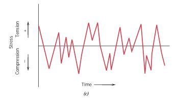
Also indicated in Figure 9.23b are several parameters used to characterize the fluctuating stress cycle. The stress amplitude alternates about a *mean stress*  $\sigma_m$ , defined as the average of the maximum and minimum stresses in the cycle, or
