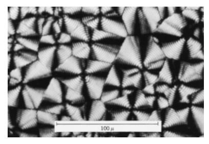
lamellae appear as thin white lines. The detailed structure of a spherulite is illustrated schematically in Figure 4.14; shown here are the individual chain-folded lamellar crystals that are separated by amorphous material. Tie-chain molecules that act as connecting links between adjacent lamellae pass through these amorphous regions.
