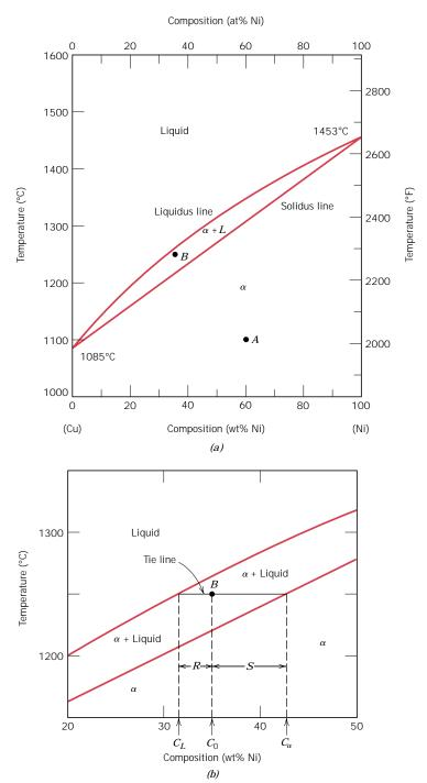
both solid  $\alpha$  and liquid phases will be in equilibrium within this temperature range. For example, upon heating an alloy of composition 50 wt% Ni–50 wt% Cu (Figure 10.2 a), melting begins at approximately 1280°C (2340°F); the amount of liquid phase continuously increases with temperature until about 1320°C (2410°F), at which the alloy is completely liquid.
