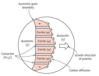
FIGURE 10.30 Schematic representation of the formation of pearlite from austenite; direction of carbon diffusion indicated by arrows.
