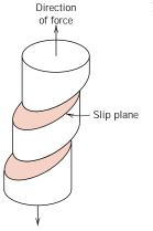
FIGURE 8.8 Macroscopic slip in a single crystal.
