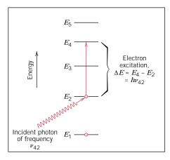
**FIGURE 19.3** For an isolated atom, a schematic illustration of photon absorption by the excitation of an electron from one energy state to another. The energy of the photon  $(hv_{42})$  must be exactly equal to the difference in energy between the two states  $(E_4 - E_2)$ .
