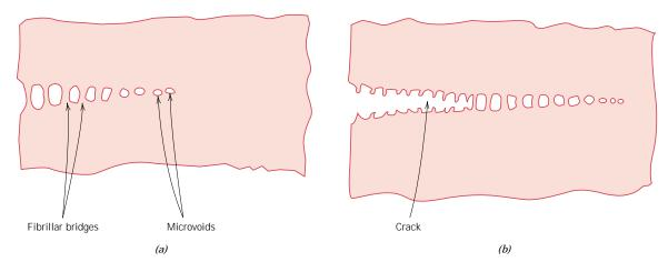
**FIGURE 9.17** Schematic drawings of (a) a craze showing microvoids and fibrillar bridges, and (b) a craze followed by a crack. (From J. W. S. Hearle, *Polymers and Their Properties*, Vol. 1, *Fundamentals of Structure and Mechanics*, Ellis Horwood, Ltd., Chichester, West Sussex, England, 1982.)
