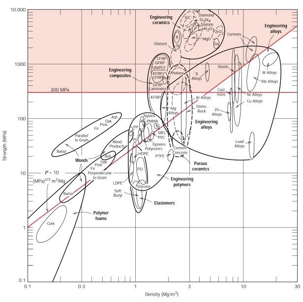
FIGURE 20.3 Strength versus density materials selection chart. Those materials lying within the shaded region are acceptable candidates for a solid cylindrical shaft which has a mass-strength performance index in excess of 10 (MPa)<sup>2/3</sup>m³/Mg, and a strength of at least 300 MPa (43,500 psi). (Adapted from M. F. Ashby, *Materials Selection in Mechanical Design*. Copyright © 1992. Reprinted by permission of Butterworth-Heinemann Ltd.)
