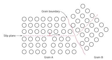
**FIGURE 8.14** The motion of a dislocation as it encounters a grain boundary, illustrating how the boundary acts as a barrier to continued slip. Slip planes are discontinuous and change directions across the boundary. (From *A Textbook of Materials Technology* by Van Vlack, © 1973. Reprinted by permission of Prentice-Hall, Inc., Upper Saddle River, NJ.)
