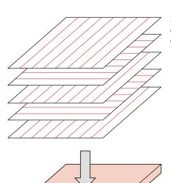
FIGURE 15.16 The stacking of successive oriented, fiber-reinforced layers for a laminar composite.
