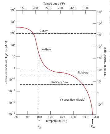
FIGURE 7.28 Logarithm of the relaxation modulus versus temperature for amorphous polystyrene, showing the five different regions of viscoelastic behavior. (From A. V. Tobolsky, *Properties and Structures of Polymers.* Copyright © 1960 by John Wiley & Sons, New York. Reprinted by permission of John Wiley & Sons, Inc.)
