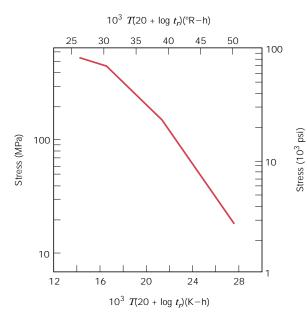
FIGURE 9.47 Logarithm stress versus the Larson–Miller parameter for an 18-8 Mo stainless steel. (From F. R. Larson and J. Miller, *Trans. ASME*, 74, 765, 1952. Reprinted by permission of ASME.)
