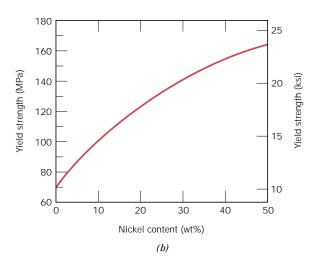
**FIGURE 8.16** Variation with nickel content of (*a*) tensile strength, (*b*) yield strength, and (*c*) ductility (%EL) for copper-nickel alloys, showing strengthening.
