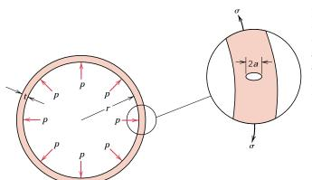
FIGURE 9.15 Schematic diagram showing the cross section of a spherical tank that is subjected to an internal pressure *p*, and that has a radial crack of length 2*a* in its wall.
