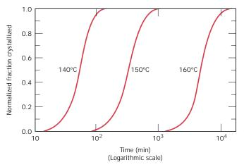
FIGURE 11.35 Plot of normalized fraction crystallized versus the logarithm of time for polypropylene at constant temperatures of 140°C, 150°C, and 160°C. (Adapted from P. Parrini and G. Corrieri, *Makromol. Chem.,* 62, 83, 1963. Reprinted by permission of Hüthig & Wepf Publishers, Zug, Switzerland.)
