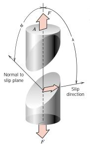
FIGURE 8.7 Geometrical relationships between the tensile axis, slip plane, and slip direction used in calculating the resolved shear stress for a single crystal.
