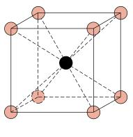
**FIGURE 3.6** A unit cell for the cesium chloride (CsCl) crystal structure.
