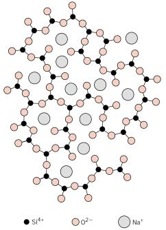
**FIGURE 3.39** Schematic representation of ion positions in a sodium–silicate glass.
