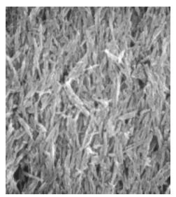
FIGURE 18.19 A scanning electron micrograph showing the microstructure of a magnetic storage disk. Needle-shaped particles of  $\gamma$ -Fe<sub>2</sub>O<sub>3</sub> are oriented and embedded within an epoxy phenolic resin. 8000×. (Photograph courtesy of P. Rayner and N. L. Head, IBM Corporation.)
