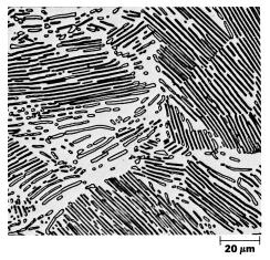
FIGURE 10.29 Photomicrograph of a eutectoid steel showing the pearlite microstructure consisting of alternating layers of  $\alpha$  ferrite (the light phase) and Fe<sub>3</sub>C (thin layers most of which appear dark). 500×. (Reproduced with permission from *Metals Handbook*, Vol. 9, 9th edition, *Metallography and Microstructures*, American Society for Metals, Materials Park, OH, 1985.)
