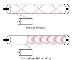
FIGURE 15.14 Schematic representations of helical, circumferential, and polar filament winding techniques. (From N. L. Hancox, Editor, *Fibre Composite Hybrid Materials*, The Macmillan Company, New York, 1981.)
