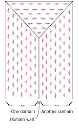
FIGURE 18.11 Schematic depiction of domains in a ferromagnetic or ferrimagnetic material; arrows represent atomic magnetic dipoles. Within each domain, all dipoles are aligned, whereas the direction of alignment varies from one domain to another.
