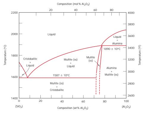
furthermore, mullite melts incongruently at 1890°C (3435°F). A single eutectic exists at 1587°C (2890°F) and 7.7 wt%  $Al_2O_3$ . In Section 13.7, refractory ceramic materials, the prime constituents for which are silica and alumina, are discussed.
