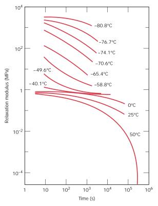
FIGURE 7.35 Logarithm of relaxation modulus versus logarithm of time for polyisobutylene between -80 and 50°C. (Adapted from E. Catsiff and A. V. Tobolsky, "Stress-Relaxation of Polyisobutylene in the Transition Region [1,2]," *J. Colloid Sci.*, 10, 377 [1955]. Reprinted by permission of Academic Press, Inc.)
