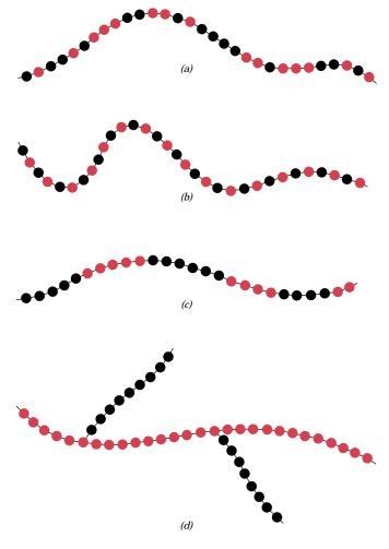
FIGURE 4.9 Schematic representations of (a) random, (b) alternating, (c) block, and (d) graft copolymers. The two different mer types are designated by black and colored circles.
