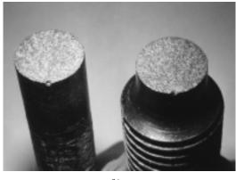
FIGURE 9.3 (a) Cup-and-cone fracture in aluminum. (b) Brittle fracture in a mild steel.
