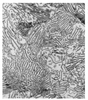
FIGURE 11.11 A photomicrograph of a pearlitic steel that has partially transformed to spheroidite. 1400×. (Courtesy of United States Steel Corporation.)
