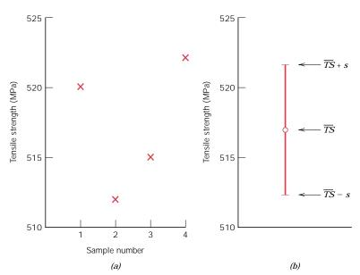
**FIGURE 7.32** (a) Tensile strength data associated with Example Problem 7.6. (b) The manner in which these data could be plotted. The data point corresponds to the average value of the tensile strength  $(\overline{TS})$ ; error bars that indicate the degree of scatter correspond to the average value plus and minus the standard deviation  $(\overline{TS} \pm s)$ .
