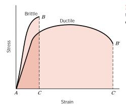
FIGURE 7.13 Schematic representations of tensile stress–strain behavior for brittle and ductile materials loaded to fracture.
