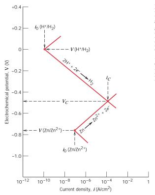
FIGURE 16.10 Electrode kinetic behavior of zinc in an acid solution; both oxidation and reduction reactions are rate limited by activation polarization. (Adapted from M. G. Fontana, *Corrosion Engineering*, 3rd edition. Copyright © 1986 by McGraw-Hill Book Company. Reproduced with permission.)
