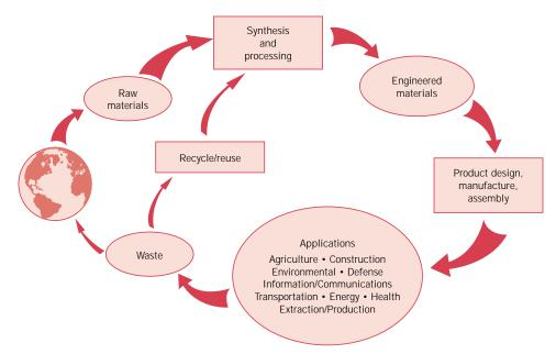
FIGURE 21.1 Schematic representation of the total materials cycle. (Adapted from M. Cohen, Advanced Materials & Processes, Vol. 147, No. 3, p. 70, 1995. Copyright © 1995 by ASM International. Reprinted by permission of ASM International, Materials Park, OH.)
