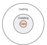
FIGURE 19.18 Schematic cross section of an optical fiber.
