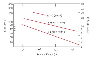
FIGURE 9.42 Stress (logarithmic scale) versus rupture lifetime (logarithmic scale) for a low carbon–nickel alloy at three temperatures. (From *Metals Handbook: Properties and Selection: Stainless Steels, Tool Materials and Special-Purpose Metals*, Vol. 3, 9th edition, D. Benjamin, Senior Editor, American Society for Metals, 1980, p. 130.)
