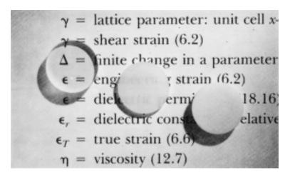
crystals that are all connected; the boundaries between these small crystals scatter a portion of the light reflected from the printed page, which makes this material optically translucent. And finally, the specimen on the right is composed not only of many small, interconnected crystals, but also of a large number of very small pores or void spaces. These pores also effectively scatter the reflected light and render this material opaque.
