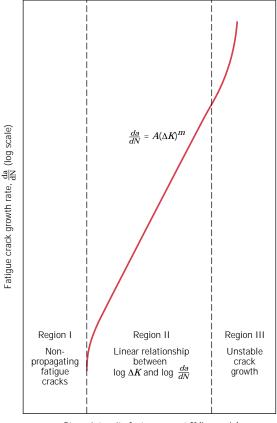
FIGURE 9.34 Schematic representation of logarithm fatigue crack propagation rate da/dN versus logarithm stress intensity factor range  $\Delta K$ . The three regions of different crack growth response (I, II, and III) are indicated. (Reprinted with permission from ASM International, Metals Park, OH 44073-9989. W. G. Clark, Jr., "How Fatigue Crack Initiation and Growth Properties Affect Material Selection and Design Criteria," *Metals Engineering Quarterly*, Vol. 14, No. 3, 1974.)
