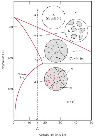
FIGURE 10.10 Schematic representations of the equilibrium microstructures for a lead-tin alloy of composition  $C_2$  as it is cooled from the liquid-phase region.
