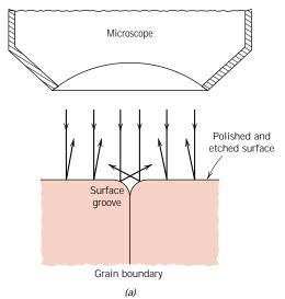
FIGURE 5.16 (a) Section of a grain boundary and its surface groove produced by etching; the light reflection characteristics in the vicinity of the groove are also shown. (b) Photomicrograph of the surface of a polished and etched polycrystalline specimen of an iron-chromium alloy in which the grain boundaries appear dark. 100×. (Photomicrograph courtesy of L. C. Smith and C. Brady, the National Bureau of Standards, Washington, DC.)
