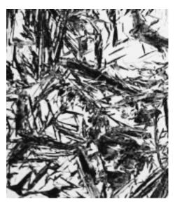
FIGURE 11.13 Photomicrograph showing the martensitic microstructure. The needle-shaped grains are the martensite phase, and the white regions are austenite that failed to transform during the rapid quench. 1220×. (Photomicrograph courtesy of United States Steel Corporation.)
