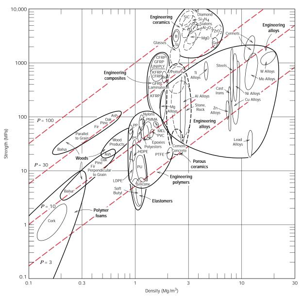
**FIGURE 20.2** Strength versus density materials selection chart. Design guidelines for performance indices of 3, 10, 30, and 100 (MPa) $^{2/3}$ m<sup>3</sup>/Mg have been constructed, all having a slope of  $\frac{3}{2}$ . (Adapted from M. F. Ashby, *Materials Selection in Mechanical Design.* Copyright © 1992. Reprinted by permission of Butterworth-Heinemann Ltd.)
