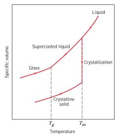
FIGURE 14.15 Contrast of specific volume-versus-temperature behavior of crystalline and noncrystalline materials. Crystalline materials solidify at the melting temperature  $T_m$ . Characteristic of the noncrystalline state is the glass transition temperature  $T_g$ .
