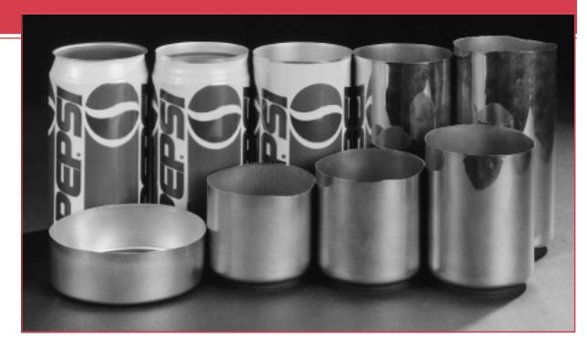
his photograph shows the aluminum beverage can in various stages of production. The can is formed from a single sheet of an aluminum alloy. Production operations include drawing, dome forming, trimming, cleaning, decorating, and neck and flange forming. (PEPSI is a registered trademark of PepsiCo, Inc. Used by permission.)
