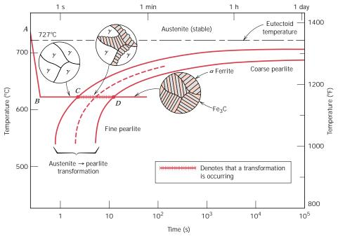
**FIGURE 11.5** Isothermal transformation diagram for a eutectoid iron–carbon alloy, with superimposed isothermal heat treatment curve (*ABCD*). Microstructures before, during, and after the austenite-to-pearlite transformation are shown. (Adapted from H. Boyer, Editor, *Atlas of Isothermal Transformation and Cooling Transformation Diagrams, American Society for Metals, 1977, p. 28.)*
