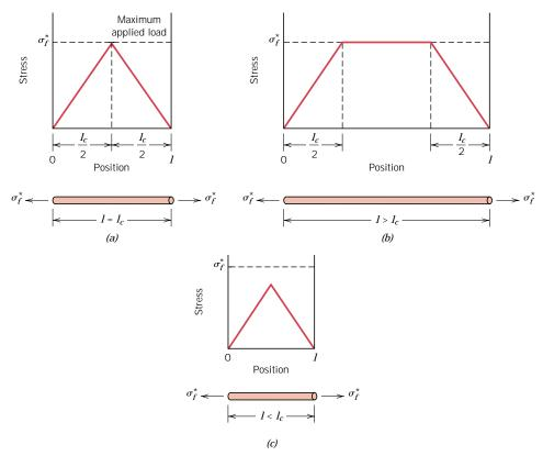
**FIGURE 15.7** Stress-position profiles when fiber length I(a) is equal to the critical length  $I_c$ , (b) is greater than the critical length, and (c) is less than the critical length for a fiber-reinforced composite that is subjected to a tensile stress equal to the fiber tensile strength  $\sigma_{\epsilon}^*$ .
