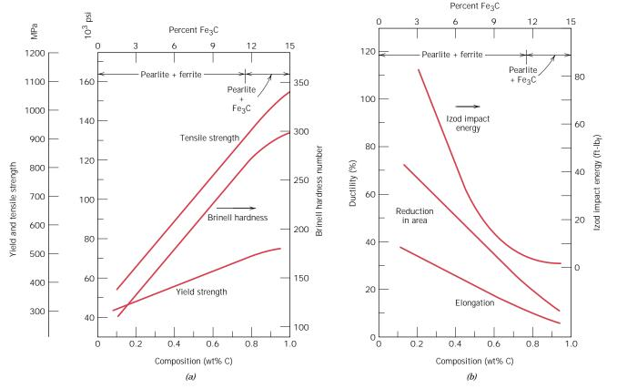
**FIGURE 11.21** (a) Yield strength, tensile strength, and Brinell hardness versus carbon concentration for plain carbon steels having microstructures consisting of fine pearlite. (b) Ductility (%EL and %RA) and Izod impact energy versus carbon concentration for plain carbon steels having microstructures consisting of fine pearlite. (Data taken from *Metals Handbook: Heat Treating,* Vol. 4, 9th edition, V. Masseria, Managing Editor, American Society for Metals, 1981, p. 9.)
