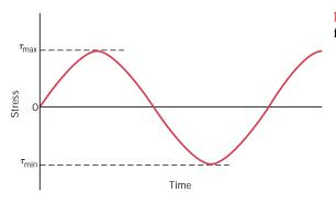
FIGURE 20.8 Stress versus time for a reversed cycle in shear.
