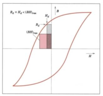
FIGURE 18.17 Schematic magnetization curve that displays hysteresis. Within the second quadrant are drawn two B-H energy product rectangles; the area of that rectangle labeled  $(BH)_{\rm max}$  is the largest possible, which is greater than the area defined by  $B_d$ - $H_d$ .
