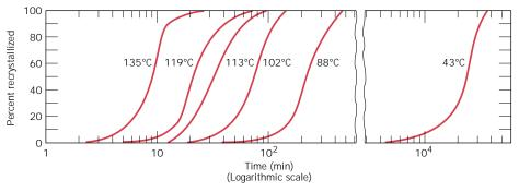
FIGURE 11.2 Percent recrystallization as a function of time and at constant temperature for pure copper. (Reprinted with permission from *Metallurgical Transactions,* Vol. 188, 1950, a publication of The Metallurgical Society of AIME, Warrendale, Pennsylvania. Adapted from B. F. Decker and D. Harker, "Recrystallization in Rolled Copper," *Trans. AIME,* 188, 1950, p. 888.)
