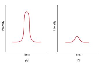
encoding scheme for optical communications. (a) A high-power pulse of photons corresponds to a "one" in the binary format. (b) A low-power photon pulse represents a "zero."
