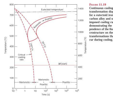
**FIGURE 11.19** Continuous cooling transformation diagram for a eutectoid ironcarbon alloy and superimposed cooling curves, demonstrating the dependence of the final microstructure on the transformations that oc-
