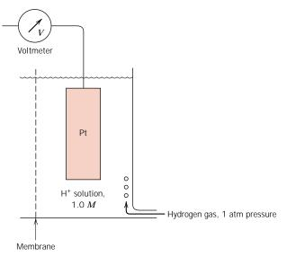
**FIGURE 16.4** The standard hydrogen reference half-cell.
