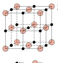
FIGURE 3.5 A unit cell for the rock salt, or sodium chloride (NaCl), crystal structure.
