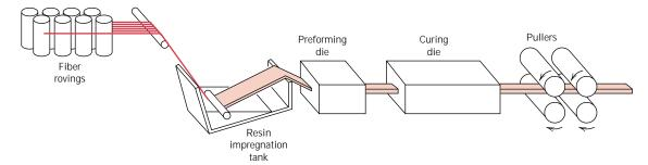
FIGURE 15.12 Schematic diagram showing the pultrusion process.
