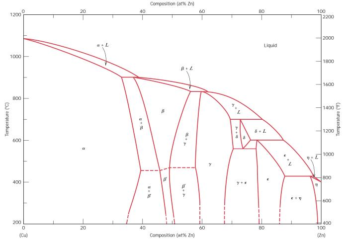
FIGURE 10.17 The copper–zinc phase diagram. (Adapted from *Binary Alloy Phase Diagrams*, 2nd edition, Vol. 2, T. B. Massalski, Editor-in-Chief, 1990. Reprinted by permission of ASM International, Materials Park, OH.)
