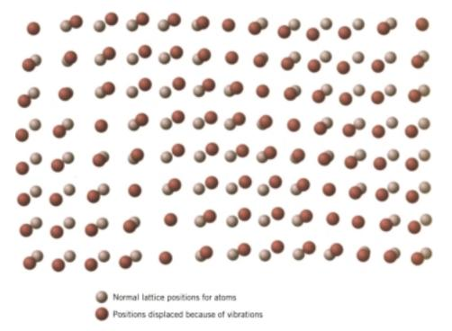
**FIGURE 17.1** Schematic representation of the generation of lattice waves in a crystal by means of atomic vibrations. (Adapted from "The Thermal Properties of Materials" by J. Ziman. Copyright © 1967 by Scientific American, Inc. All rights reserved.)
