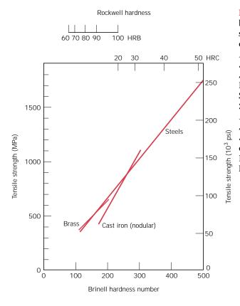
FIGURE 7.31 Relationships between hardness and tensile strength for steel, brass, and cast iron. (Data taken from Metals Handbook: Properties and Selection: Irons and Steels, Vol. 1, 9th edition, B. Bardes, Editor, American Society for Metals, 1978, pp. 36 and 461; and Metals Handbook: Properties and Selection: Nonferrous Alloys and Pure Metals, Vol. 2, 9th edition, H. Baker, Managing Editor, American Society for Metals, 1979, p. 327.)
