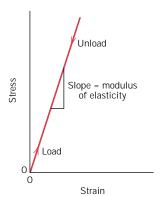
FIGURE 7.5 Schematic stress-strain diagram showing linear elastic deformation for loading and unloading cycles.
