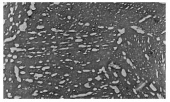
FIGURE 11.25 Electron micrograph of tempered martensite. Tempering was carried out at 594°C (1100°F). The small particles are the cementite phase; the matrix phase is  $\alpha$  ferrite. 9300×. (Copyright 1971 by United States Steel Corporation.)
