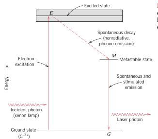
FIGURE 19.12 Schematic energy diagram for the ruby laser, showing electron excitation and decay paths.
