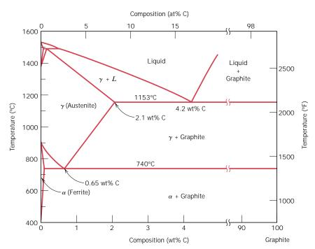
as graphite, and both microstructure and mechanical behavior depend on composition and heat treatment. The most common cast iron types are gray, nodular, white, and malleable.
