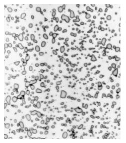
FIGURE 11.10 Photomicrograph of a steel having a spheroidite microstructure. The small particles are cementite; the continuous phase is  $\alpha$  ferrite.  $1000 \times$ . (Copyright 1971 by United States Steel Corporation.)
