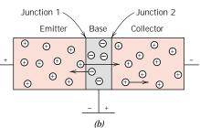
its attendant circuitry. A very thin *n*-type *base* region is sandwiched in between *p*-type *emitter* and *collector* regions. The circuit that includes the emitter-base junction (junction 1) is forward biased, whereas a reverse bias voltage is applied across the base-collector junction (junction 2).
