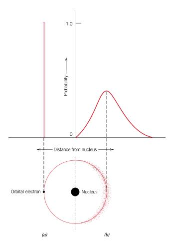
FIGURE 2.3 Comparison of the (a) Bohr and (b) wave-mechanical atom models in terms of electron distribution. (Adapted from Z. D. Jastrzebski, *The Nature and Properties of Engineering Materials,* 3rd edition, p. 4. Copyright © 1987 by John Wiley & Sons, New York. Reprinted by permission of John Wiley & Sons, Inc.)
