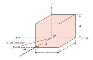
This problem is solved by reversing the procedure of the preceding example. For this  $[1\bar{1}0]$  direction, the projections along the x, y, z axes are a, -a, and 0a, respectively. This direction is defined by a vector passing from the origin to point P, which is located by first moving along the x axis a units, and from this position, parallel to the y axis -a units, as indicated in the figure. There is no z component to the vector, since the z projection is zero.
