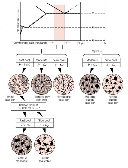
phase, white iron is extremely hard but also very brittle, to the point of being virtually unmachinable. Its use is limited to applications that necessitate a very hard and wear-resistant surface, and without a high degree of ductility—for example, as rollers in rolling mills. Generally, white iron is used as an intermediary in the production of yet another cast iron, **malleable iron**.
