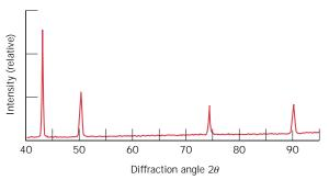
**FIGURE 3.41** Diffraction pattern for polycrystalline copper.
