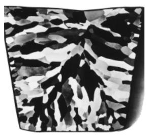
FIGURE 5.14 High-purity polycrystalline lead ingot in which the individual grains may be discerned. 0.7×. (Reproduced with permission from *Metals Handbook*, Vol. 9, 9th edition, *Metallography and Microstructures*, American Society for Metals, Metals Park, OH, 1985.)
