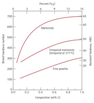
FIGURE 11.24 Hardness as a function of carbon concentration for plain carbon martensitic, tempered at 371°C (700°F)], and pearlitic steels. (Adapted from Edgar C. Bain, Functions of the Alloying Elements in Steel, American Society for Metals, 1939, p. 36; and R. A. Grange, C. R. Hribal, and L. F. Porter: Metall. Trans. A, Vol. 8A, p. 1776.)
