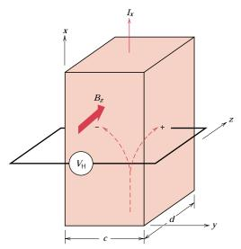
FIGURE 12.18 Schematic demonstration of the Hall effect. Positive and/or negative charge carriers that are part of the  $I_x$  current are deflected by the magnetic field  $B_z$  and give rise to the Hall voltage,  $V_{\rm H}$ .
