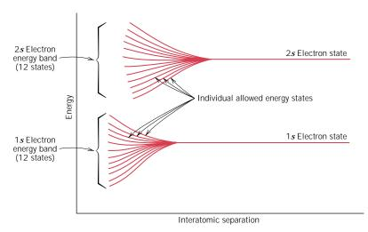
adjacent states is exceedingly small. At the equilibrium spacing, band formation may not occur for the electron subshells nearest the nucleus, as illustrated in Figure 12.3b. Furthermore, gaps may exist between adjacent bands, as also indicated in the figure; normally, energies lying within these band gaps are not available for electron occupancy. The conventional way of representing electron band structures in solids is shown in Figure 12.3a.
