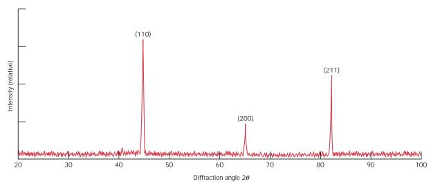
**FIGURE 3.37** Diffraction pattern for polycrystalline  $\alpha$ -iron.
