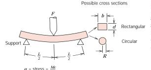
FIGURE 7.18 A three-point loading scheme for measuring the stress-strain behavior and flexural strength of brittle ceramics, including expressions for computing stress for rectangular and circular cross sections.
