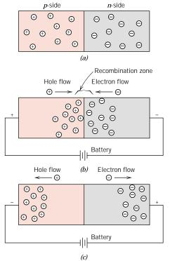
**FIGURE 12.19** For a p-n rectifying junction, representations of electron and hole distributions for (a) no electrical potential, (b) forward bias, and (c) reverse bias.
