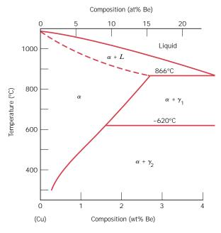
FIGURE 11.40 The copper-rich side of the copper-beryllium phase diagram. (Adapted from Binary Alloy Phase Diagrams, 2nd edition, Vol. 2, T. B. Massalski, Editor-in-Chief, 1990. Reprinted by permission of ASM International, Materials Park, OH.)
