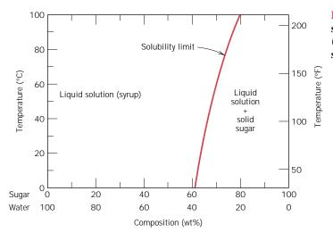
FIGURE 10.1 The solubility of sugar  $(C_{12}H_{22}O_{11})$  in a sugar-water syrup.
