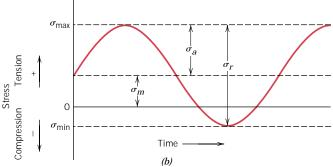
FIGURE 9.23 Variation of stress with time that accounts for fatigue failures. (a) Reversed stress cycle, in which the stress alternates from a maximum tensile stress (+) to a maximum compressive stress (-) of equal magnitude. (b) Repeated stress cycle, in which maximum and minimum stresses are asymmetrical relative to the zero stress level; mean stress  $\sigma_m$ , range of stress  $\sigma_r$ , and stress amplitude  $\sigma_a$  are indicated. (c) Random stress cycle.
