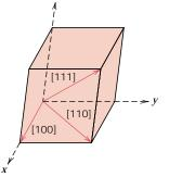
**FIGURE 3.20** The [100], [110], and [111] directions within a unit cell.
