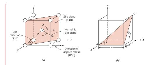
**(b)** The yield strength  $\sigma_y$  may be computed from Equation 8.3;  $\phi$  and  $\lambda$  will be the same as for part a, and
