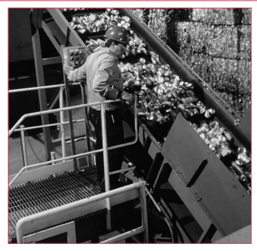
Used aluminum beverage cans that are to be recycled. These cans will be crushed and pressed into bales (shown in the background) and then shredded into small pieces. Ferrous and nonferrous metal contaminants are next eliminated, and the decorative coating is removed in a delacquering operation. A thermomechanical process then separates can bodies (alloy 3004) from the lids (alloy 5182). The final recycling stages include melting, refining, casting, and rolling. (Photograph courtesy Alcoa.)
