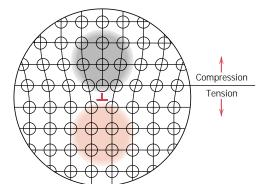
FIGURE 8.4 Regions of compression (dark) and tension (colored) located around an edge dislocation. (Adapted from W. G. Moffatt, G. W. Pearsall, and J. Wulff, *The Structure and Properties of Materials*, Vol. I, *Structure*, p. 85. Copyright © 1964 by John Wiley & Sons, New York. Reprinted by permission of John Wiley & Sons, Inc.)
