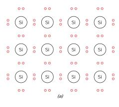
**FIGURE 12.10** Electron bonding model of electrical conduction in intrinsic silicon: (a) before excitation; (b) and (c) after excitation (the subsequent free-electron and hole motions in response to an external electric field).
