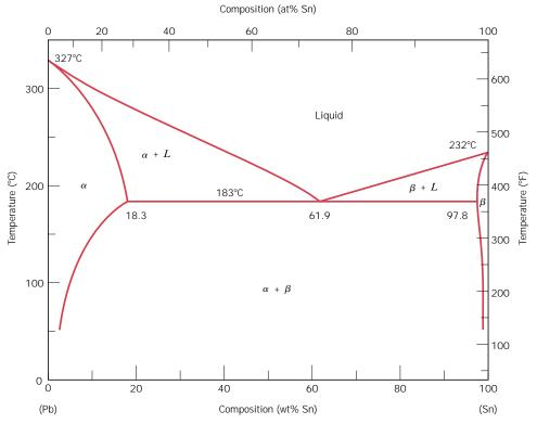
**FIGURE 10.7** The lead-tin phase diagram. (Adapted from *Binary Alloy Phase Diagrams*, 2nd edition, Vol. 3, T. B. Massalski, Editor-in-Chief, 1990. Reprinted by permission of ASM International, Materials Park, OH.)
