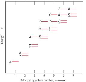
FIGURE 2.4 Schematic representation of the relative energies of the electrons for the various shells and subshells. (From K. M. Ralls, T. H. Courtney, and J. Wulff, *Introduction to Materials Science and Engineering,* p. 22. Copyright © 1976 by John Wiley & Sons, New York. Reprinted by permission of John Wiley & Sons, Inc.)
