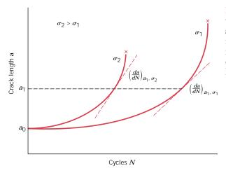
**FIGURE 9.33** Crack length versus the number of cycles at stress levels  $\sigma_1$  and  $\sigma_2$  for fatigue studies. Crack growth rate da/dN is indicated at crack length  $a_1$  for both stress levels.
