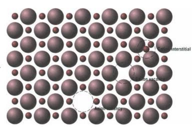
Schematic diagram showing Frenkel and Schottky defects in ionic solids. (From W. G. Moffatt, G. W. Pearsall, and J. Wulff, The Structure and Properties of Materials, Vol. 1, Structure, p. 78. Copyright © 1964 by John Wiley & Sons, New York. Reprinted by permission of John Wiley & Sons, Inc.)
