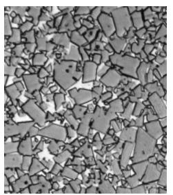
FIGURE 15.4 Photomicrograph of a WC-Co cemented carbide. Light areas are the cobalt matrix; dark regions, the particles of tungsten carbide. 100×. (Courtesy of Carboloy Systems Department, General Electric Company.)
