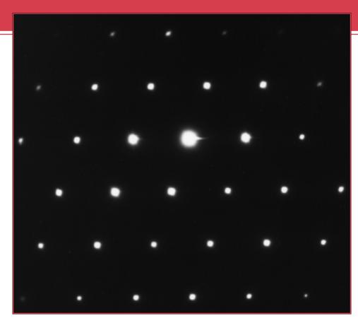
High velocity electron beams that are produced when electrons are accelerated across large voltages become wavelike in character. Their wavelengths are shorter than interatomic spacings, and thus these beams may be diffracted by atomic planes in crystalline materials, in the same manner as x-rays experience diffraction.
