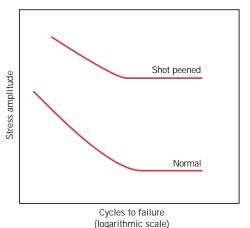
**FIGURE 9.38** Schematic S-N fatigue curves for normal and shot-peened steel.
