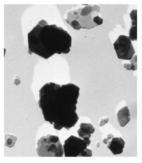
FIGURE 3.15 Electron micrograph of kaolinite crystals. They are in the form of hexagonal plates, some of which are stacked on top of one another. 15,000×. (Photograph courtesy of Georgia Kaolin Co., Inc.)
