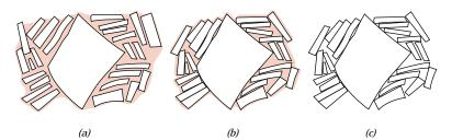
FIGURE 14.21 Several stages in the removal of water from between clay particles during the drying process. (a) Wet body. (b) Partially dry body. (c) Completely dry body. (From W. D. Kingery, *Introduction to Ceramics*. Copyright © 1960 by John Wiley & Sons, New York. Reprinted by permission of John Wiley & Sons, Inc.)
