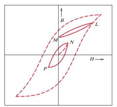
FIGURE 18.15 A hysteresis curve at less than saturation (curve NP) within the saturation loop for a ferromagnetic material. The B-H behavior for field reversal at other than saturation is indicated by curve LM.
