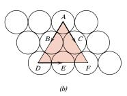
FIGURE 8.6 (a) A  $\{111\}\langle 110 \rangle$  slip system shown within an FCC unit cell. (b) The (111) plane from (a) and three  $\langle 110 \rangle$  slip directions (as indicated by arrows) within that plane comprise possible slip systems.
