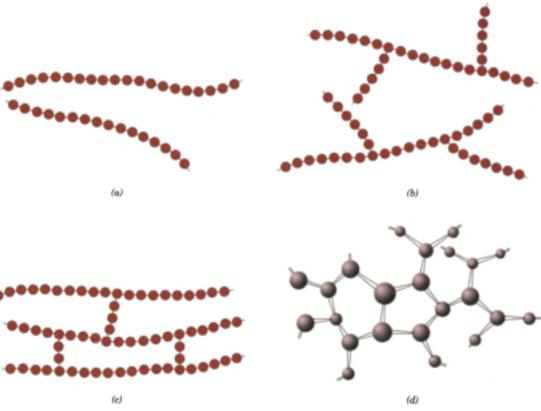
**FIGURE 4.7** Schematic representations of (a) linear, (b) branched, (c) crosslinked, and (d) network (three-dimensional) molecular structures. Circles designate individual mer units.
