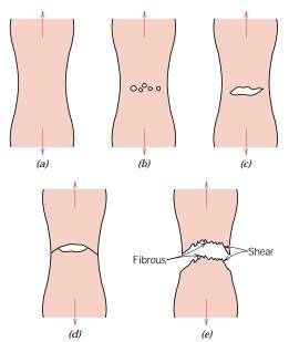
FIGURE 9.2 Stages in the cup-and-cone fracture. (a) Initial necking. (b) Small cavity formation. (c) Coalescence of cavities to form a crack. (d) Crack propagation. (e) Final shear fracture at a 45° angle relative to the tensile direction. (From K. M. Ralls, T. H. Courtney, and J. Wulff, Introduction to Materials Science and Engineering, p. 468. Copyright © 1976 by John Wiley & Sons, New York. Reprinted by permission of John Wiley & Sons, Inc.)
