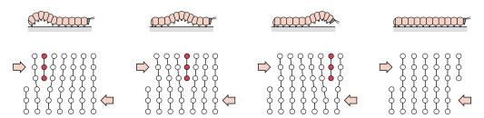
FIGURE 8.3 Representation of the analogy between caterpillar and dislocation motion.
