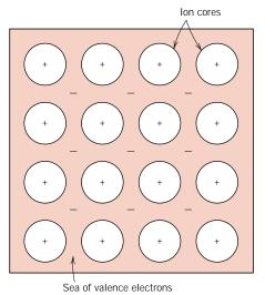
**FIGURE 2.11** Schematic illustration of metallic bonding.
