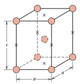
**FIGURE 11.12** The body-centered tetragonal unit cell for martensitic steel showing iron atoms (circles) and sites that may be occupied by carbon atoms (crosses). For this tetragonal unit cell, c > a.
