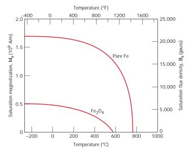
FIGURE 18.10 Plot of saturation magnetization as a function of temperature for iron and Fe<sub>3</sub>O<sub>4</sub>. [Adapted from J. Smit and H. P. J. Wijn, *Ferrites*. Copyright © 1959 by N. V. Philips Gloeilampenfabrieken, Eindhoven (Holland). Reprinted by permission.]
