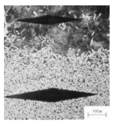
FIGURE 9.39 Photomicrograph showing both core (bottom) and carburized outer case (top) regions of a case-hardened steel. The case is harder as attested by the smaller microhardness indentation. 100×. (From R. W. Hertzberg, *Deformation and Fracture Mechanics of Engineering Materials,* 3rd edition. Copyright © 1989 by John Wiley & Sons, New York. Reprinted by permission of John Wiley & Sons, Inc.)
