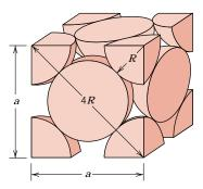
the atoms touch one another across a face-diagonal the length of which is 4R. Since the unit cell is a cube, its volume is  $a^3$ , where a is the cell edge length. From the right triangle on the face,
