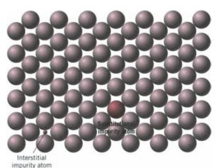
FIGURE 5.5 Two-dimensional schematic representations of substitutional and interstitial impurity atoms. (Adapted from W. G. Moffatt, G. W. Pearsall, and J. Wulff, *The Structure and Properties of Materials*, Vol. I, *Structure*, p. 77. Copyright © 1964 by John Wiley & Sons, New York. Reprinted by permission of John Wiley & Sons, Inc.)
