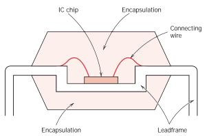
FIGURE 20.25 Schematic diagram showing an encapsulated IC leadframe package. (Adapted from Electronic Materials Handbook, Vol. 1, Packaging, C. A. Dostal, editor, ASM International, 1989, p. 241.)
