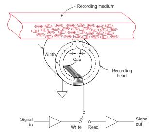
FIGURE 18.18 Schematic representation showing how information is stored and retrieved using a magnetic storage medium. (From J. U. Lemke, *MRS Bulletin*, Vol. XV, No. 3, p. 31, 1990. Reprinted with permission.)
