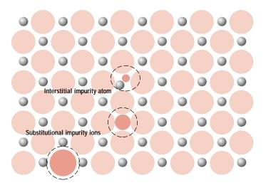
FIGURE 5.6 Schematic representations of interstitial, anion-substitutional, and cation-substitutional impurity atoms in an ionic compound. (Adapted from W. G. Moffatt, G. W. Pearsall, and J. Wulff, *The Structure and Properties of Materials*, Vol. 1, *Structure*, p. 78. Copyright © 1964 by John Wiley & Sons, New York. Reprinted by permission of John Wiley & Sons, Inc.)
