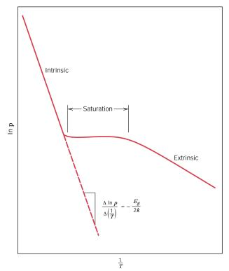
FIGURE 12.17 Schematic plot of the natural logarithm of hole concentration as a function of the reciprocal of absolute temperature for a *p*-type semiconductor that exhibits extrinsic, saturation, and intrinsic behavior.
