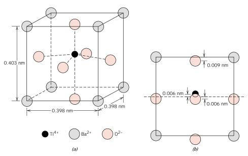
**FIGURE 12.33** A barium titanate (BaTiO<sub>3</sub>) unit cell (*a*) in an isometric projection, and (*b*) looking at one face, which shows the displacements of  $Ti^{4+}$  and  $O^{2-}$  ions from the center of the face.
