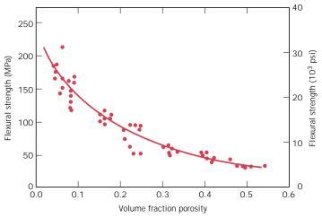
**FIGURE 7.21** The influence of porosity on the flexural strength for aluminum oxide at room temperature. (From R. L. Coble and W. D. Kingery, "Effect of Porosity on Physical Properties of Sintered Alumina," *J. Am. Ceram. Soc.*, **39**, 11, Nov. 1956, p. 382. Reprinted by permission of the American Ceramic Society.)
