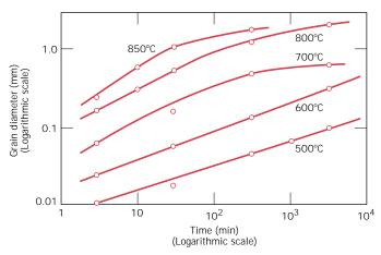
**FIGURE 8.25** The logarithm of grain diameter versus the logarithm of time for grain growth in brass at several temperatures. (From J. E. Burke, "Some Factors Affecting the Rate of Grain Growth in Metals." Reprinted with permission from *Metallurgical Transactions*, Vol. 180, 1949, a publication of The Metallurgical Society of AIME, Warrendale, Pennsylvania.)
