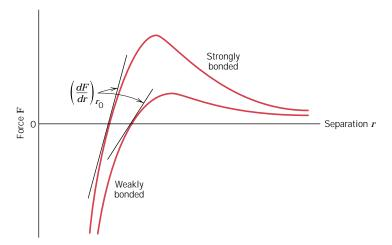
Differences in modulus values between metals, ceramics, and polymers are a direct consequence of the different types of atomic bonding that exist for the three materials types. Furthermore, with increasing temperature, the modulus of elasticity diminishes for all but some of the rubber materials; this effect is shown for several metals in Figure 7.8.
