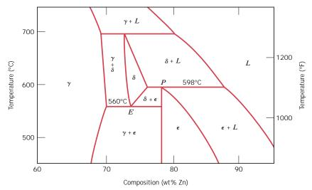
**FIGURE 10.19** A region of the copper–zinc phase diagram that has been enlarged to show eutectoid and peritectic invariant points, labeled E (560°C, 74 wt% Zn) and P (598°C, 78.6 wt% Zn), respectively. (Adapted from *Binary Alloy Phase Diagrams*, 2nd edition, Vol. 2, T. B. Massalski, Editor-in-Chief, 1990. Reprinted by permission of ASM International, Materials Park, OH.)
