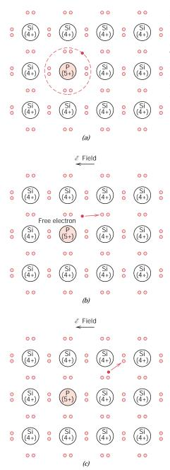
FIGURE 12.11 Extrinsic *n*-type semiconduction model (electron bonding). (a) An impurity atom such as phosphorus, having five valence electrons, may substitute for a silicon atom. This results in an extra bonding electron, which is bound to the impurity atom and orbits it. (b) Excitation to form a free electron. (c) The motion of this free electron in response to an electric field.
