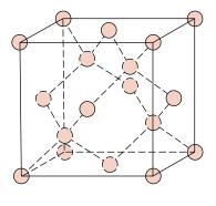
FIGURE 3.16 A unit cell for the diamond cubic crystal structure.
