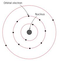
FIGURE 2.1 Schematic representation of the Bohr atom.
