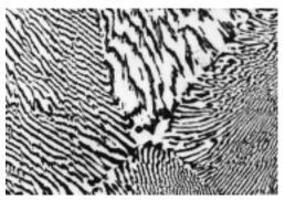
FIGURE 10.12 Photomicrograph showing the microstructure of a lead–tin alloy of eutectic composition. This microstructure consists of alternating layers of a lead-rich  $\alpha$ -phase solid solution (dark layers), and a tin-rich  $\beta$ -phase solid solution (light layers). 375×. (Reproduced with permission from *Metals Handbook*, Vol. 9, 9th edition, *Metallography and Microstructures*, American Society for Metals, Materials Park, OH, 1985.)
