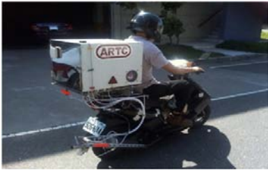
Figure 1. OBS-584 Installed onto One of Test Motorcycles
