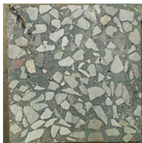
Figure 2. Distribution of the Coarse Aggregate in Concrete.
