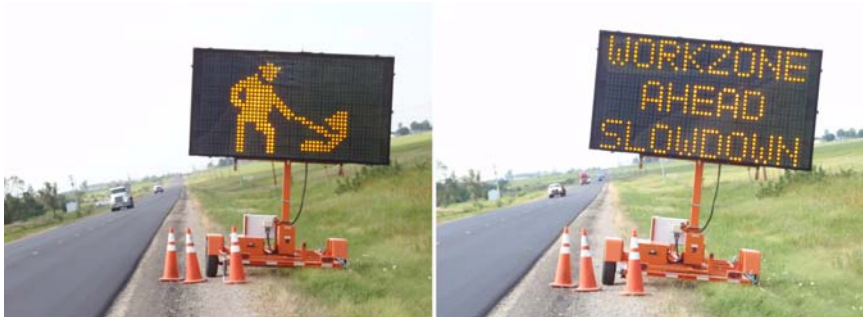
Figure 2. Work Zone PCMS One
