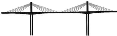
Figure 2.The FEA model of bridge
