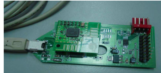
Fig. 9 Prototype hub device connected to USB port
