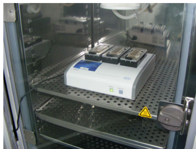
Fig. 2 Image of the cell analyzer of the xCELLigence system, located in a cell culture incubator. Three 16 well E-Plates are placed in the three appropriate holders
