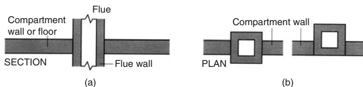
Figure 6.110 Flues penetrating compartment walls or floors. (a) Flue passing through compartment wall or floor. (b) Flue built into compartment wall
