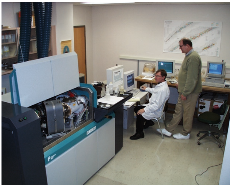
Fig. 4.25 James Burton and Doug Price with the Element ICP-MS in the Laboratory for Archaeological Chemistry at the University of Wisconsin–Madison
