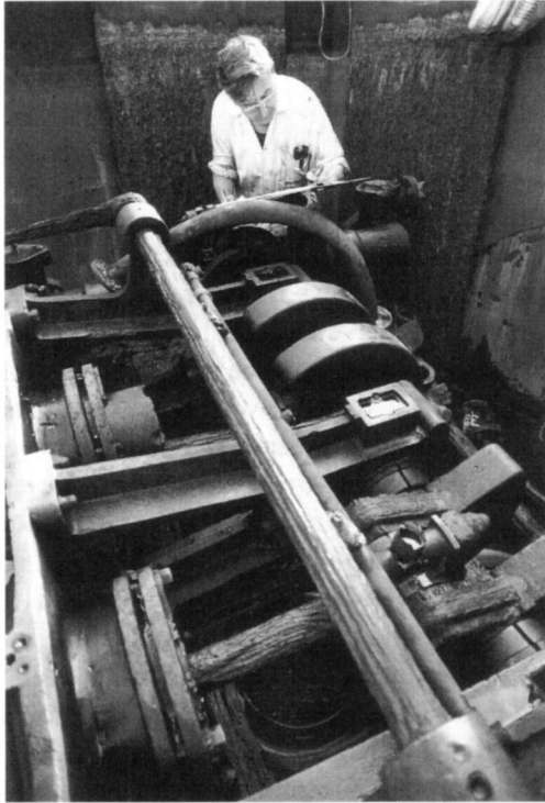
Figure 67. Noel Miller recording the upper surfaces of the engine. The oil cup is in the right foreground (Pat Baker).
