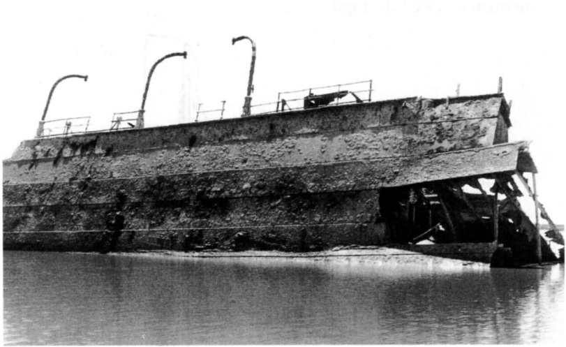
Figure 3. Hull plating amidships on SS Colac . The “in and out” system is clearly visible (M. McCarthy). See also Figures 19 and 39.
