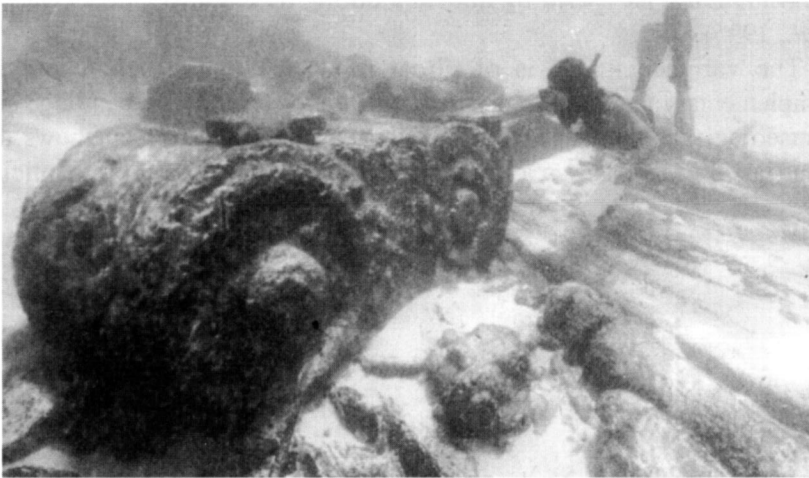
Figure 10. The SS Georgette compound engine, showing the differing diameters of the cylinders. The author is examining the high-pressure cylinder (Scott Sledge).
