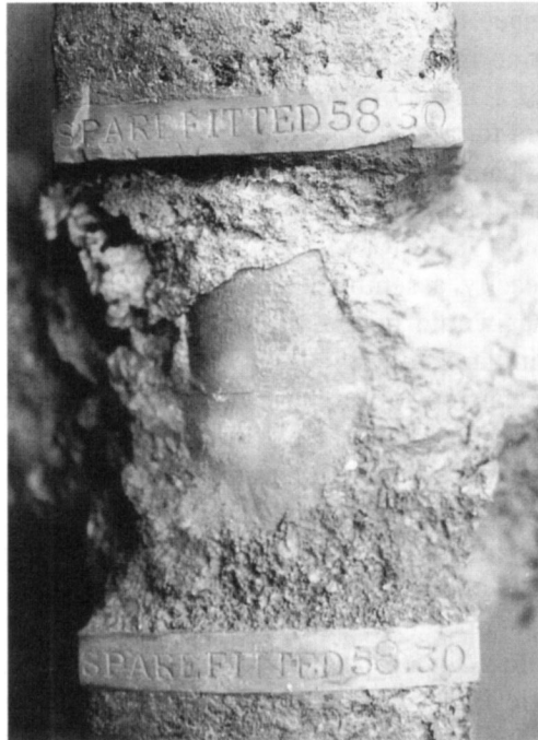
Figure 69. An end of the spare connecting rod showing the markings, SPARE FITTED 58.30. The connecting rod is shown in situ beneath the thrust block and flanges in Figure 45 (Jon Carpenter).
