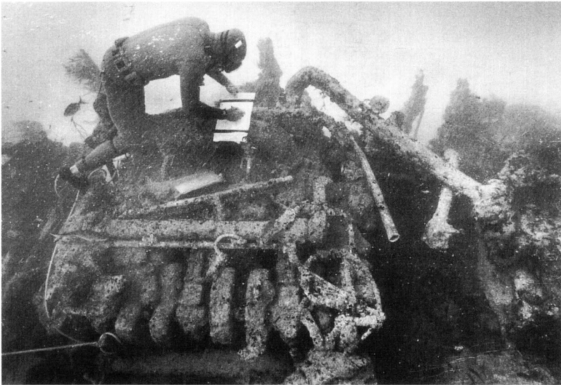
Figure 30. Geoff Kimpton recording the Xantho engine using manual methods. The crankshaft, oil cups, and piping are visible (M. McCarthy).
