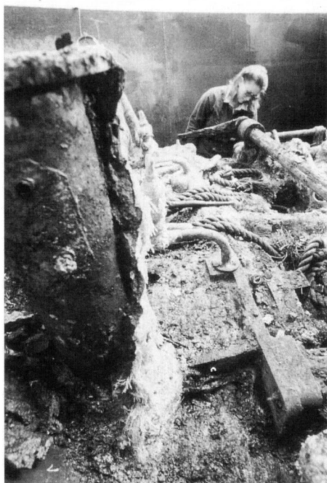
Figure 63. Deconcretion in progress. In the foreground is the upper part of the engine exhausts, showing the thickness of the concretion layer. In front of conservator Michelle Berry is the wrought-iron weigh shaft (Jon Carpenter).
