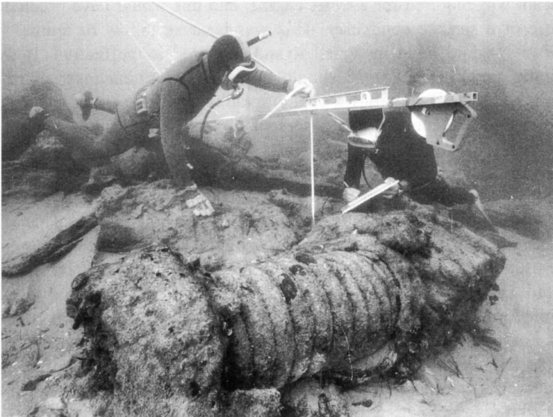
Figure 48. The object believed to be a condenser on the Xantho wreck (Pat Baker).
