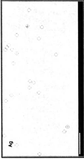
Figure 4. X-ray map for As, Sb, Cu, and Ag on curse tablet P44. Regions with concentrations of elements above background level are circled.
