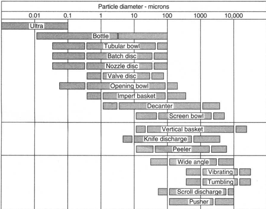
Figure 10.16. Classification of centrifuges by particle size (after Sutherland, 1970)
