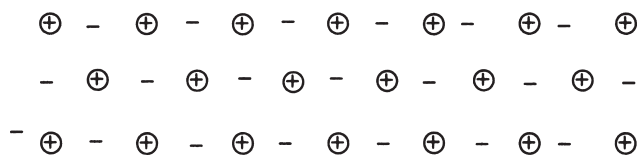
Figure 11.4 Metallic bonding. The atoms of the metal form a regular lattice, the exact nature of which depends on the ionic radius of the metal involved. Each atom donates an electron to the “cloud” which is free to move throughout the structure and holds the ions together.
