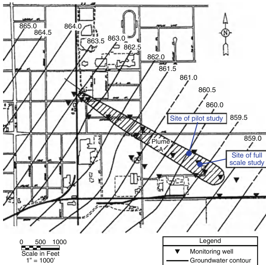
Figure 9.11. Schoolcraft Plume A: site of pilot- and demonstration-scale tests of bioaugmentation with P. stutzeri KC.
