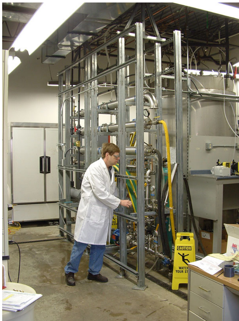
Figure 3.10. Stainless steel cell filtration system for concentrating Dhc cultures. The concentration system consists of tubular ceramic membranes contained within stainless steel shells. The individual membrane units are connected in series and water from the culture passes through the membranes and is captured in the shell and disposed. Concentrated culture is transferred back to the fermentor ( background ) and the culture recirculated through the system until the desired concentration factor is achieved.
