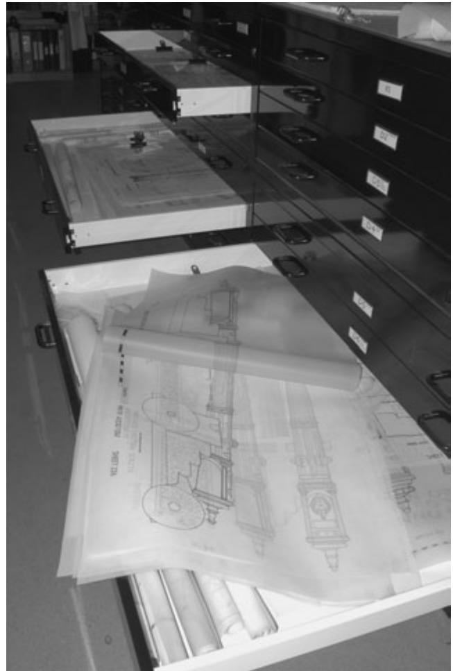
Figure 19.1 A plan chest is an ideal way to store plans and drawings. They can be laid flat and inspected with ease. Variants in which drawings are suspended from racks are also available. (Photo: Mary Rose Trust)
