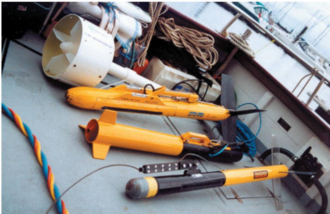
Plate 13.12 Top to bottom: a Geometrics G-881 caesium magnetometer (white tow-fish), an EdgeTech 272-TD side-scan, a GeoAcoustics side-scan and an Imagenex 885 side-scan sonar. (Photo: Rory Quinn)
