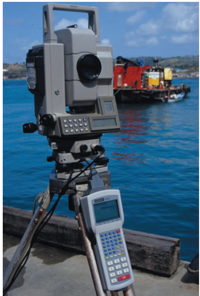
Plate 11.1 A 'total station' ready for use. (Photo: Kester Keighley)
