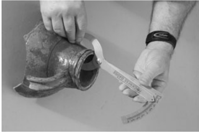
Figure 18.8 Thickness-gauge callipers can be useful in determining a pot's section. (Photo: Edward Martin)
