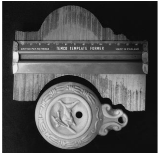
Figure 18.10 Profile gauges can provide a quick way of checking the shape of an object but they can easily damage delicate surfaces and should only be used on robust items. Their use is not generally recommended in recording small finds (for which better techniques are available), but they can be useful for recording features such as the mouldings on guns. (Photo: Colin Martin)
