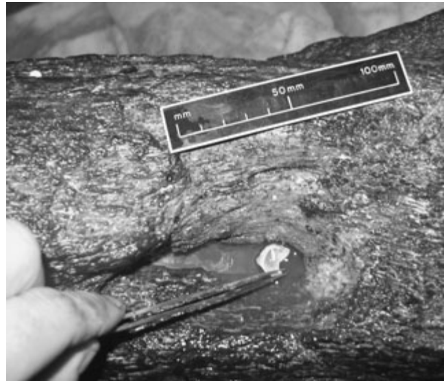
Figure 16.1 Teredo navalis (shipworm): a large shell, evidence for historical shipworm infestation of the timber, is removed from the upper stem timber of the Mary Rose as part of the recording and cleaning process, prior to active conservation. (Photo: Doug McElvogue)
