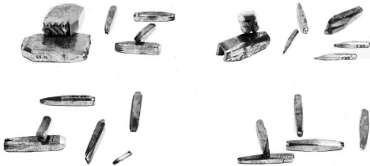
(8) Top : Punches from the Plantin-Moretus Museum collection, the work of some of the greatest sixteenth-century punch-cutters: above left Van den Keere; above right Le Bé; below left Granjon; below right Garamond. Each of these craftsmen had his own way of finishing off his punches, seen in the length of the shanks, in square-cut, pointed, or rounded ends, so that the sets are quite easily distinguishable. Note among Granjon's punches one with the shank partly cut through ( above left ) and a small punch ( below right ). The latter is an accent which could be fastened to the larger punch and struck together in a matrix.
