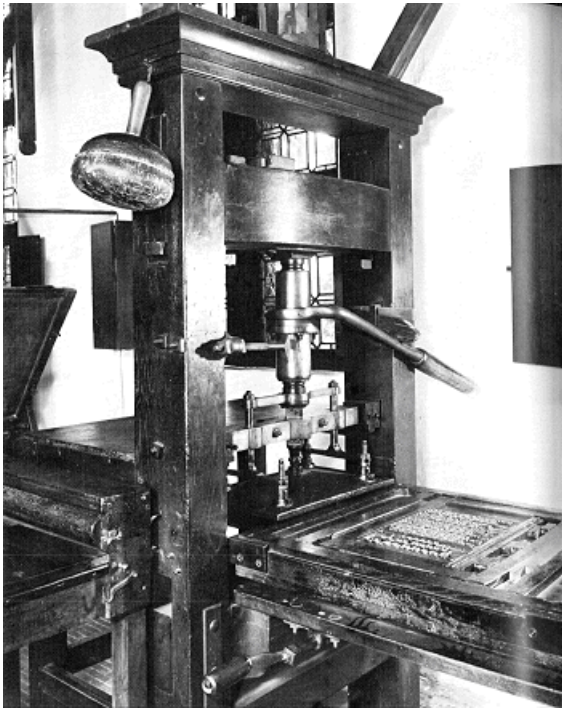
(20) Detailed view of one of the later presses. The more sophisticated system of screws fastening the platen to the yoke is clearly visible.
