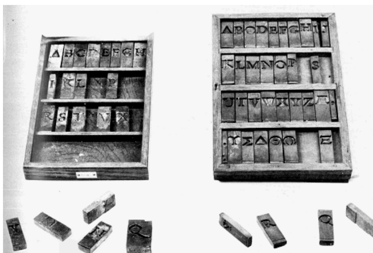
(11) Opposite, bottom : Matrices. Left in lead-(MA 9); right in copper (MA 78) of the same body size ('Grosses Capitales Extraordinaires' by Garamond, later completed by the addition of Greek capitals by Van den Keere). The lead matrices, which lack the Greek capitals, are more roughly finished: they may have been a cheap set, meant for sale at Frankfurt.
