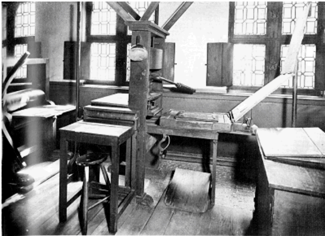
21) Top : Side view of one of the later presses showing the various appurtenances. On the left, leaning against the press, is the stand on which the ink was spread. An ink-ball hangs from the top of the frame.
