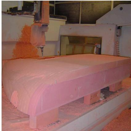
Figure 13: Plug Machining
