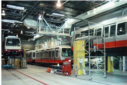
South of it is a cleaning cubicle that is enclosed on three sides and prevents positioning of a third vehicle on that track under any circumstances. Because of the limited space south of the current positions and the trapping potential discussed above which would be worsened if three individual vehicles were serviced on any one track, there is little opportunity to increase the number of vehicle service positions inside the current shop.
