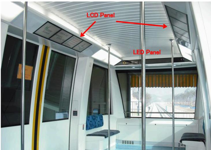
IHI has achieved the effect of a brighter, more spacious and comfortable vehicle cabin in part by adopting large windows and doors. In certain situations, this can reduce the impact of the LCD wide screen panels by interfering with visibility. Table: 'Factors Affecting LCD Visibility' lists some of the factors that can result in reduced LCD visibility in the vehicle cabin.
