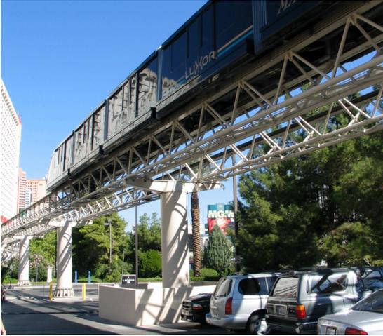
Image 1: Doppelmayr Cable Liner Shuttle; © DCC
