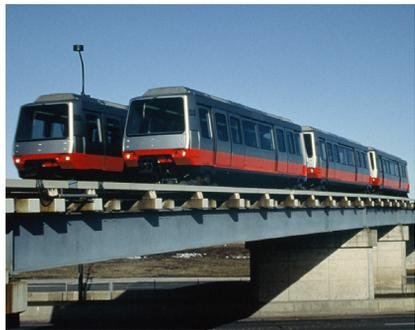
French Matra (now Siemens) VAL technology, which opened in Lille, France in 1983. The O'Hare ATS opened in 1993 and uses a wider VAL 256 vehicle. Those wider vehicles were also originally delivered as part of VAL systems built in Jacksonville and Taipei. The current ATS fleet is 15 vehicles which operate on 2.71 miles of double guideway with passenger stations at three domestic terminals, the international terminal and remote parking facilities.
