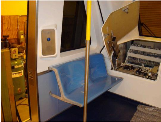
Figure 20: End Interior with Cover Open
