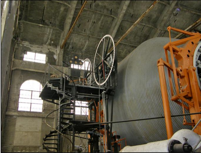
**Figure 6 -- Nordberg double expansion steam hoist**
