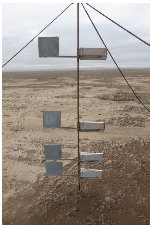
Simple but effective rotating BSNE (Big Spring Number Eight) horizontal flux sand traps. Heights of individual traps often relate to those of accompanying anemometers, which record wind velocities. Photograph by David Thomas.
