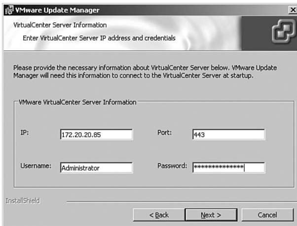
Figure 8.22 Installing Update Manager: Entering vCenter Server information
