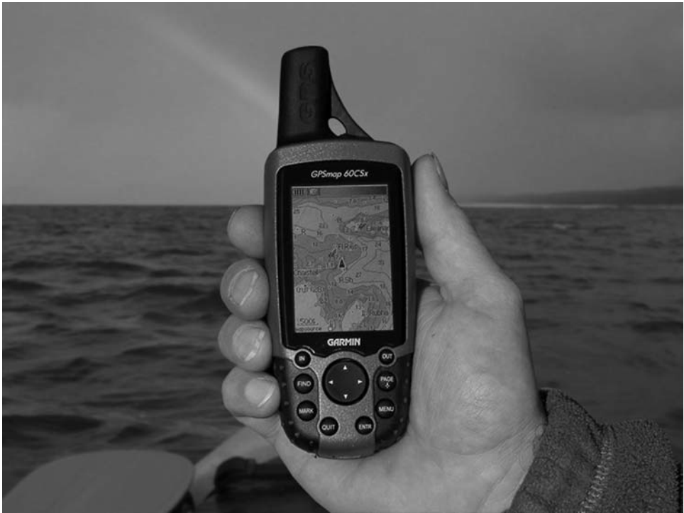
Figure 4-1. Garmin handheld recreational GPS receiver with compass and barometric altimeter. Such receivers can be DGPS if WAAS-enabled.
