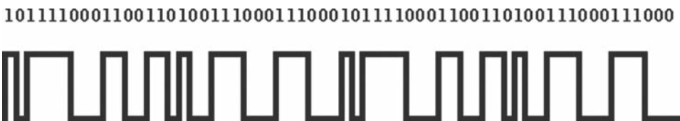
Figure 2-11. A short pseudo random noise (PRN) code sample.
