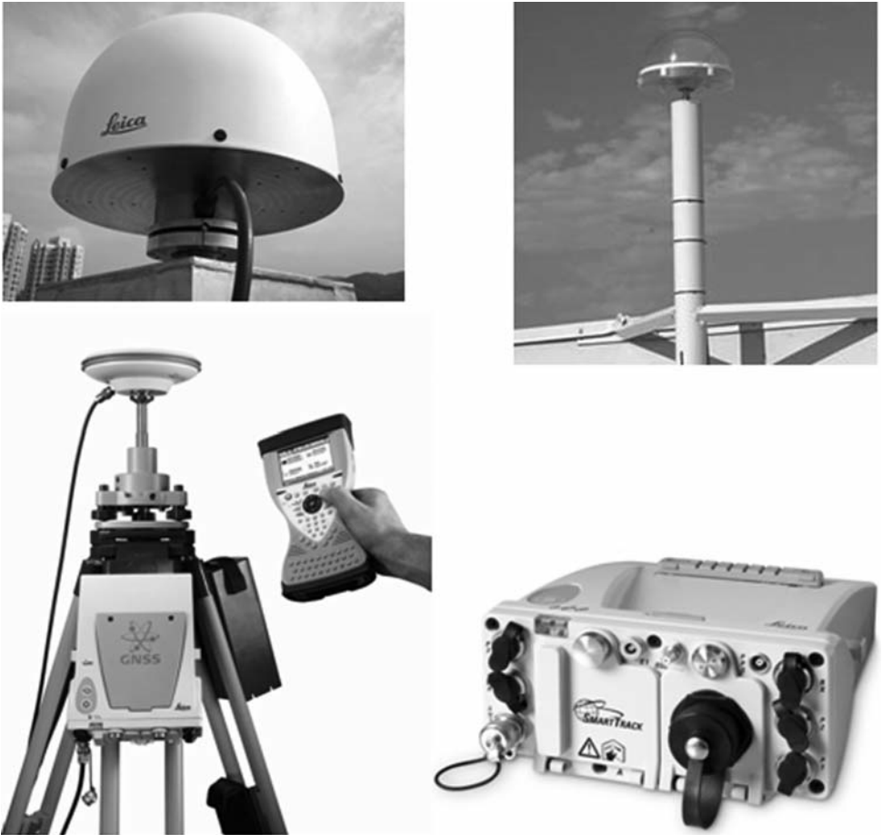
Figure 5-4. Equipment for centimeter-level (or better) positioning. Clockwise from top left: geodetic antenna with radome antenna cover; geodetic antenna at a base station; geodetic receiver; antenna on tripod with receiver and a detached handheld controller.
